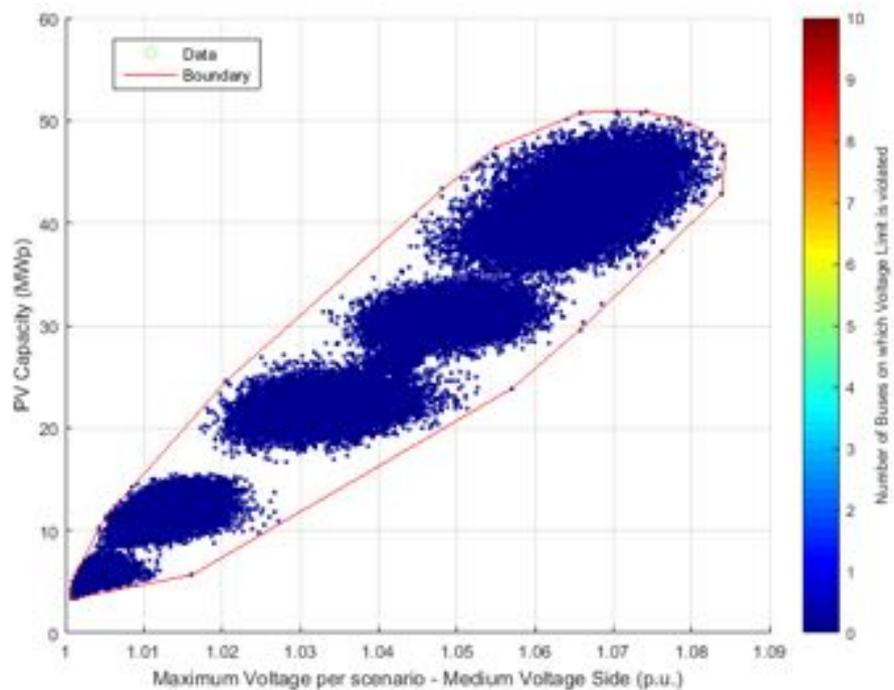
**Figure 316.** PV Capacity against Voltage – Medium voltage side - Power Factor equal to 0.95.
