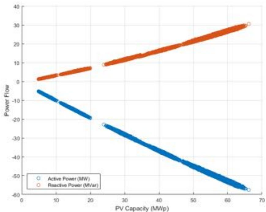
**Figure 267.** Power flow at PCC (connection of the reference substation with HV network) vs PV Capacity - Power Factor equal to 0.95.
