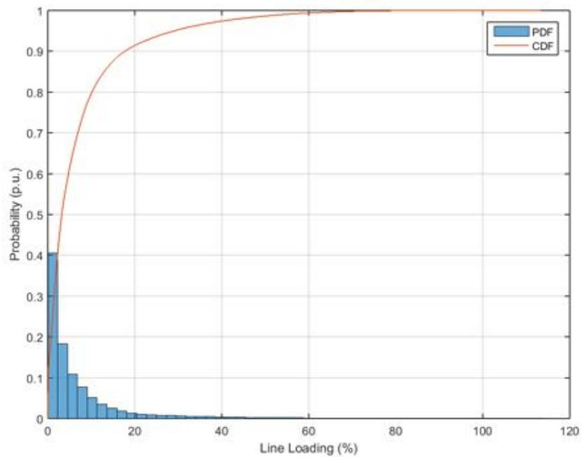
**Figure 186.** Probability distribution and cumulative probability distribution – Line Loading – Power Factor  $\cos\phi(P)$ .
