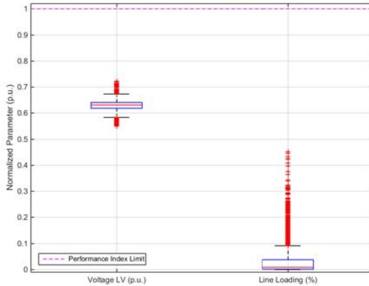
**Figure 34.** Performance Index parameters normalized to their limit – Power Factor equal to 0.95.
