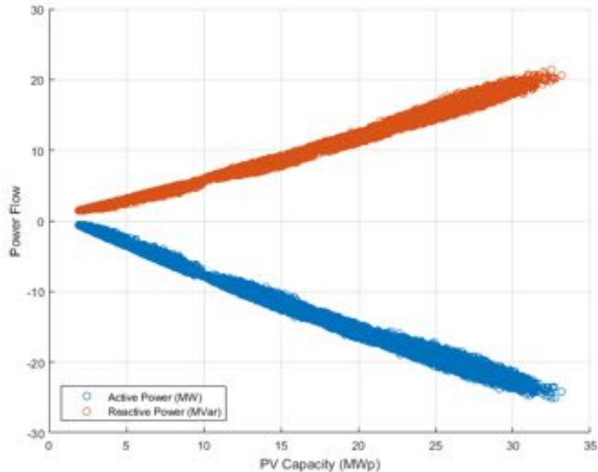
**Figure 153.** Power flow at PCC (connection of the reference substation with HV network) against PV capacity - Unity Power Factor (negative sign denotes reverse power flow).
