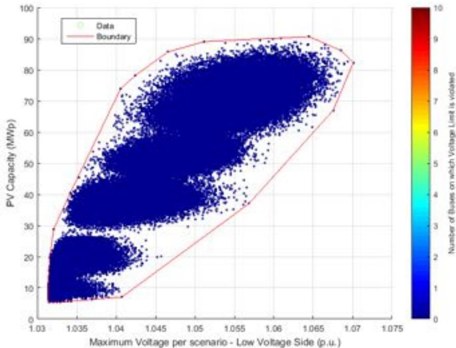
**Figure 58.** PV Capacity against Voltage – Low voltage side - Power Factor  $\cos\phi(P)$ .
