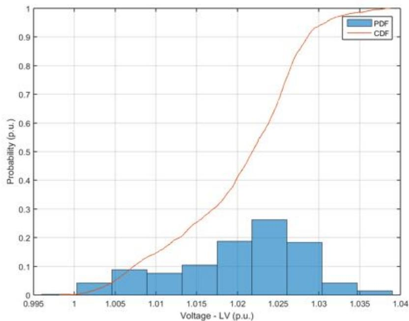
**Figure 92.** Probability distribution and cumulative probability distribution – Voltage at low voltage side – Power Factor  $\cos\phi(P)$ .
