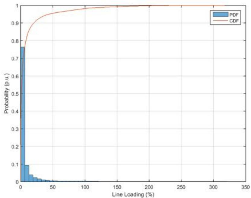
**Figure 128.** Probability distribution and cumulative probability distribution – Line Loading – Power Factor equal to 0.95.
