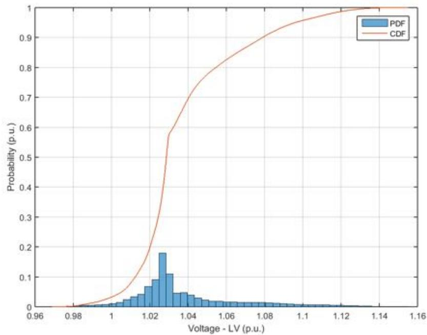
**Figure 290.** Probability distribution and cumulative probability distribution – Voltage at low voltage side – Power Factor  $\cos\phi(P)$ .
