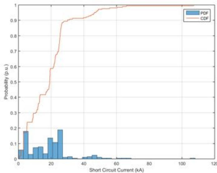
**Figure 37.** Probability distribution and cumulative probability distribution – Short Circuit Current – Power Factor equal to 0.95.
