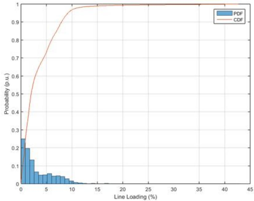
**Figure 195.** Probability distribution and cumulative probability distribution – Line Loading – Power Factor equal to 0.95.
