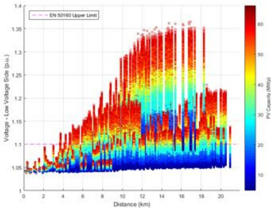
**Figure 266.** Voltage at low voltage side against Distance from transmission substation - Power Factor equal to 0.95.
