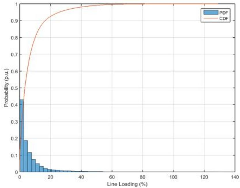
**Figure 176.** Probability distribution and cumulative probability distribution – Line Loading – Unity power factor.
