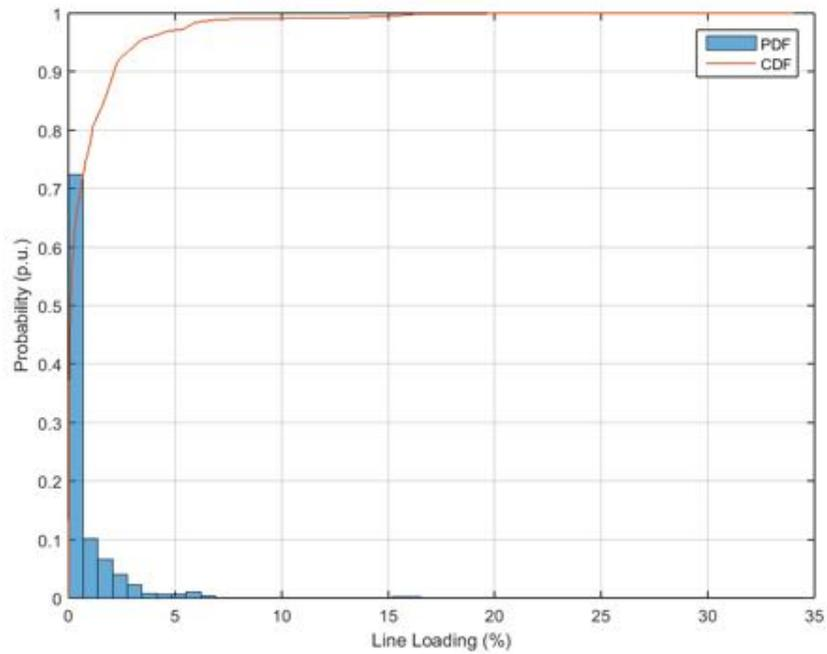
**Figure 248.** Probability distribution and cumulative probability distribution – Line Loading – Power Factor equal to 0.95.
