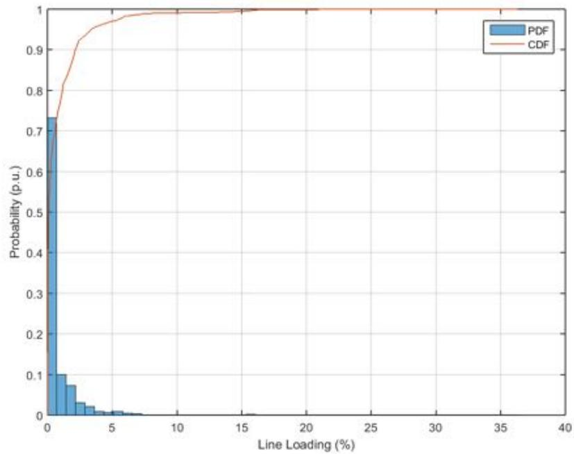
**Figure 252.** Probability distribution and cumulative probability distribution – Line Loading – Power Factor  $\cos\phi(P)$ .
