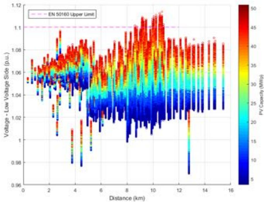
**Figure 319.** Voltage at low voltage side against Distance from transmission substation - Power Factor equal to 0.95.
