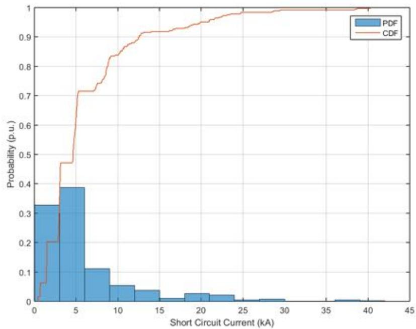
**Figure 298.** Probability distribution and cumulative probability distribution – Short Circuit Current – Unity Power Factor.
