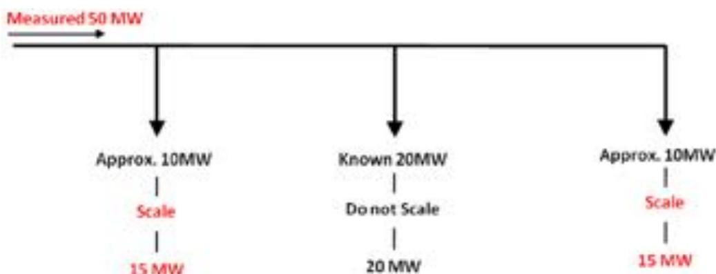
**Figure 3.** Feeder load scaling [5].
