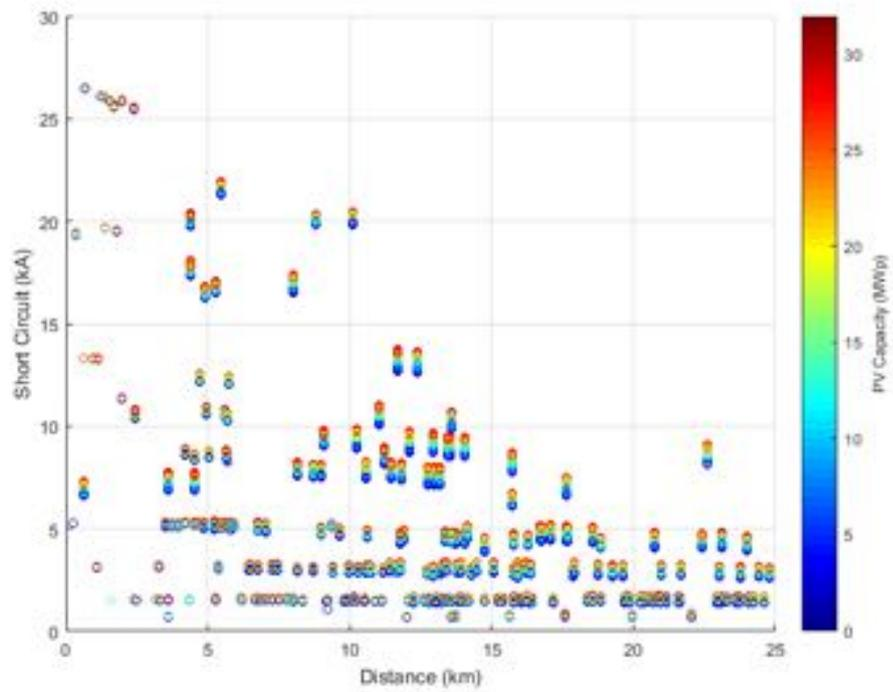
**Figure 154.** Short circuit current against distance - Unity Power Factor.
