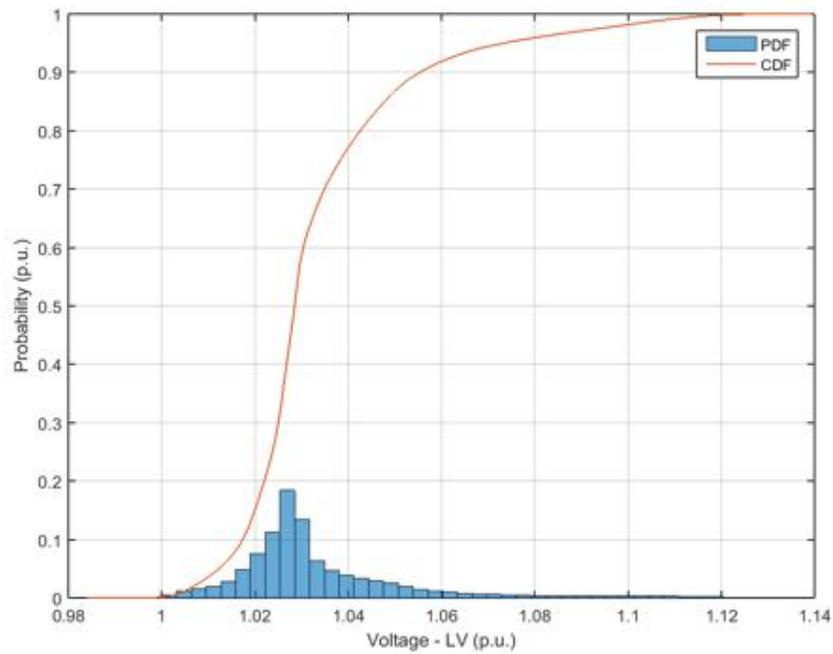
**Figure 73.** Probability distribution and cumulative probability distribution – Voltage at low voltage side – Power Factor equal to 0.95.
