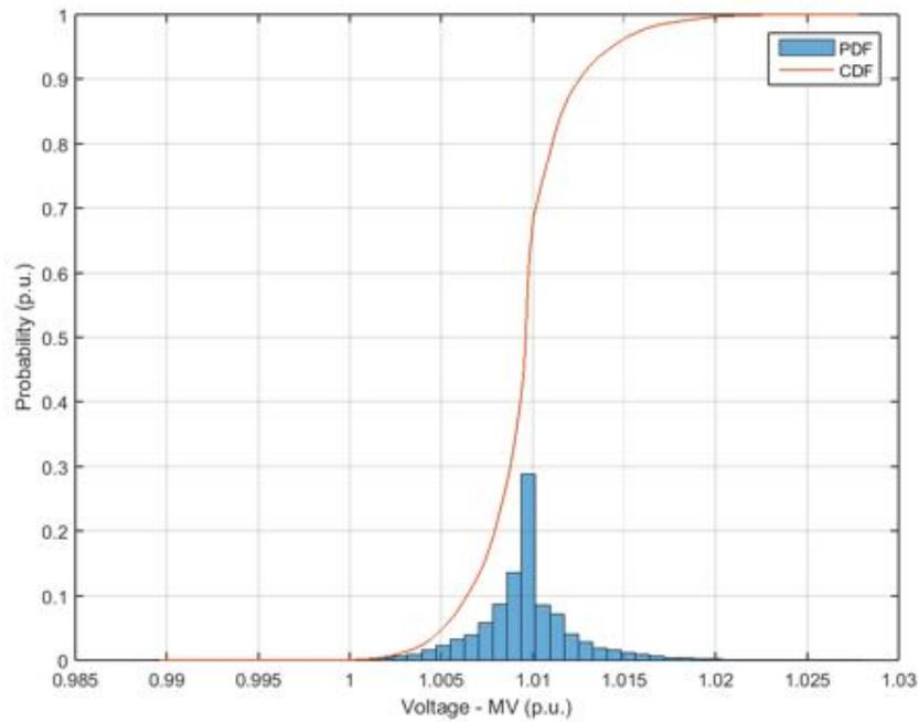
**Figure 185.** Probability distribution and cumulative probability distribution – Voltage at medium voltage side – Power Factor  $\cos\phi(P)$ .
