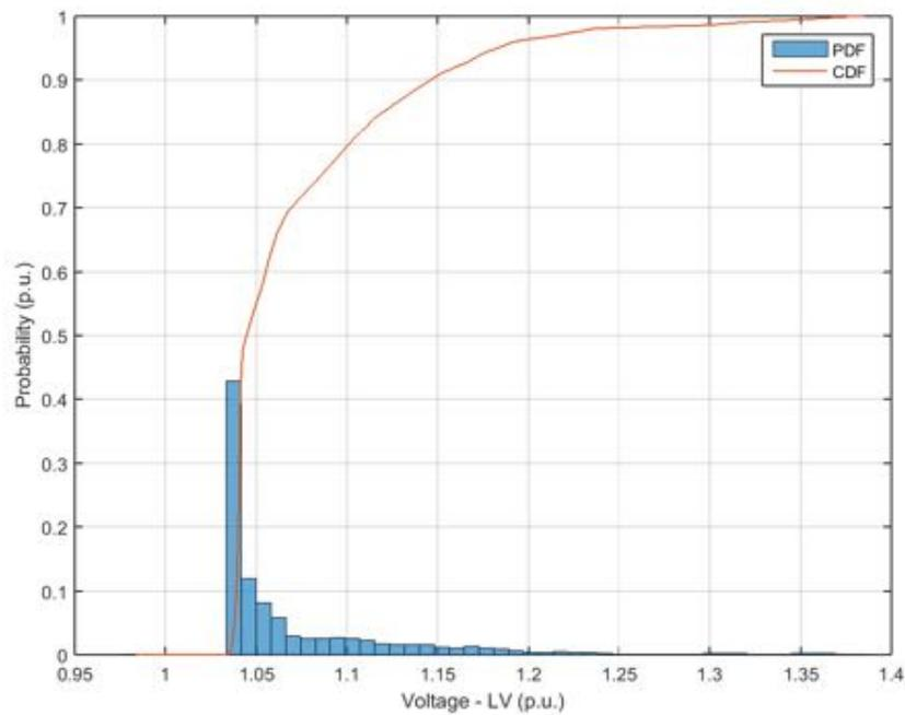
**Figure 237.** Probability distribution and cumulative probability distribution – Voltage at low voltage side – Power Factor  $\cos\phi(P)$ .
