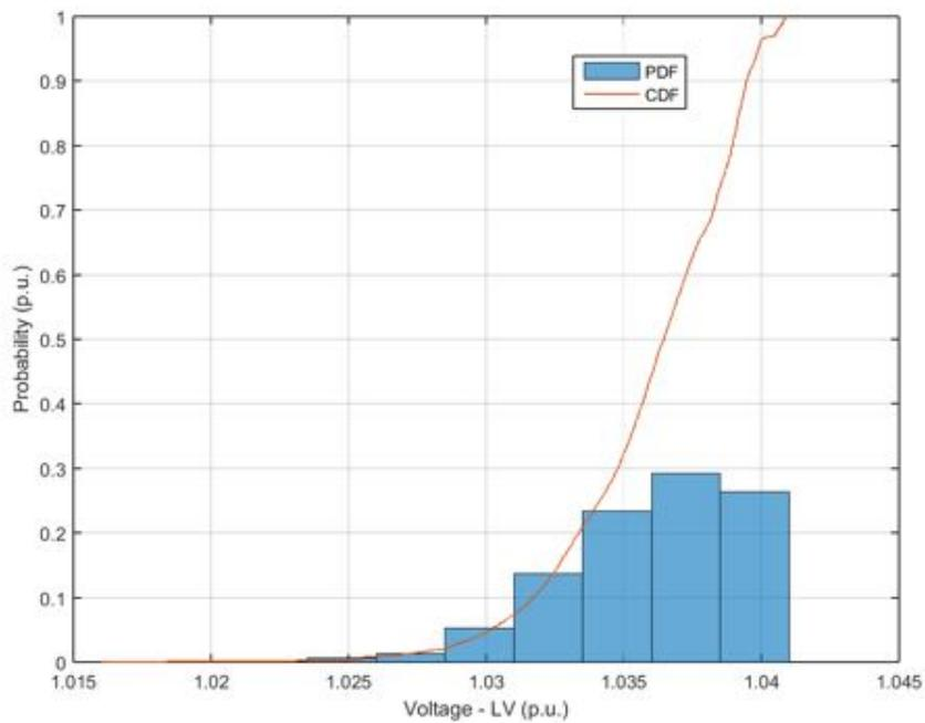
**Figure 194.** Probability distribution and cumulative probability distribution – Voltage at low voltage side – Power Factor equal to 0.95.
