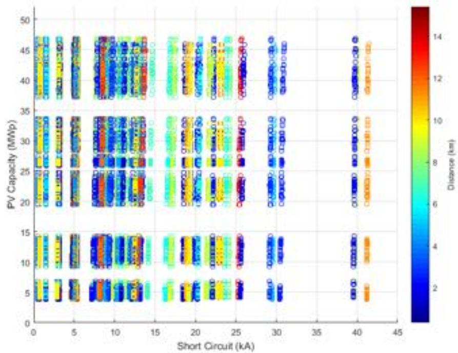
**Figure 314.** PV Capacity against Short circuit current - Unity Power Factor
