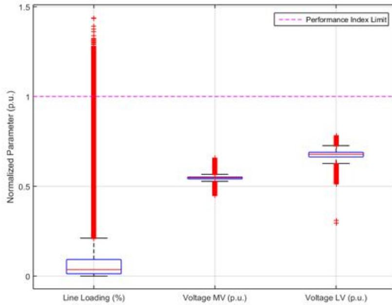
**Figure 178.** Performance Index parameters normalized to their limit – Power Factor equal to 0.95.
