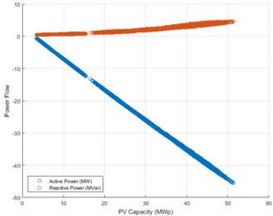
**Figure 312.** Power flow at PCC (connection of the reference substation with HV network) against PV capacity - Unity Power Factor (negative sign denotes reverse power flow).
