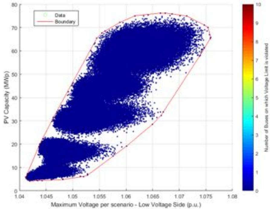
**Figure 201.** PV Capacity against Voltage – Low voltage side - Unity Power Factor.
