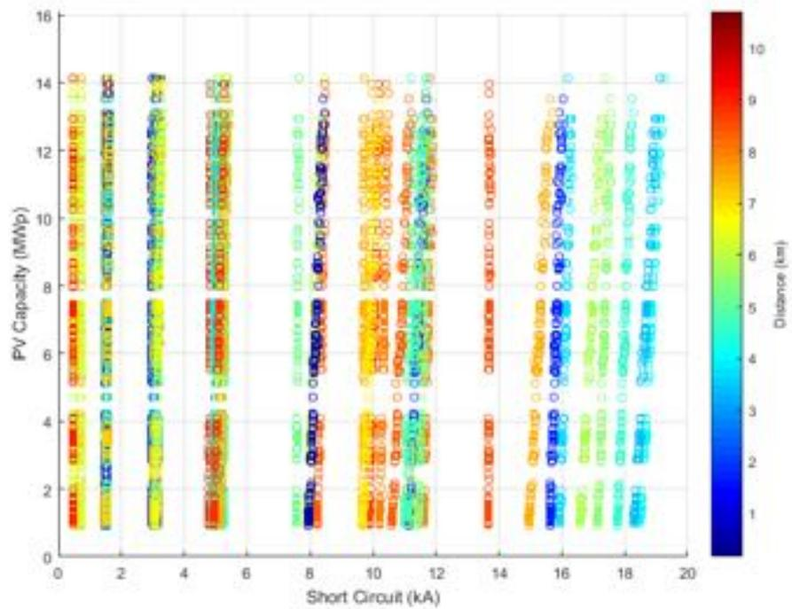
**Figure 102.** PV Capacity against Short circuit current - Unity Power Factor.
