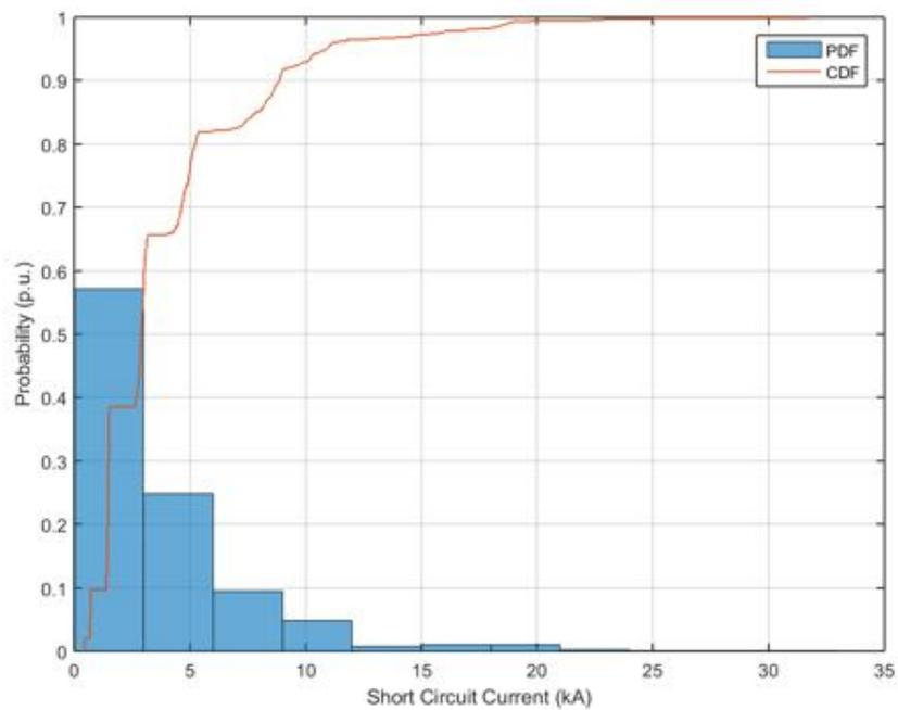
**Figure 249.** Probability distribution and cumulative probability distribution – Short Circuit Current – Power Factor equal to 0.95.
