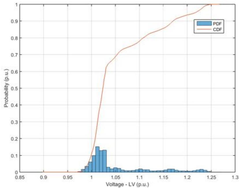
**Figure 131.** Probability distribution and cumulative probability distribution – Voltage at low voltage side – Power Factor  $\cos\phi(P)$ .
