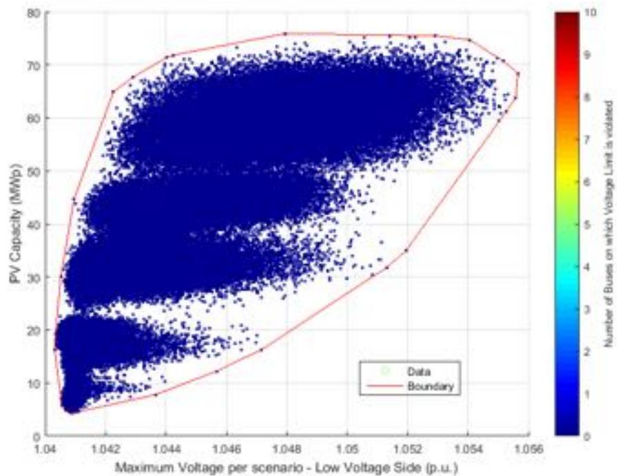
**Figure 209.** PV Capacity against Voltage – Low voltage side - Power Factor equal to 0.95.
