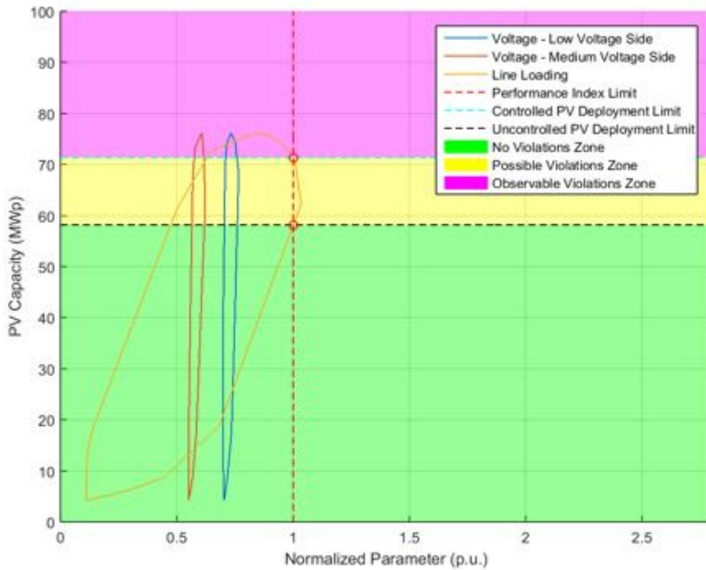
**Figure 220.** Normalized performance index parameters - Power Factor  $\cos\phi(P)$ .
