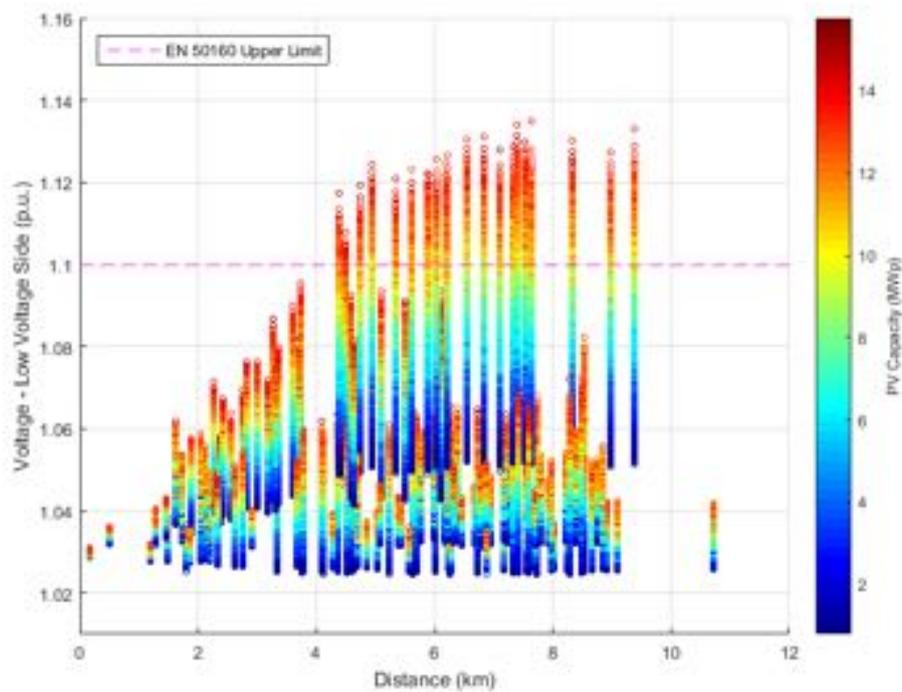
**Figure 107.** Voltage at low voltage side against Distance from transmission substation - Power Factor equal to 0.95.
