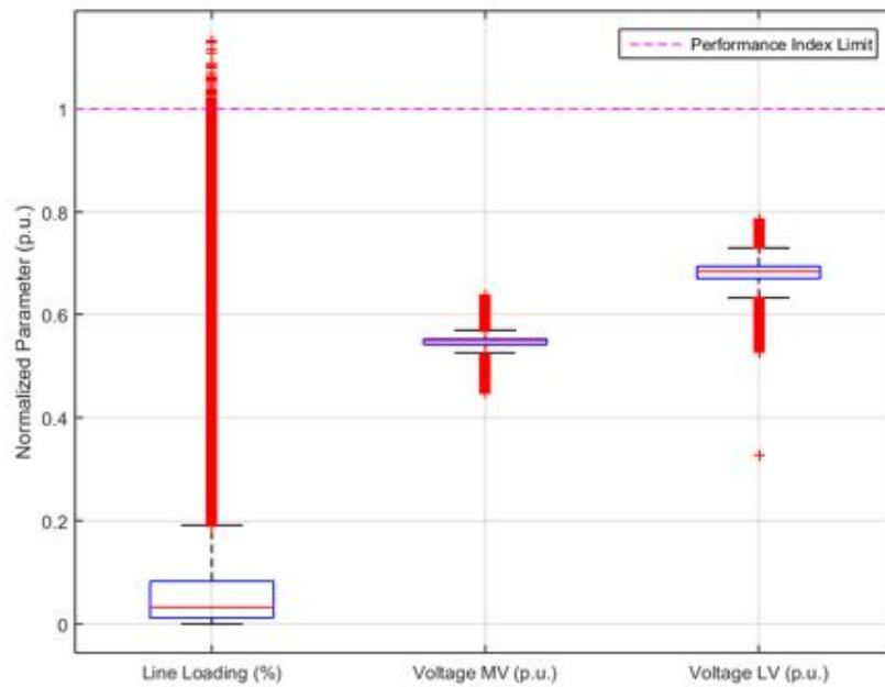
**Figure 183.** Performance Index parameters normalized to their limit – Power Factor  $\cos\phi(P)$ .
