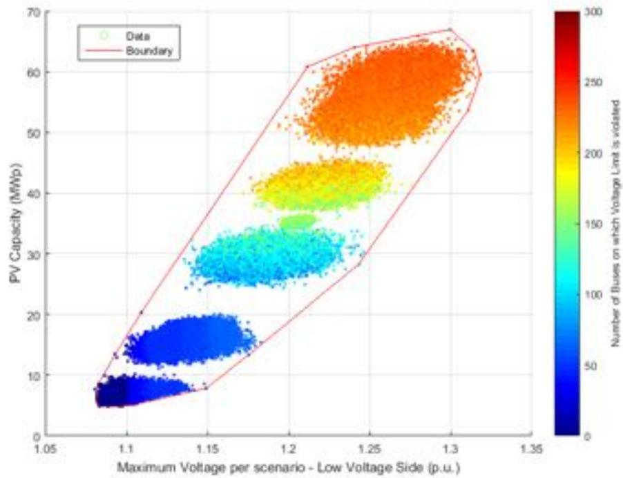
**Figure 270.** PV Capacity against Voltage – Low voltage side - Power Factor  $\cos\phi(P)$ .
