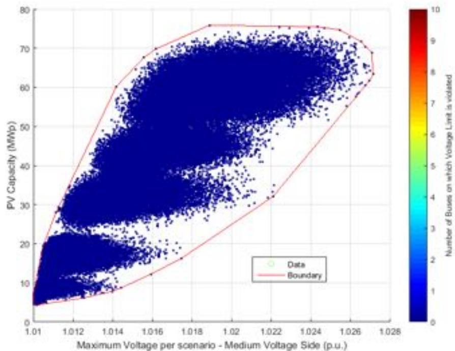
**Figure 210.** PV Capacity against Voltage – Medium voltage side - Power Factor equal to 0.95.
