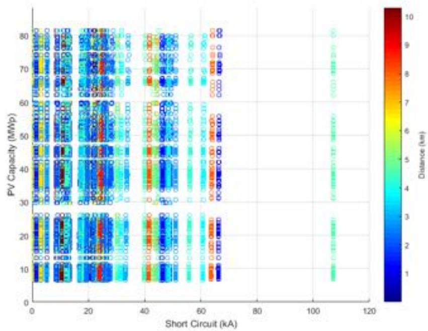
**Figure 49.** PV Capacity against Short circuit current - Unity Power Factor.
