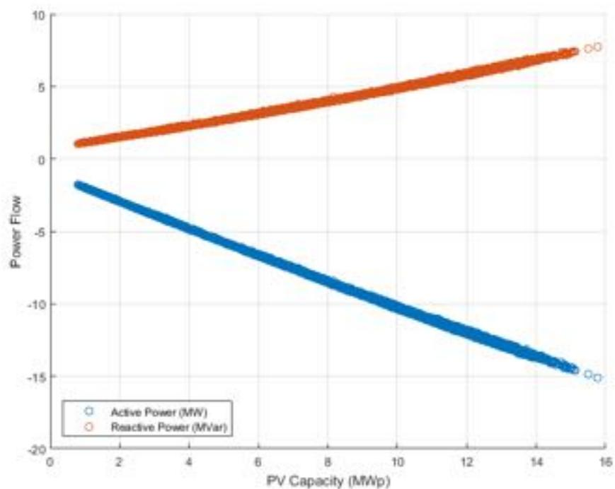
**Figure 108.** Power flow at PCC (connection of the reference substation with HV network) vs PV Capacity - Power Factor equal to 0.95.
