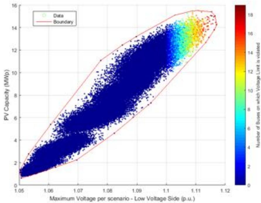
**Figure 111.** PV Capacity against Voltage – Low voltage side - Power Factor  $\cos\phi(P)$ .
