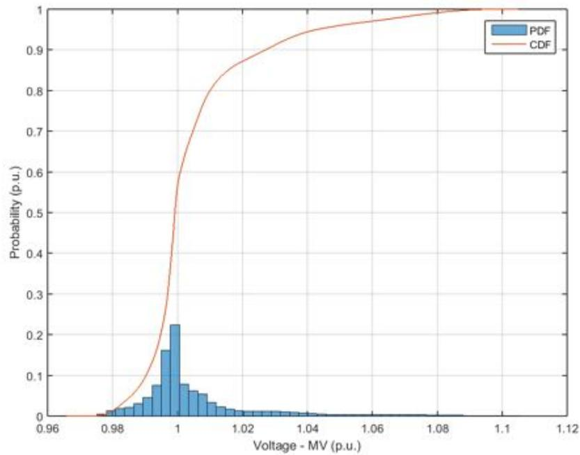
**Figure 74.** Probability distribution and cumulative probability distribution – Voltage at medium voltage side – Power Factor equal to 0.95.
