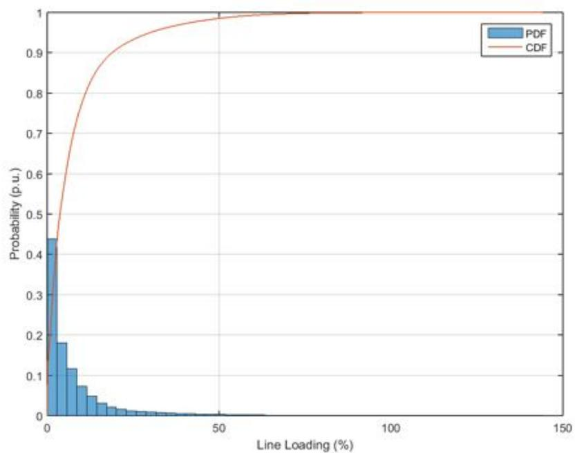
**Figure 181.** Probability distribution and cumulative probability distribution – Line Loading – Power Factor equal to 0.95.
