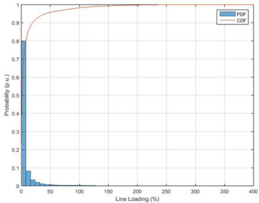
**Figure 133.** Probability distribution and cumulative probability distribution – Line Loading – Power Factor  $\cos\phi(P)$ .
