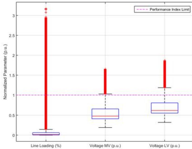
**Figure 125.** Performance Index parameters normalized to their limit – Power Factor equal to 0.95.
