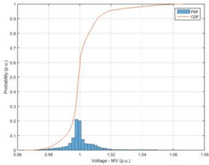
**Figure 21.** Probability distribution and cumulative probability distribution – Voltage at medium voltage side – Power Factor equal to 0.95.
