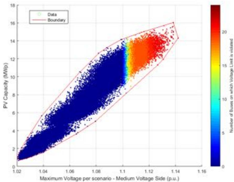
**Figure 96.** PV Capacity against Voltage – Medium voltage side - Unity Power Factor.
