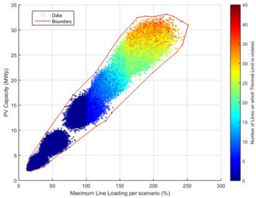
**Figure 166.** PV Capacity against Line Loading - Power Factor  $\cos\phi(P)$ .
