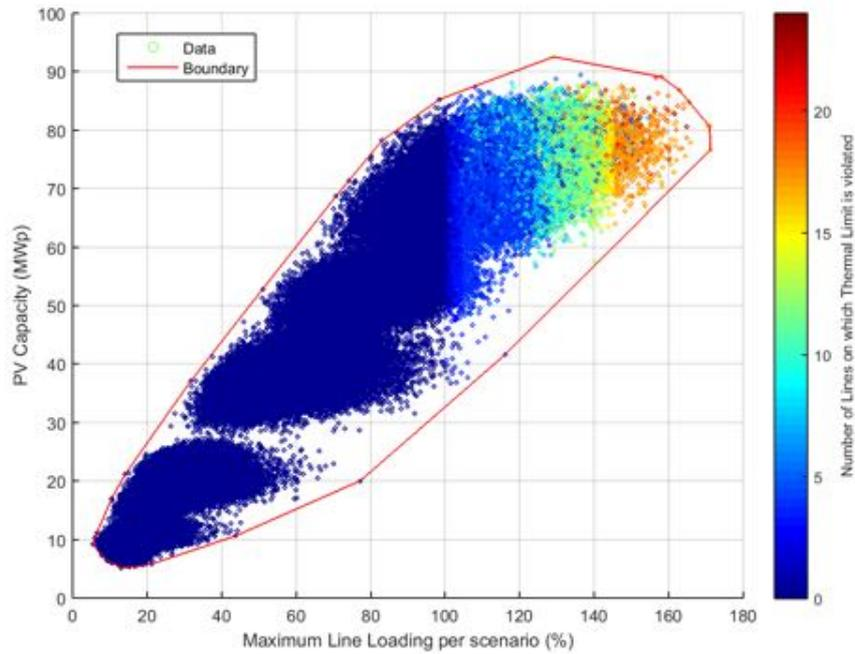
**Figure 44.** PV Capacity against Line Loading - Unity Power Factor.
