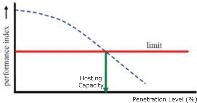
**Figure 1.** Definition of hosting capacity with the help of performance index [3].
