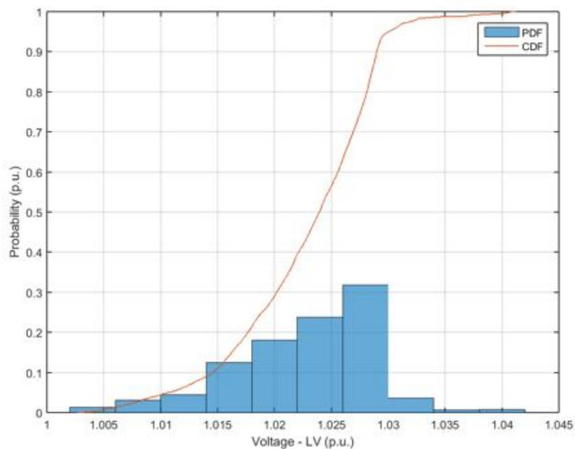
**Figure 300.** Probability distribution and cumulative probability distribution – Voltage at low voltage side – Power Factor equal to 0.95.
