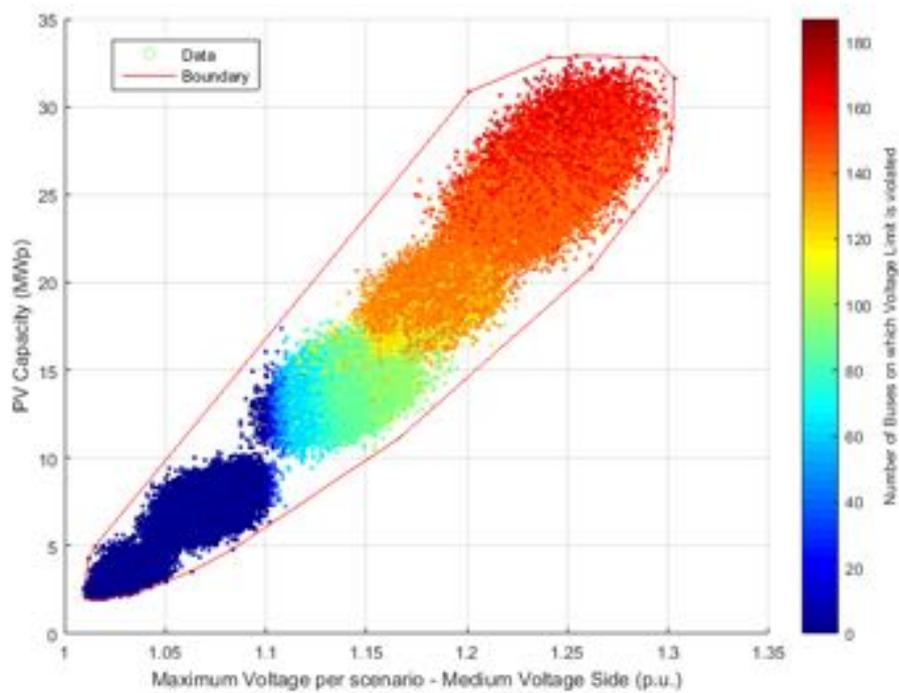
**Figure 149.** PV Capacity against Voltage – Medium voltage side - Unity Power Factor.
