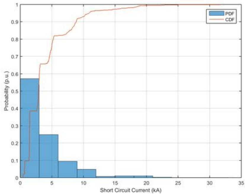
**Figure 253.** Probability distribution and cumulative probability distribution – Short Circuit Current – Power Factor  $\cos\phi(P)$ .
