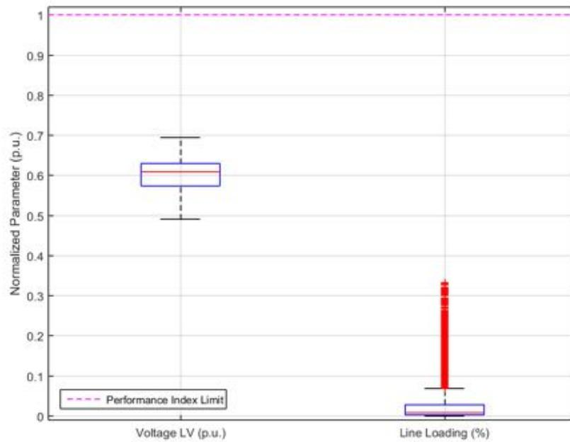
**Figure 91.** Performance Index parameters normalized to their limit – Power Factor  $\cos\phi(P)$ .
