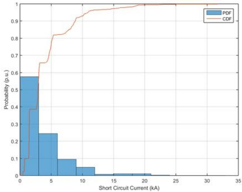
**Figure 241.** Probability distribution and cumulative probability distribution – Short Circuit Current – No PV.
