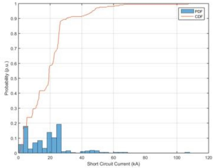
**Figure 28.** Probability distribution and cumulative probability distribution – Short Circuit Current – Power Factor  $\cos\phi(P)$ .
