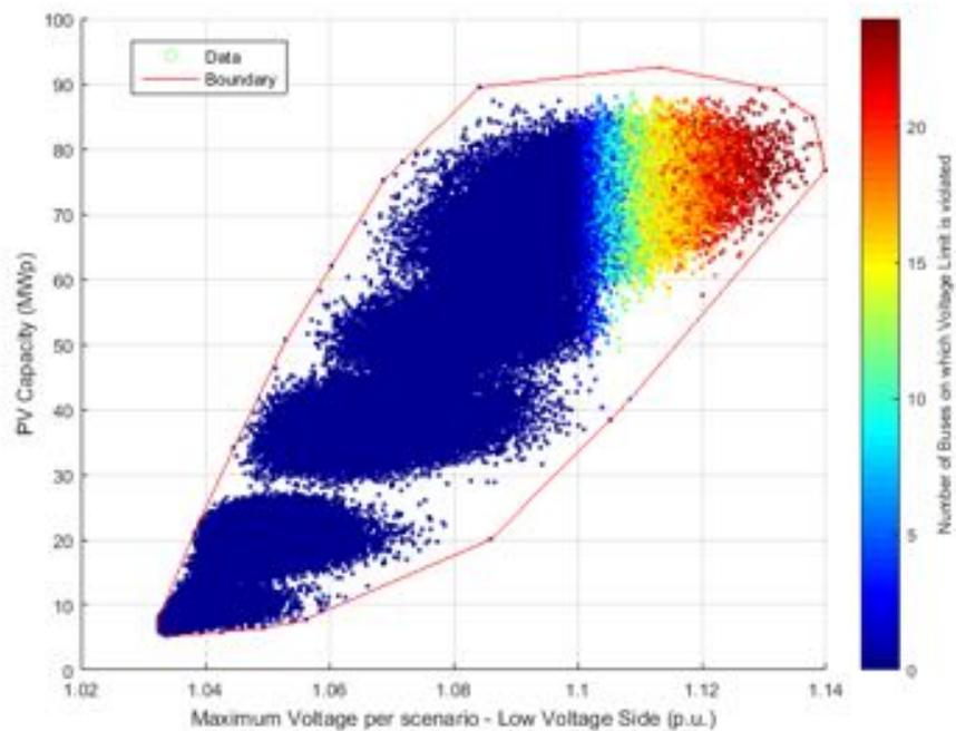
**Figure 42.** PV Capacity against Voltage – Low voltage side - Unity Power Factor.
