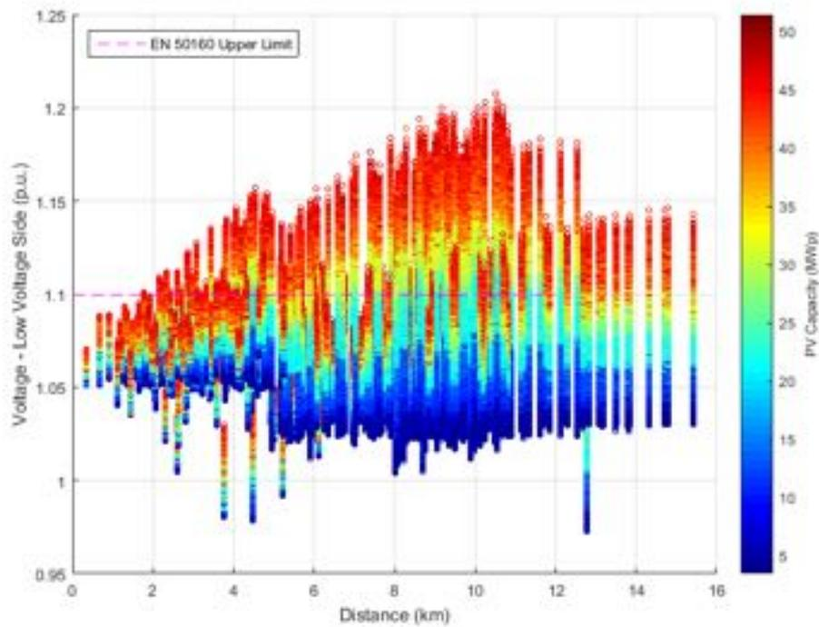
**Figure 311.** Voltage at low voltage side against distance from transmission substation - Unity Power Factor.
