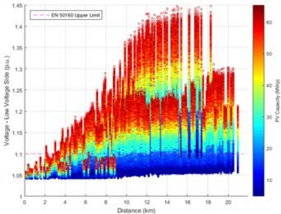
**Figure 258.** Voltage at low voltage side against distance from transmission substation - Unity Power Factor.
