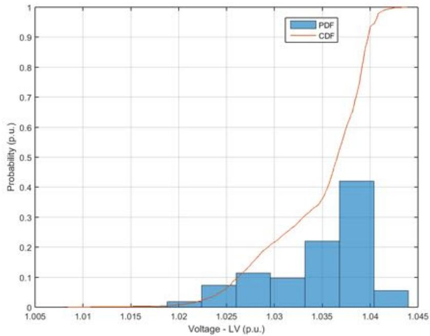
**Figure 198.** Probability distribution and cumulative probability distribution – Voltage at low voltage side – Power Factor  $\cos\phi(P)$ .
