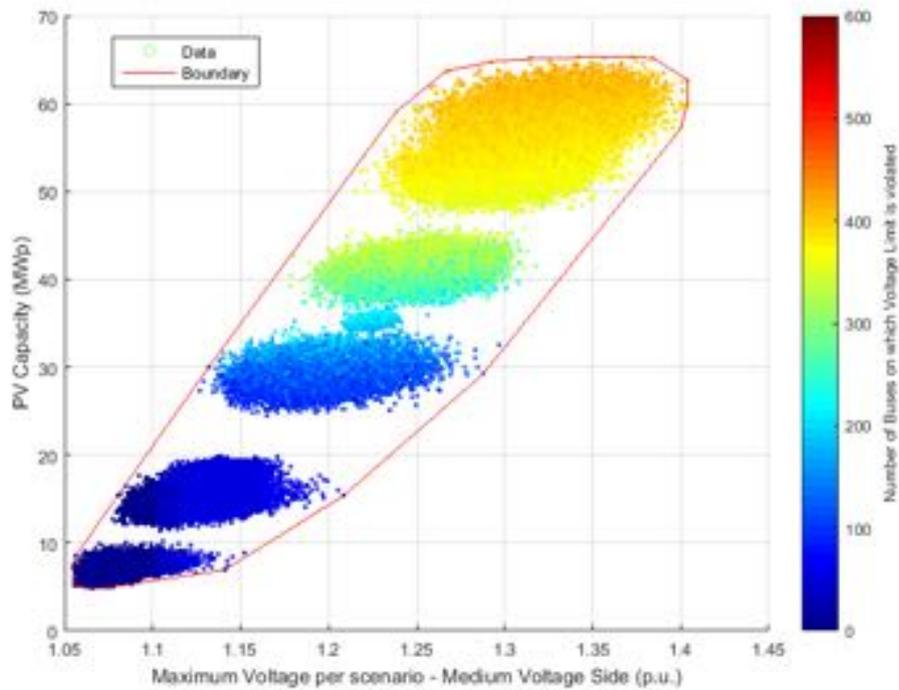
**Figure 255.** PV Capacity against Voltage – Medium voltage side - Unity Power Factor.
