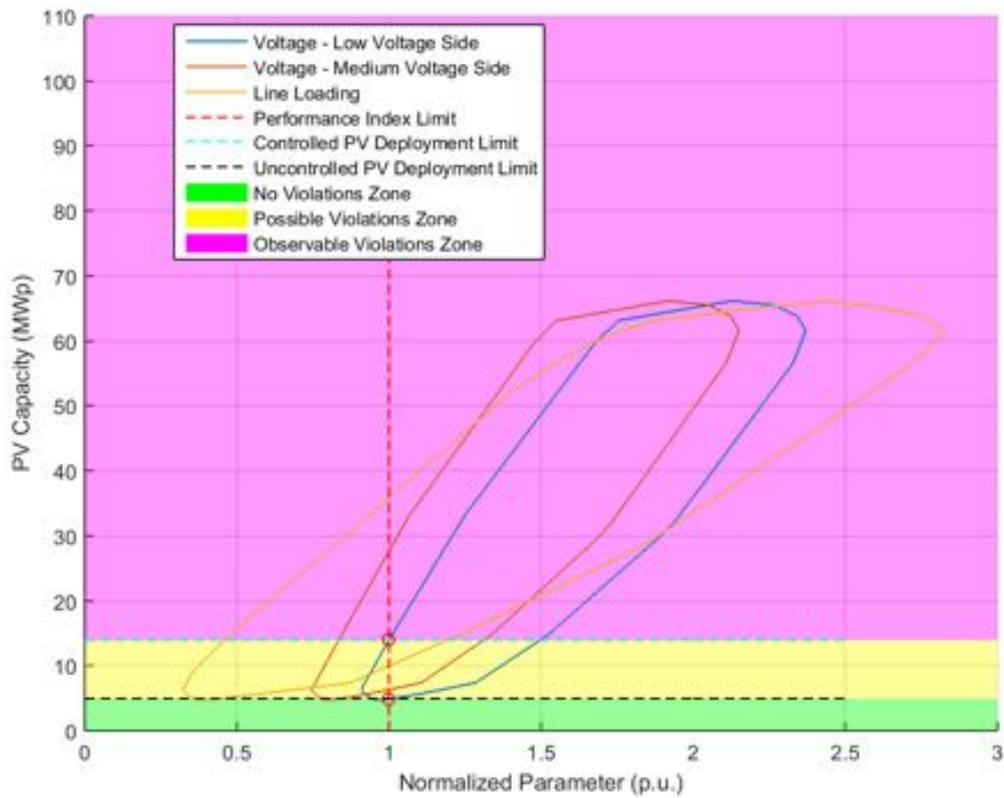
**Figure 265.** Normalized performance index parameters - Power Factor equal to 0.95.
