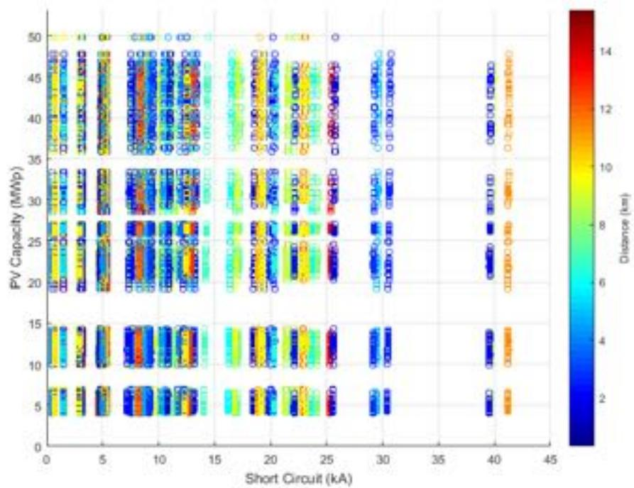
**Figure 322.** PV Capacity against Short Circuit current - Power Factor equal to 0.95.
