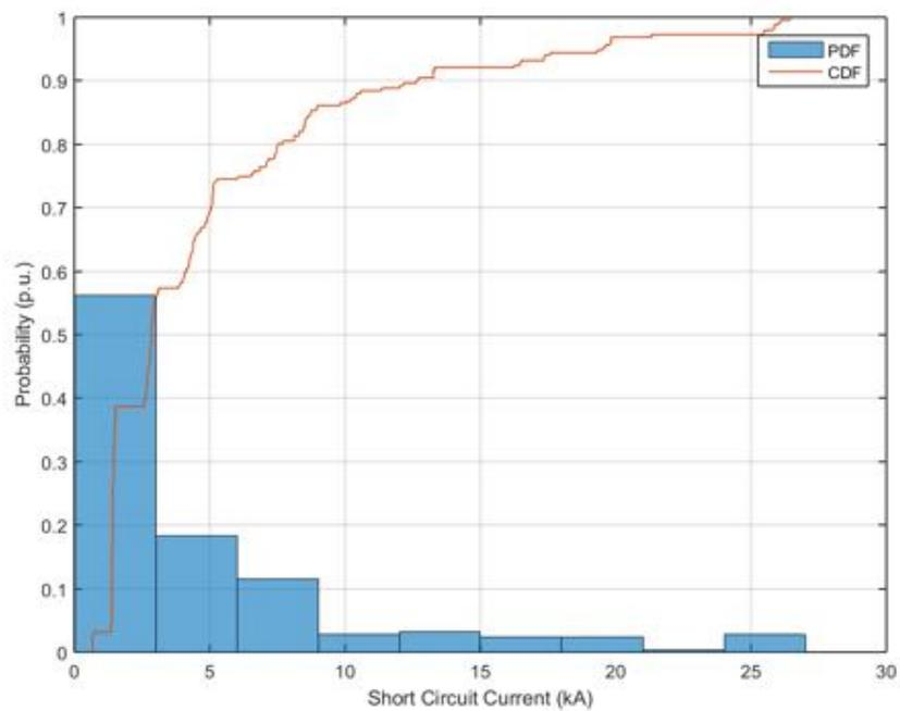
**Figure 143.** Probability distribution and cumulative probability distribution – Short Circuit Current – Power Factor equal to 0.95.
