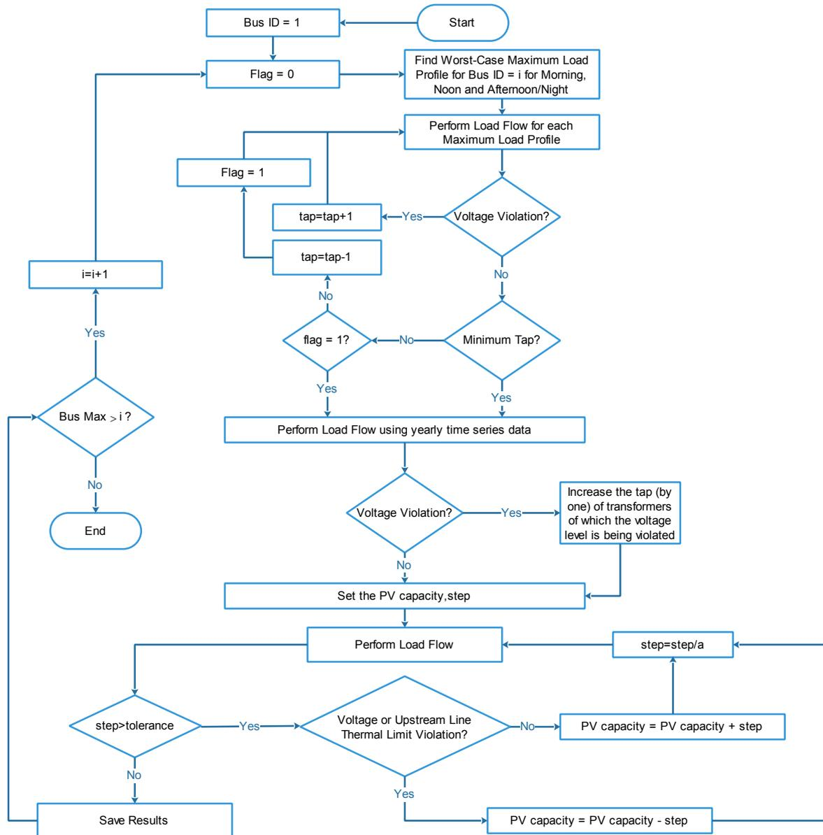
**Figure 7.** Flowchart of maximum PV capacity per substation methodology.
