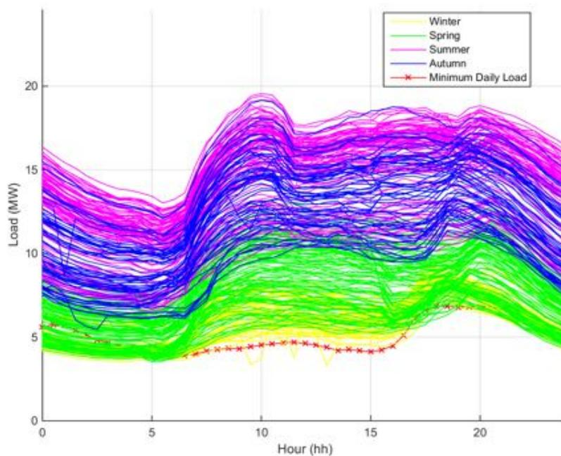
**Figure 331.** Sotera S/S - Minimum daily load.
