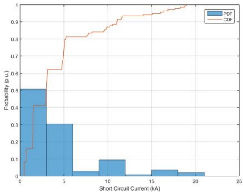
**Figure 90.** Probability distribution and cumulative probability distribution – Short Circuit Current – Power Factor equal to 0.95.
