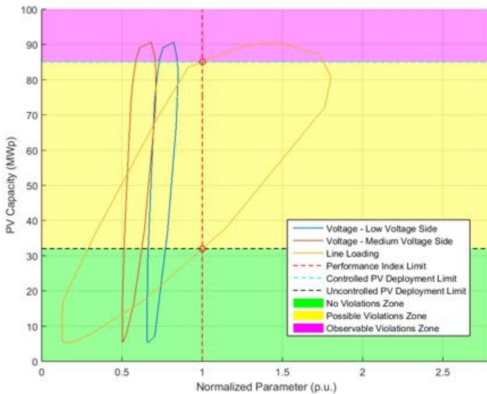
**Figure 61.** Normalized performance index parameters - Power Factor  $\cos\phi(P)$ .
