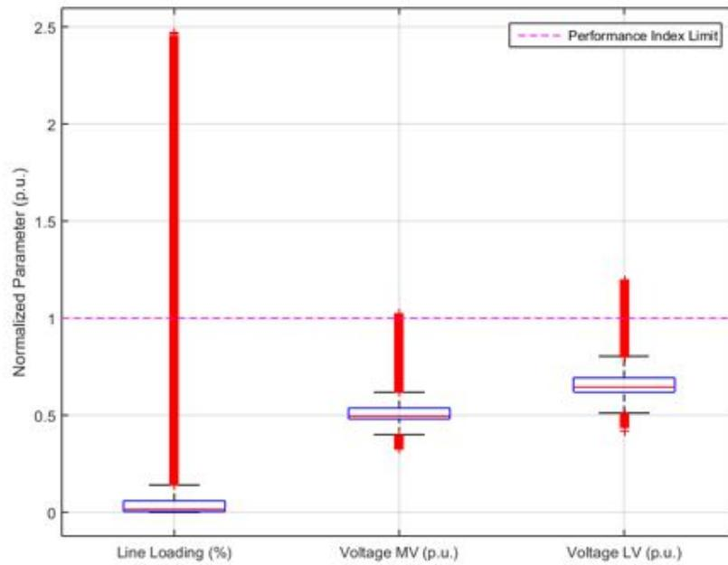
**Figure 72.** Performance Index parameters normalized to their limit – Power Factor equal to 0.95.
