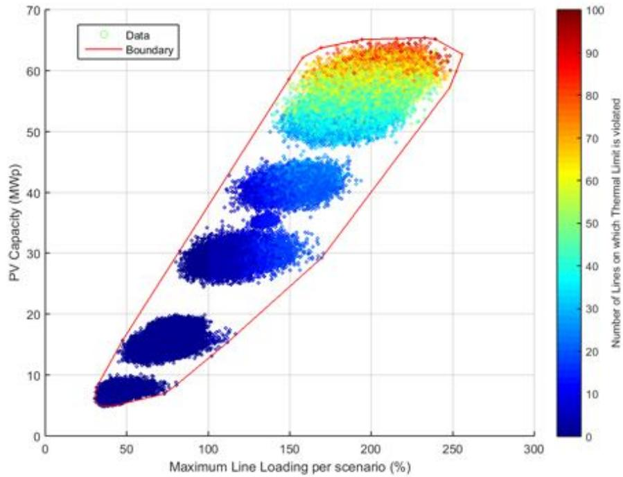
**Figure 256.** PV Capacity against Line Loading - Unity Power Factor.
