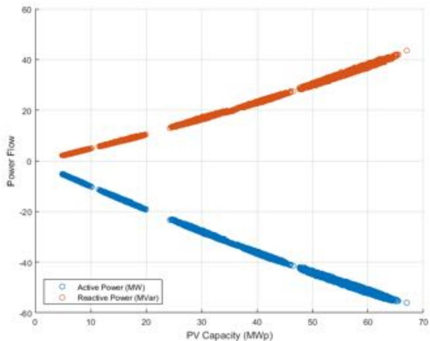
**Figure 275.** Power flow at PCC (connection of the reference substation with HV network) vs PV Capacity - Power Factor  $\cos\phi(P)$ .
