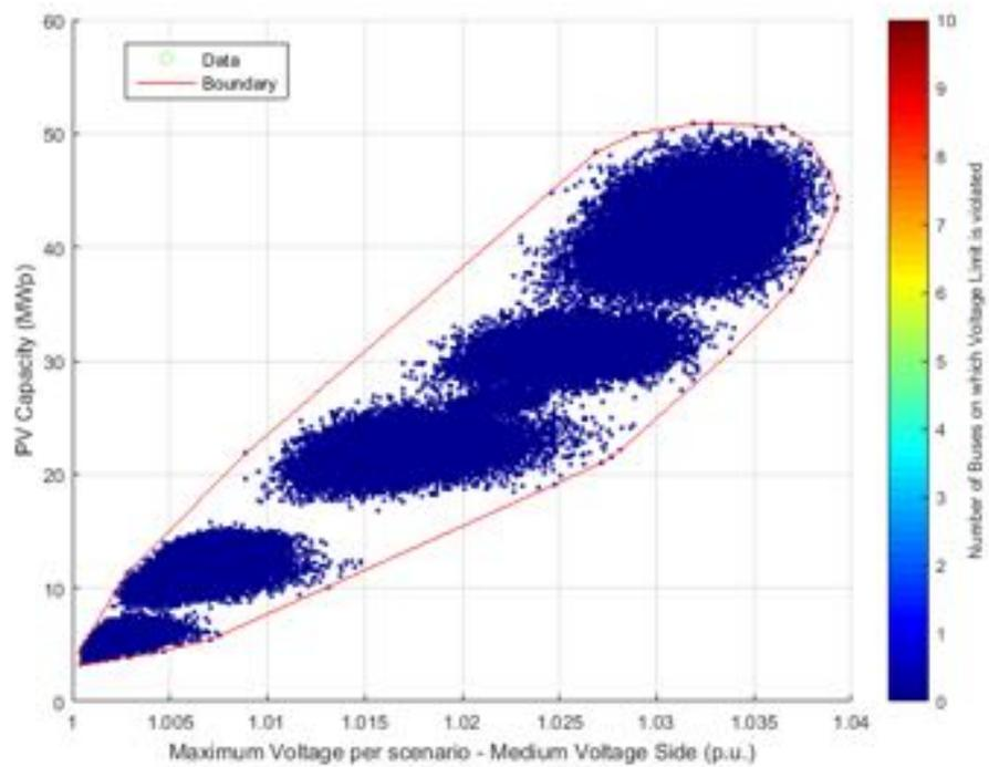
**Figure 324.** PV Capacity against Voltage – Medium voltage side - Power Factor  $\cos\phi(P)$ .
