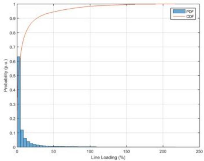
**Figure 22.** Probability distribution and cumulative probability distribution – Line Loading – Power Factor equal to 0.95.
