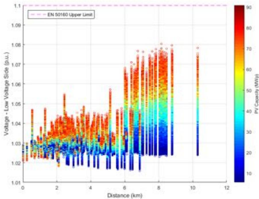
**Figure 54.** Voltage at low voltage side against Distance from transmission substation - Power Factor equal to 0.95.
