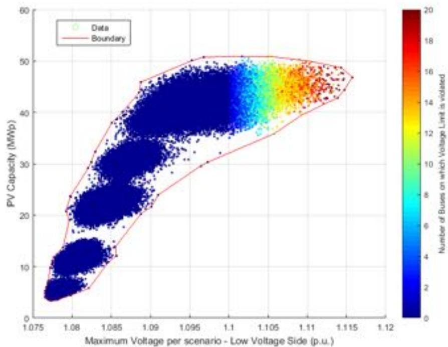
**Figure 315.** PV Capacity against Voltage – Low voltage side - Power Factor equal to 0.95.
