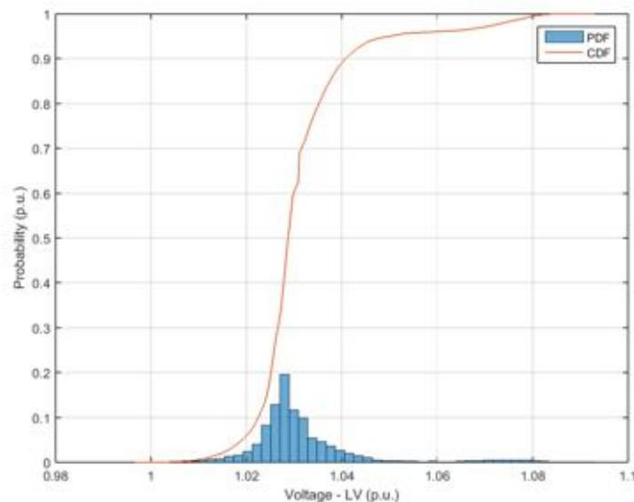
**Figure 25.** Probability distribution and cumulative probability distribution – Voltage at low voltage side – Power Factor  $\cos\phi(P)$ .
