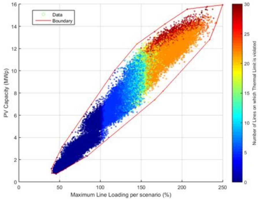
**Figure 105.** PV Capacity against Line Loading - Power Factor equal to 0.95.
