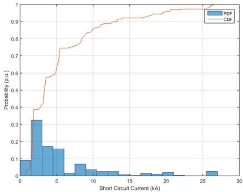
**Figure 124.** Probability distribution and cumulative probability distribution – Short Circuit Current – Unity power factor.
