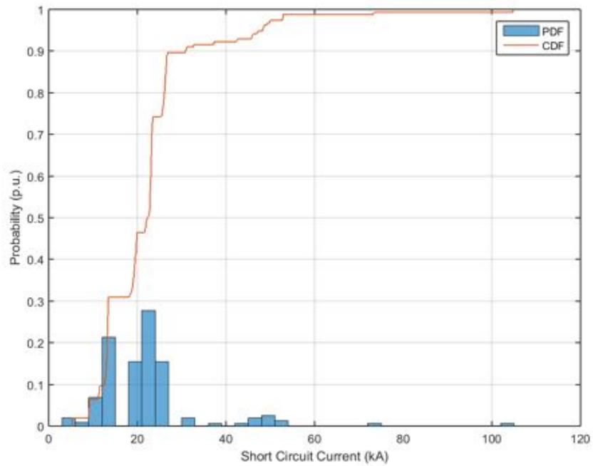
**Figure 182.** Probability distribution and cumulative probability distribution – Short Circuit Current – Power Factor equal to 0.95.
