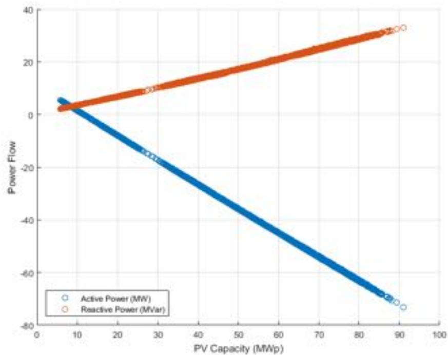
**Figure 55.** Power flow at PCC (connection of the reference substation with HV network) vs PV Capacity - Power Factor equal to 0.95.
