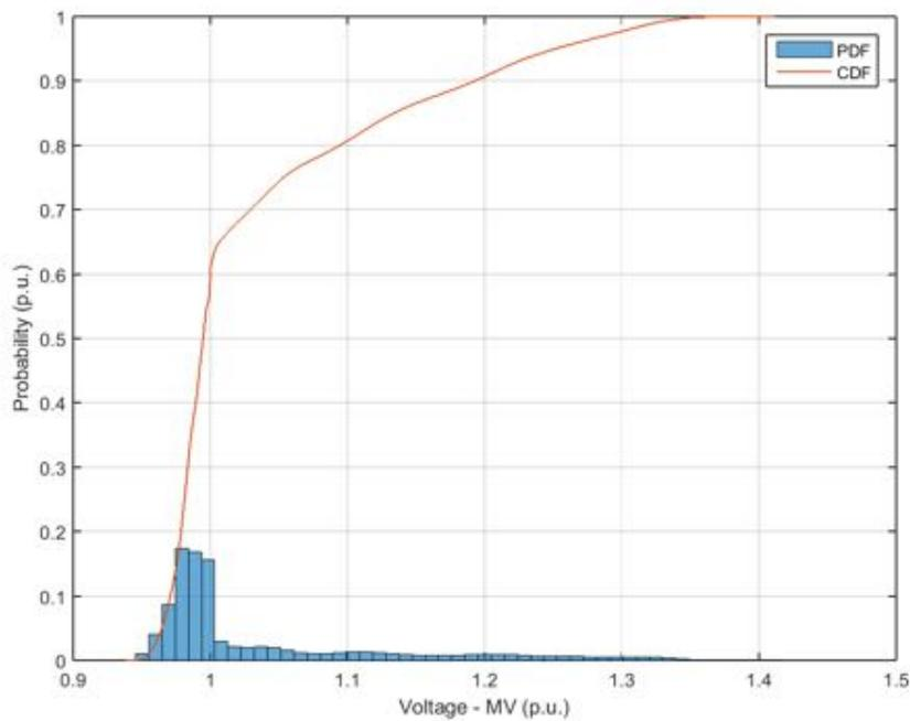
**Figure 122.** Probability distribution and cumulative probability distribution – Voltage at medium voltage side – Unity power factor.
