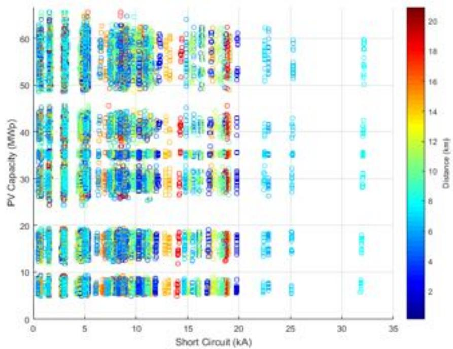
**Figure 269.** PV Capacity against Short Circuit current - Power Factor equal to 0.95.
