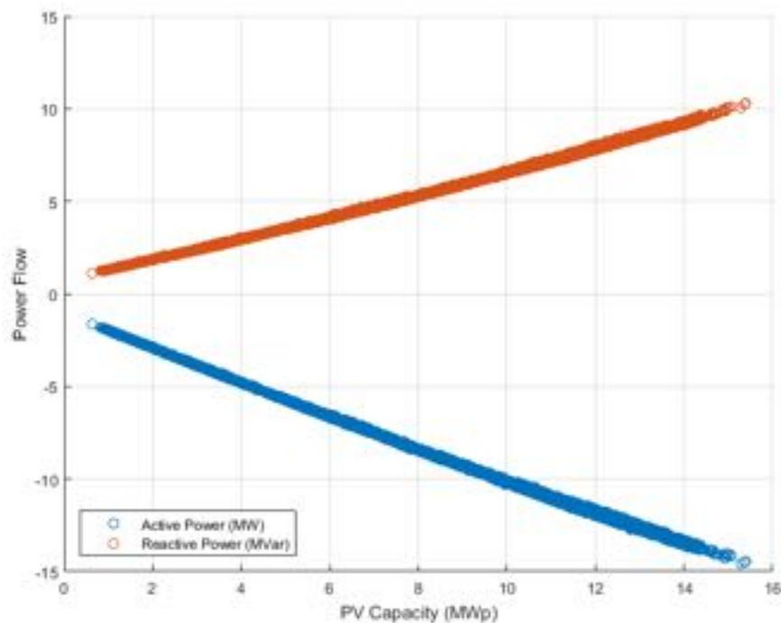
**Figure 116.** Power flow at PCC (connection of the reference substation with HV network) vs PV Capacity - Power Factor  $\cos\phi(P)$ .
