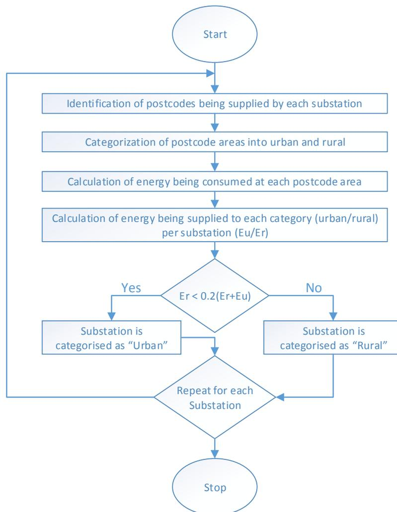
**Figure 11.** Flowchart of the methodology for the categorization of substation into urban and rural
