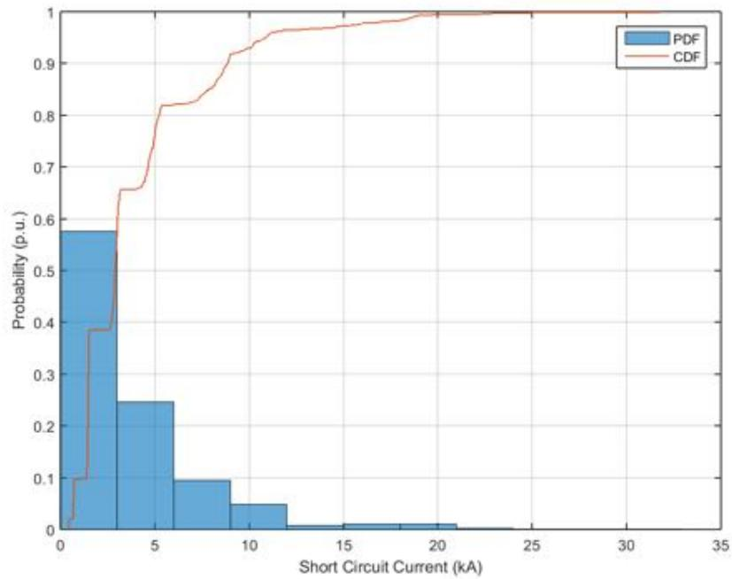
**Figure 230.** Probability distribution and cumulative probability distribution – Short Circuit Current – Unity power factor.
