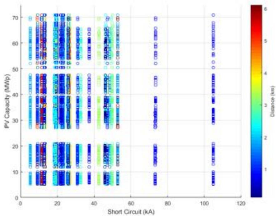
**Figure 208.** PV Capacity against Short circuit current - Unity Power Factor
