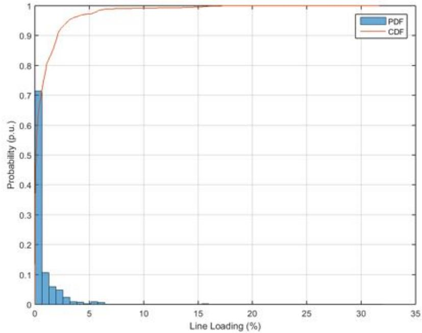
**Figure 244.** Probability distribution and cumulative probability distribution – Line Loading – Unity Power Factor.
