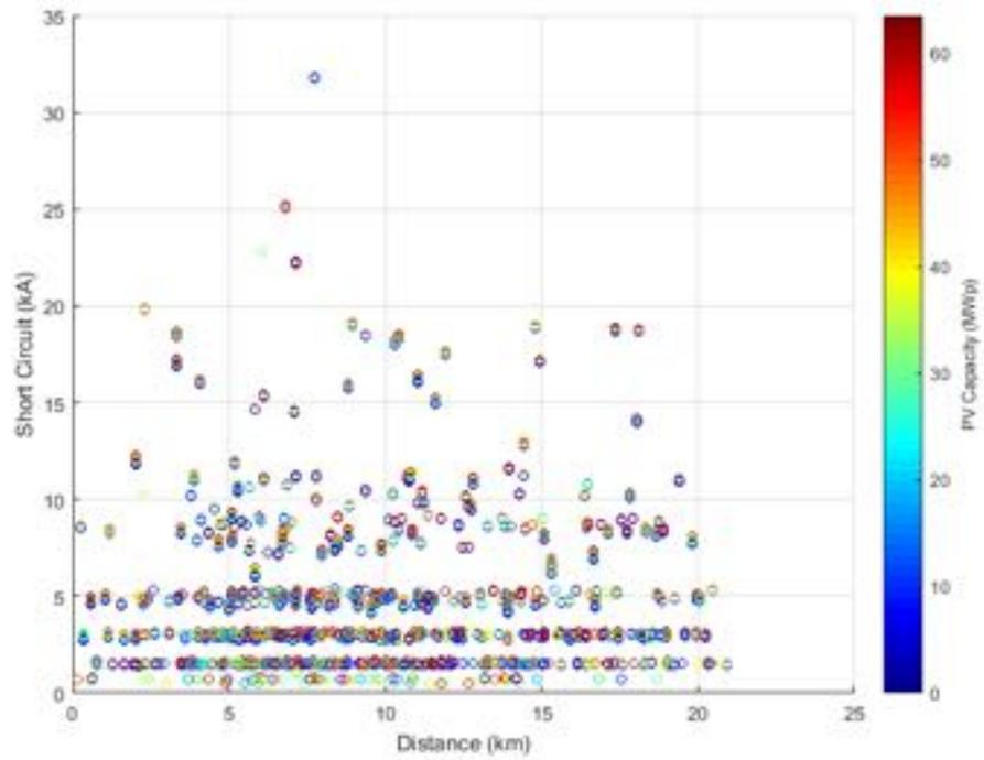
**Figure 276.** Short circuit current against distance - Power Factor  $\cos\phi(P)$ .
