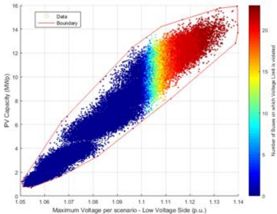
**Figure 103.** PV Capacity against Voltage – Low voltage side - Power Factor equal to 0.95.
