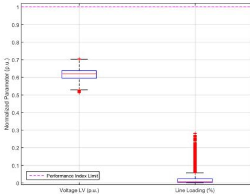
**Figure 299.** Performance Index parameters normalized to their limit – Power Factor equal to 0.95.
