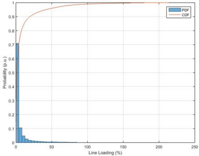
**Figure 282.** Probability distribution and cumulative probability distribution – Line Loading – Unity power factor.
