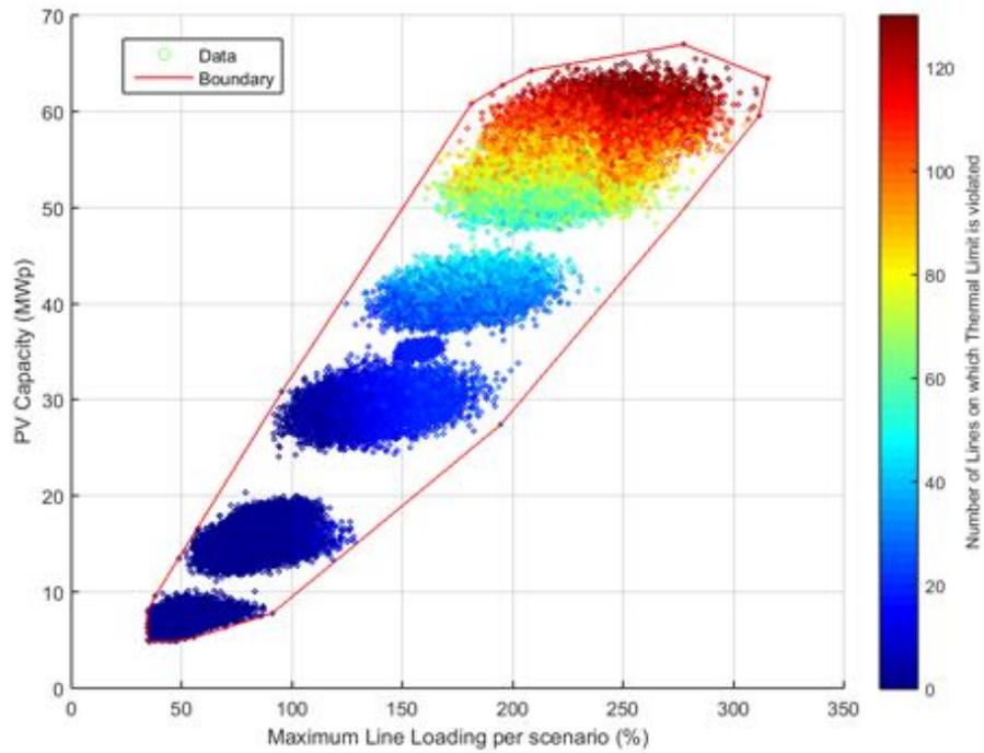
**Figure 272.** PV Capacity against Line Loading - Power Factor  $\cos\phi(P)$ .
