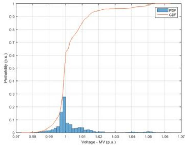
**Figure 26.** Probability distribution and cumulative probability distribution – Voltage at medium voltage side – Power Factor  $\cos\phi(P)$ .
