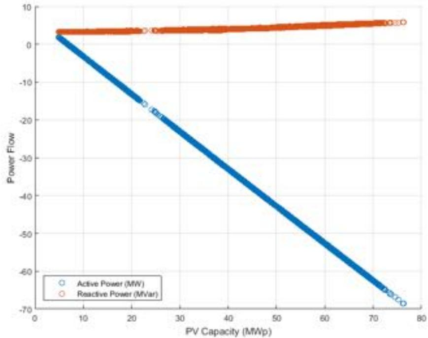
**Figure 206.** Power flow at PCC (connection of the reference substation with HV network) against PV capacity - Unity Power Factor (negative sign denotes reverse power flow).
