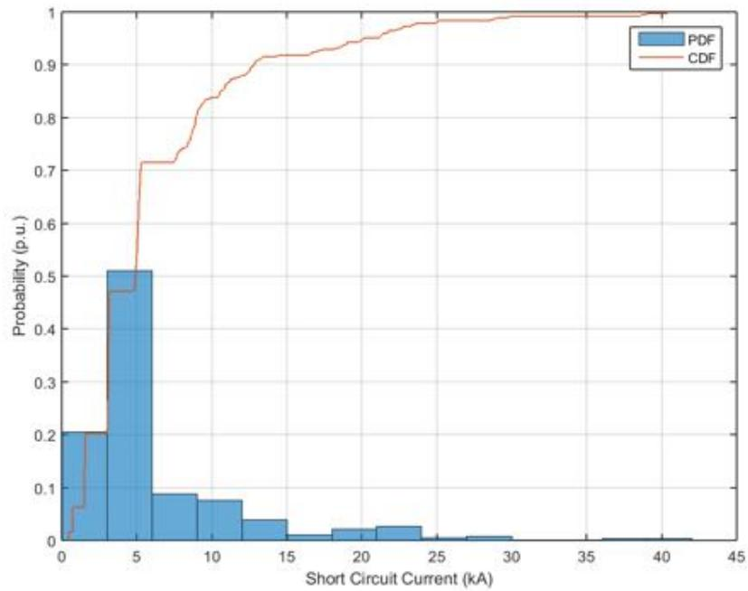
**Figure 288.** Probability distribution and cumulative probability distribution – Short Circuit Current – Power Factor equal to 0.95.
