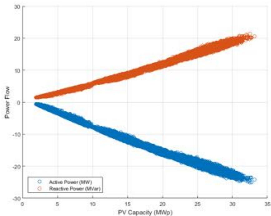
**Figure 169.** Power flow at PCC (connection of the reference substation with HV network) vs PV Capacity - Power Factor  $\cos\phi(P)$ .
