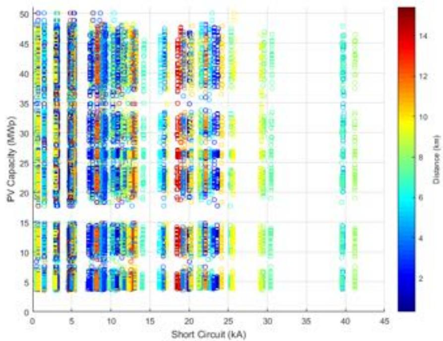
**Figure 330.** PV Capacity against short circuit current - Power Factor  $\cos\phi(P)$ .
