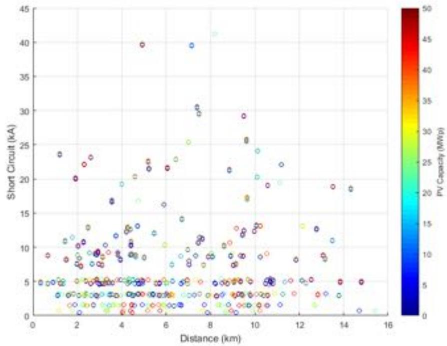
**Figure 329.** Short circuit current against distance - Power Factor  $\cos\phi(P)$ .
