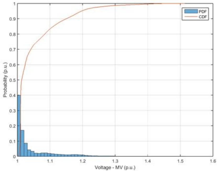
**Figure 228.** Probability distribution and cumulative probability distribution – Voltage at medium voltage side – Unity power factor.
