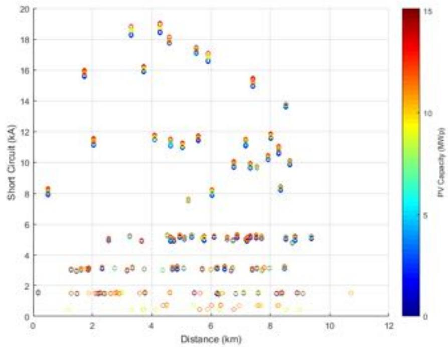
**Figure 109.** Short circuit current against Distance - Power Factor equal to 0.95.
