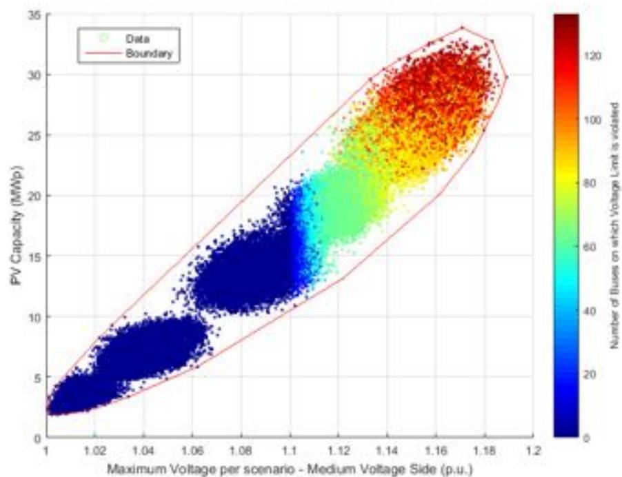
**Figure 157.** PV Capacity against Voltage – Medium voltage side - Power Factor equal to 0.95.
