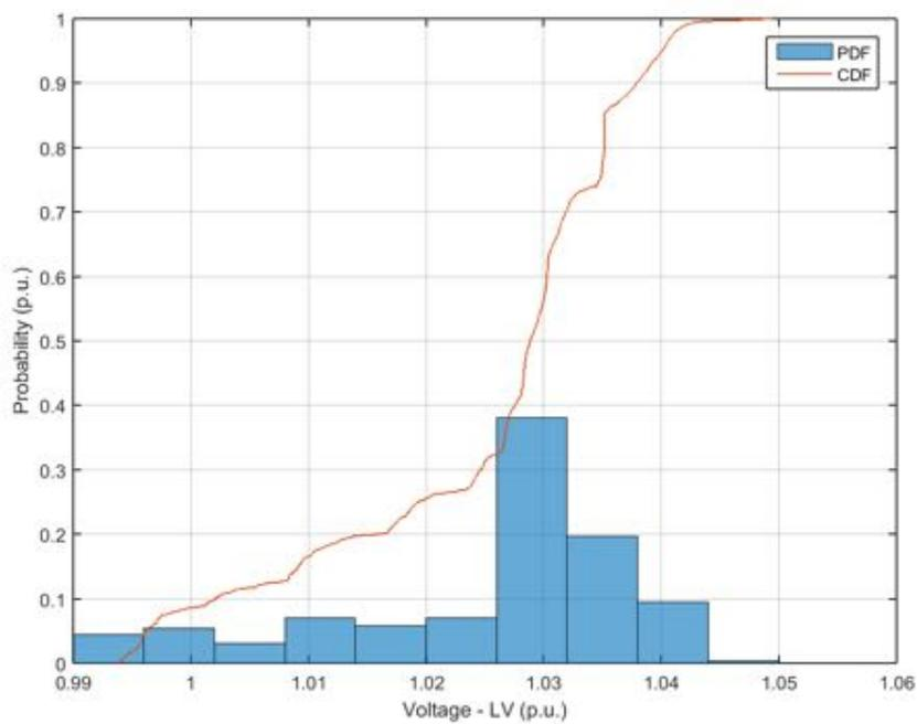
**Figure 141.** Probability distribution and cumulative probability distribution – Voltage at low voltage side – Power Factor equal to 0.95.
