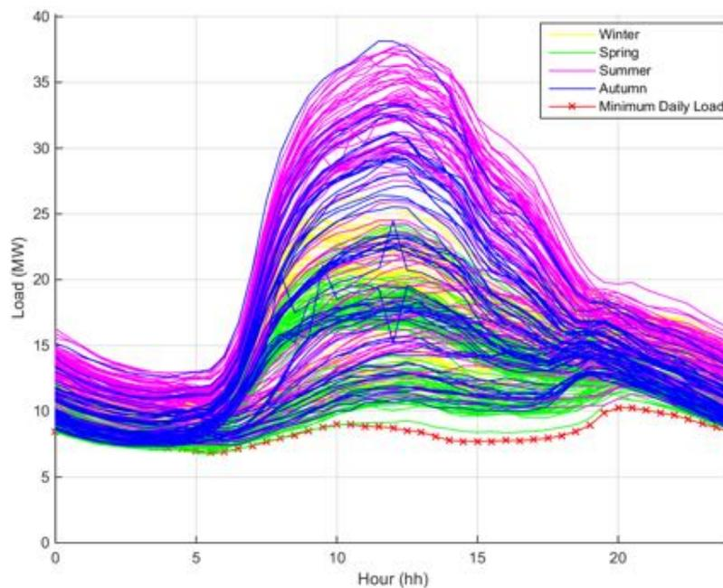
**Figure 225.** Renos Prentzas S/S - Minimum daily load.
