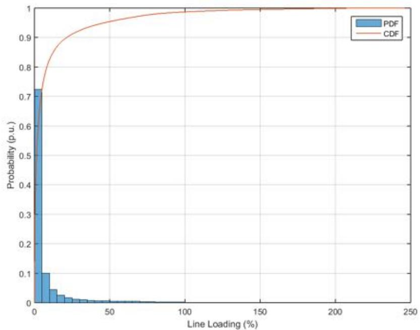
**Figure 287.** Probability distribution and cumulative probability distribution – Line Loading – Power Factor equal to 0.95.
