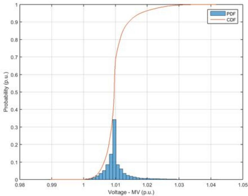
**Figure 175.** Probability distribution and cumulative probability distribution – Voltage at medium voltage side – Unity power factor.
