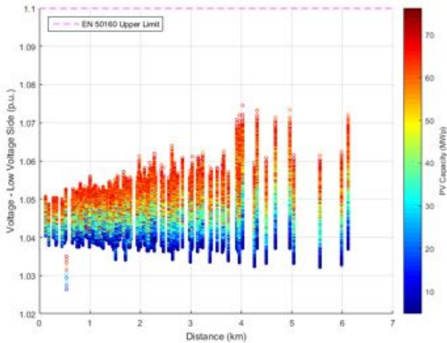
**Figure 205.** Voltage at low voltage side against distance from transmission substation - Unity Power Factor.
