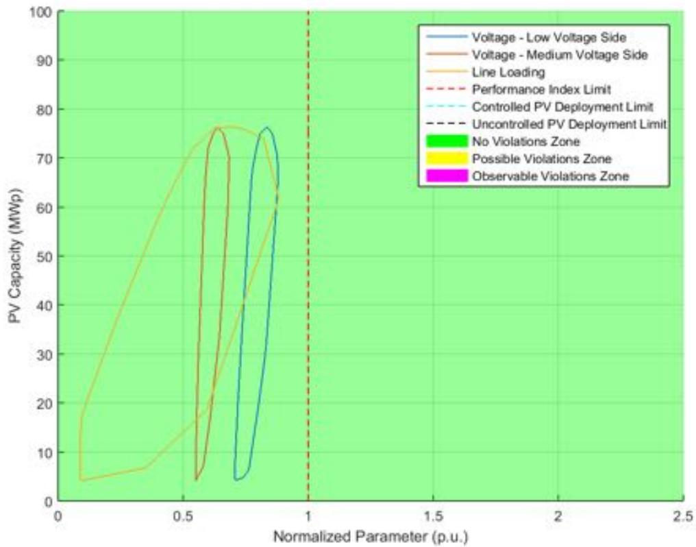
**Figure 204.** Normalized performance index parameters - Unity Power Factor.
