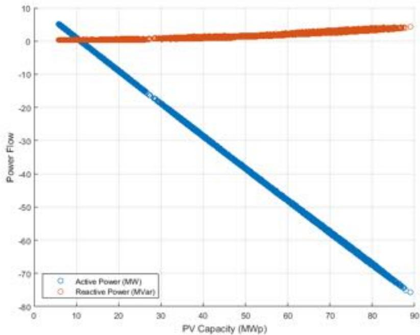
**Figure 47.** Power flow at PCC (connection of the reference substation with HV network) against PV capacity - Unity Power Factor (negative sign denotes reverse power flow).
