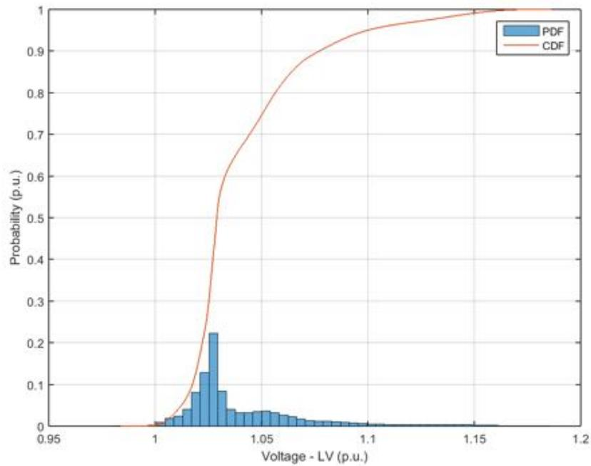
**Figure 68.** Probability distribution and cumulative probability distribution – Voltage at low voltage side – Unity power factor.
