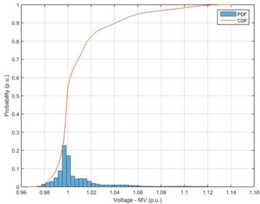
**Figure 69.** Probability distribution and cumulative probability distribution – Voltage at medium voltage side – Unity power factor.
