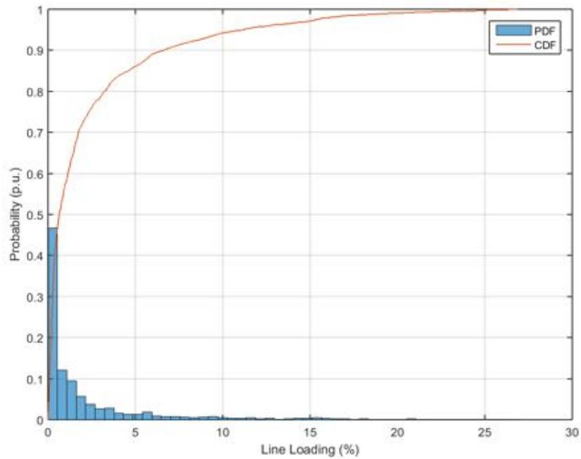
**Figure 297.** Probability distribution and cumulative probability distribution – Line Loading – Unity Power Factor.
