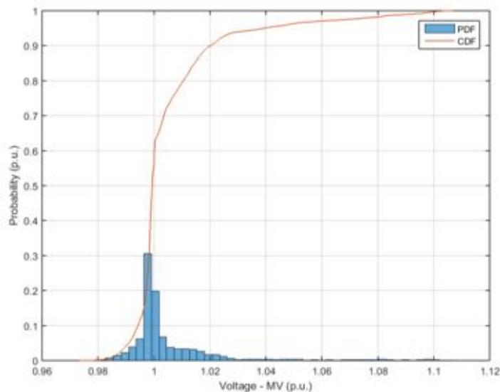
**Figure 16.** Probability distribution and cumulative probability distribution – Voltage at medium voltage side – Unity power factor.
