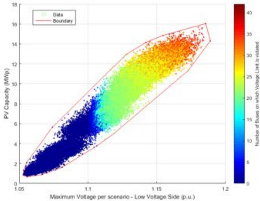
**Figure 95.** PV Capacity against Voltage – Low voltage side - Unity Power Factor.
