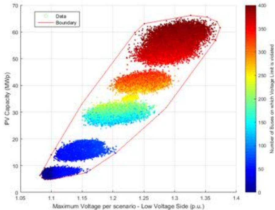
**Figure 262.** PV Capacity against Voltage – Low voltage side - Power Factor equal to 0.95.
