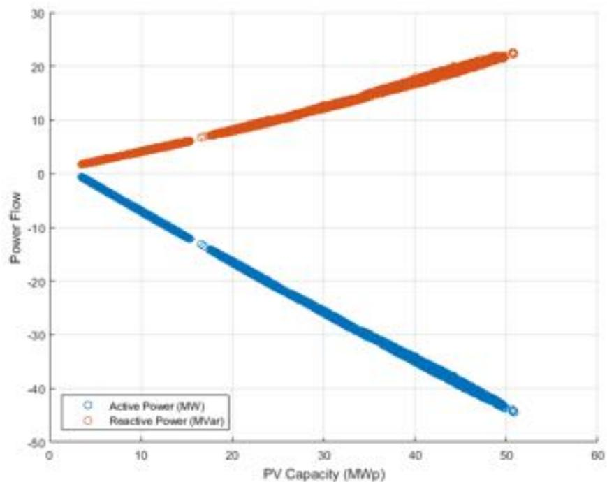
**Figure 320.** Power flow at PCC (connection of the reference substation with HV network) vs PV Capacity - Power Factor equal to 0.95.
