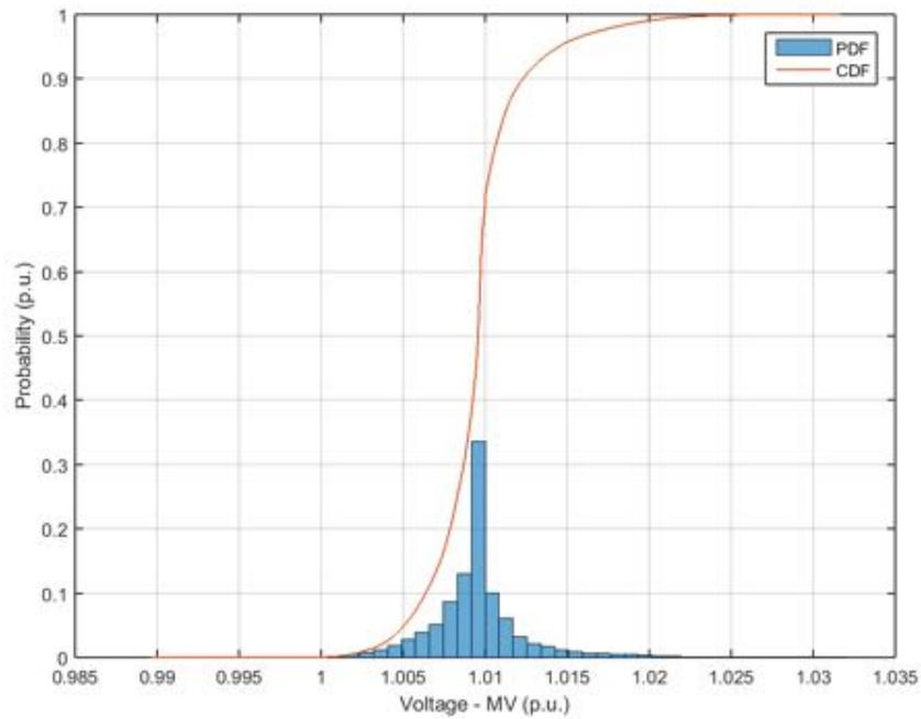
**Figure 180.** Probability distribution and cumulative probability distribution – Voltage at medium voltage side – Power Factor equal to 0.95.
