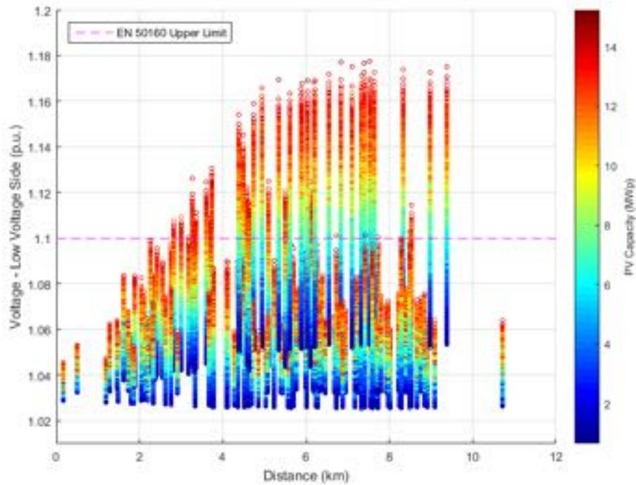
**Figure 99.** Voltage at low voltage side against distance from transmission substation - Unity Power Factor.
