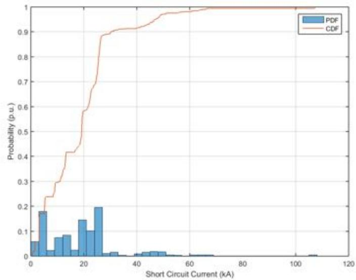
**Figure 23.** Probability distribution and cumulative probability distribution – Short Circuit Current – Power Factor equal to 0.95.
