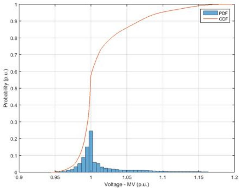
**Figure 281.** Probability distribution and cumulative probability distribution – Voltage at medium voltage side – Unity power factor.
