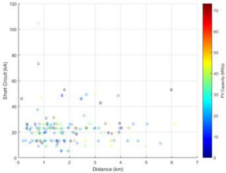
**Figure 223.** Short circuit current against distance - Power Factor  $\cos\phi(P)$ .
