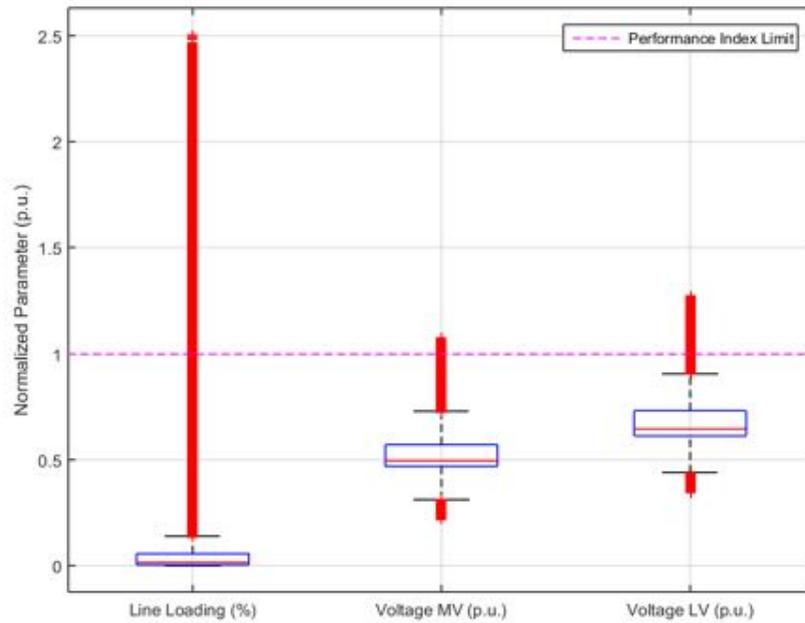
**Figure 289.** Performance Index parameters normalized to their limit – Power Factor  $\cos\phi(P)$ .
