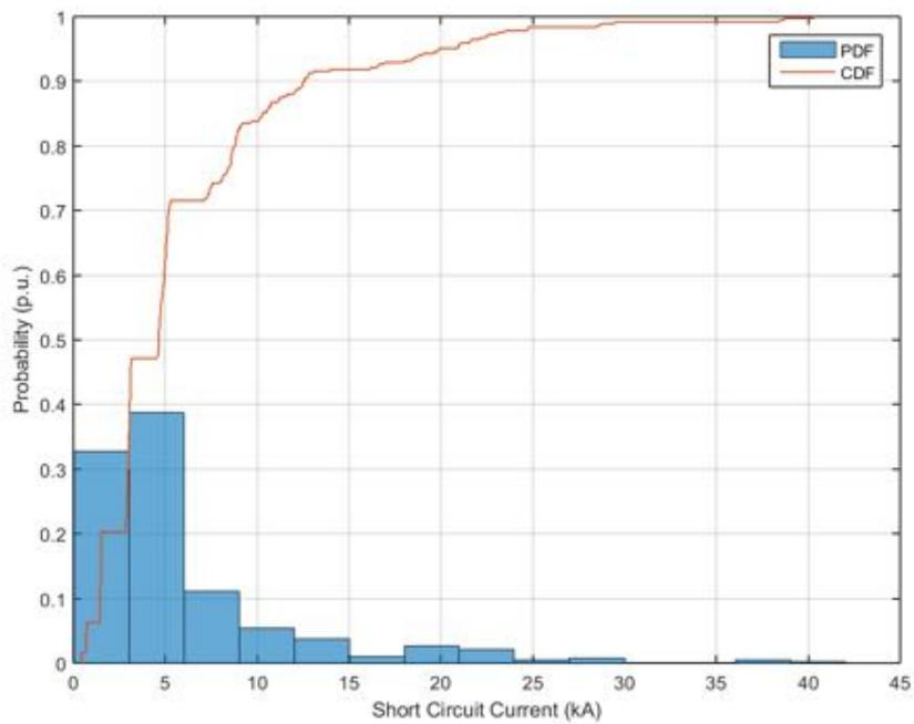
**Figure 306.** Probability distribution and cumulative probability distribution – Short Circuit Current – Power Factor  $\cos\phi(P)$ .
