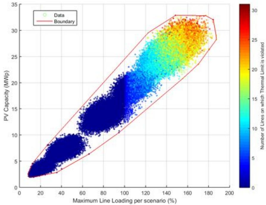
**Figure 150.** PV Capacity against Line Loading - Unity Power Factor.
