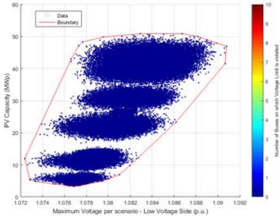
**Figure 323.** PV Capacity against Voltage – Low voltage side - Power Factor  $\cos\phi(P)$ .
