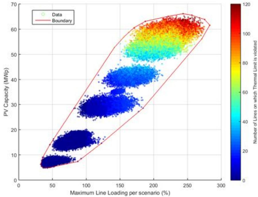
**Figure 264.** PV Capacity against Line Loading - Power Factor equal to 0.95.
