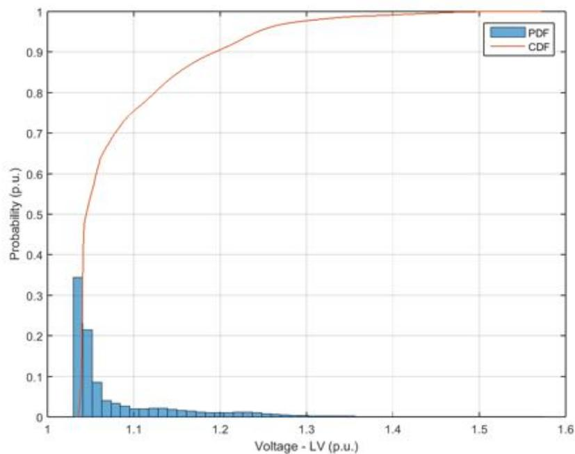
**Figure 227.** Probability distribution and cumulative probability distribution – Voltage at low voltage side – Unity power factor.
