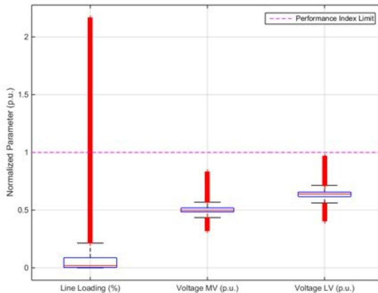
**Figure 19.** Performance Index parameters normalized to their limit – Power Factor equal to 0.95.
