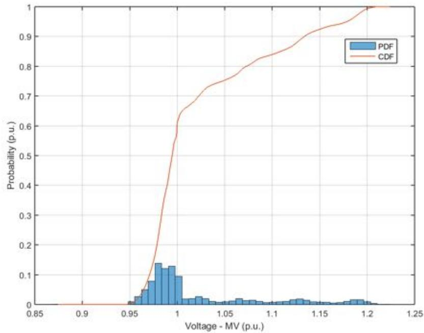
**Figure 132.** Probability distribution and cumulative probability distribution – Voltage at medium voltage side – Power Factor  $\cos\phi(P)$ .
