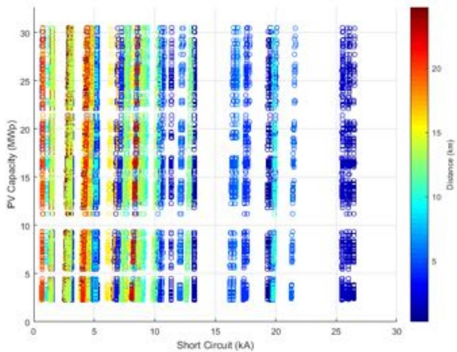
**Figure 163.** PV Capacity against Short Circuit current - Power Factor equal to 0.95.
