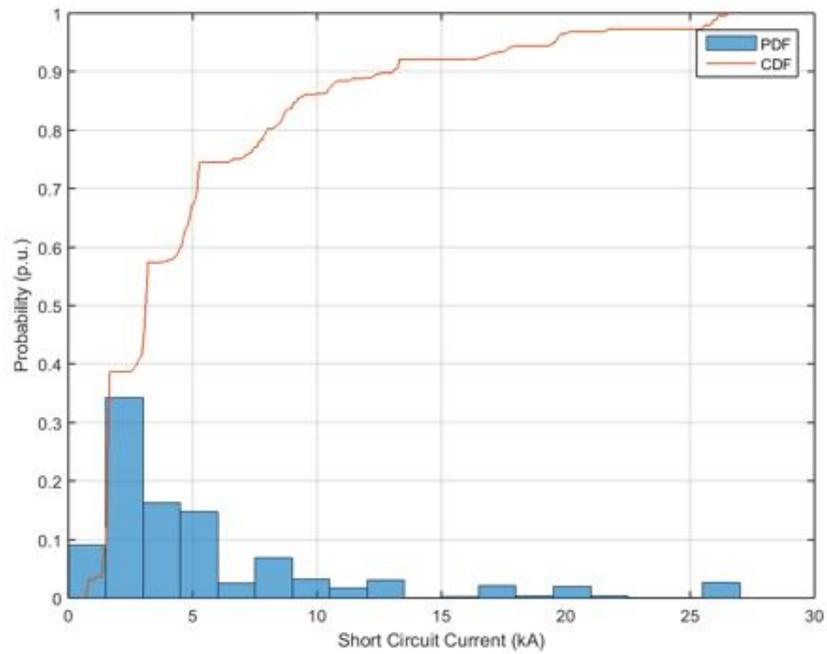
**Figure 129.** Probability distribution and cumulative probability distribution – Short Circuit Current – Power Factor equal to 0.95.
