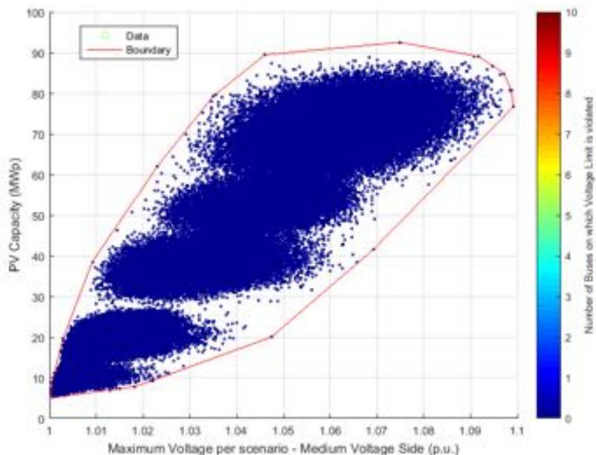
**Figure 43.** PV Capacity against Voltage – Medium voltage side - Unity Power Factor.
