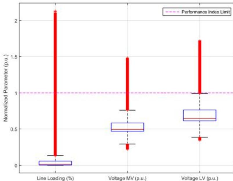
**Figure 279.** Performance Index parameters normalized to their limit – Unity Power Factor.
