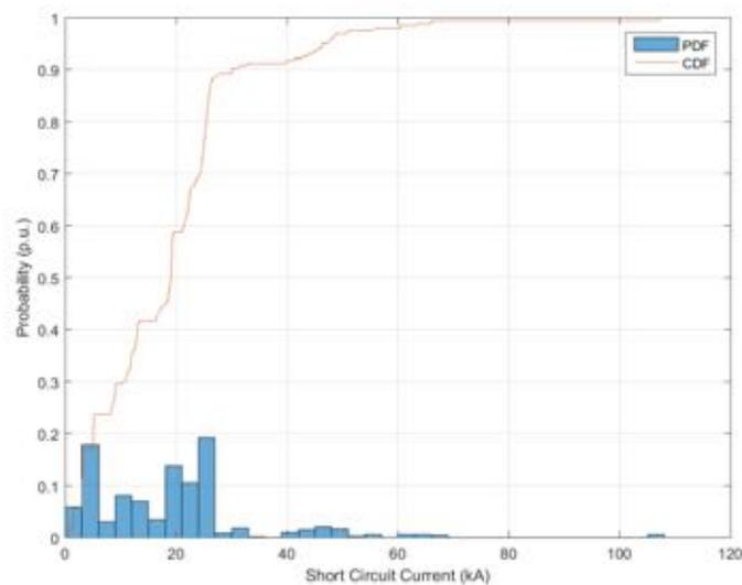
**Figure 29.** Probability distribution and cumulative probability distribution – Short Circuit Current – No PV.
