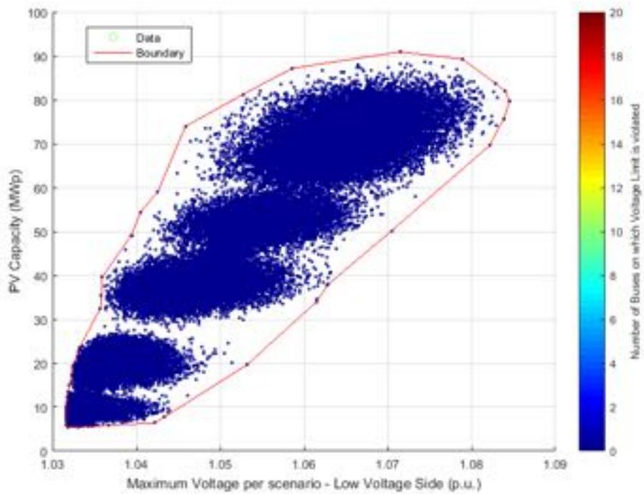
**Figure 50.** PV Capacity against Voltage – Low voltage side - Power Factor equal to 0.95.
