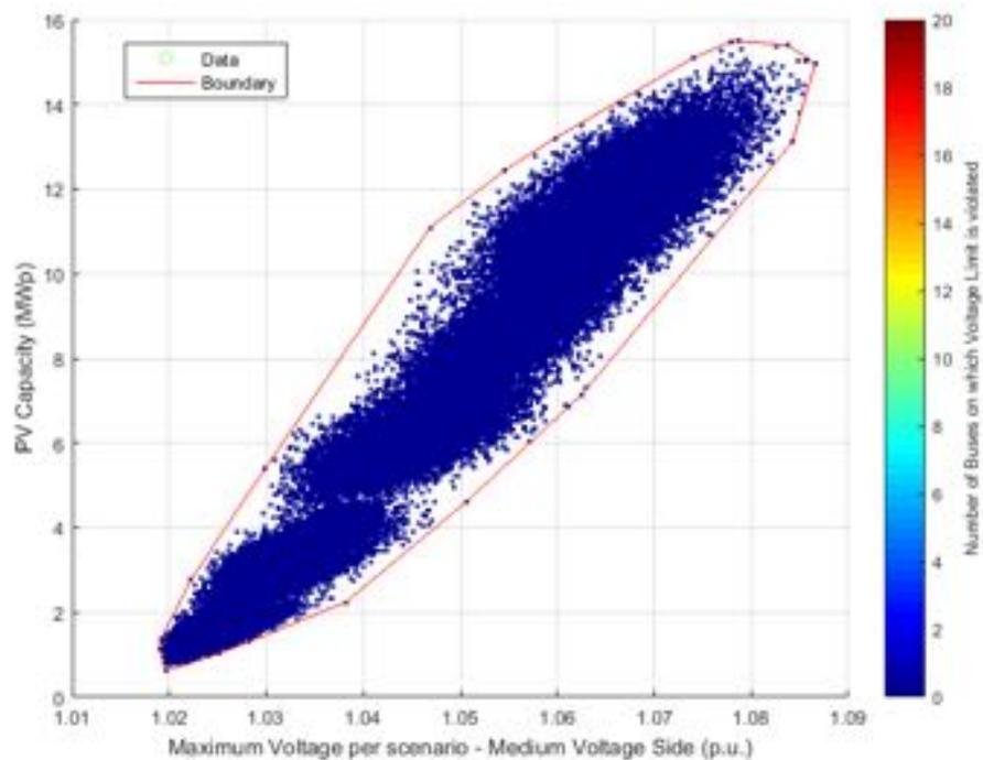
**Figure 112.** PV Capacity against Voltage – Medium voltage side - Power Factor  $\cos\phi(P)$ .
