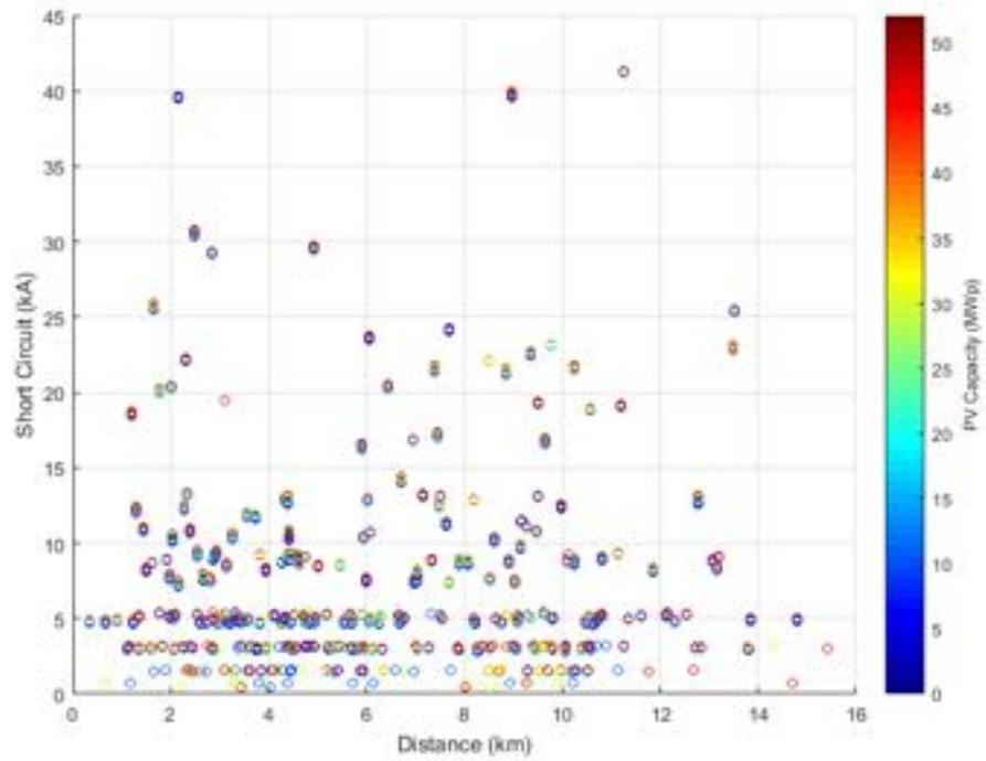
**Figure 321.** Short circuit current against Distance - Power Factor equal to 0.95.
