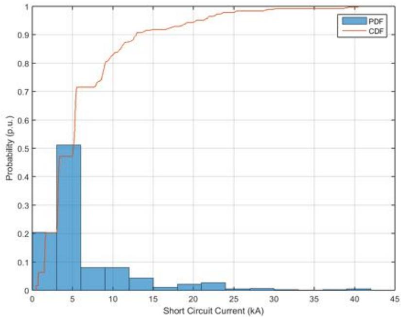
**Figure 283.** Probability distribution and cumulative probability distribution – Short Circuit Current – Unity power factor.
