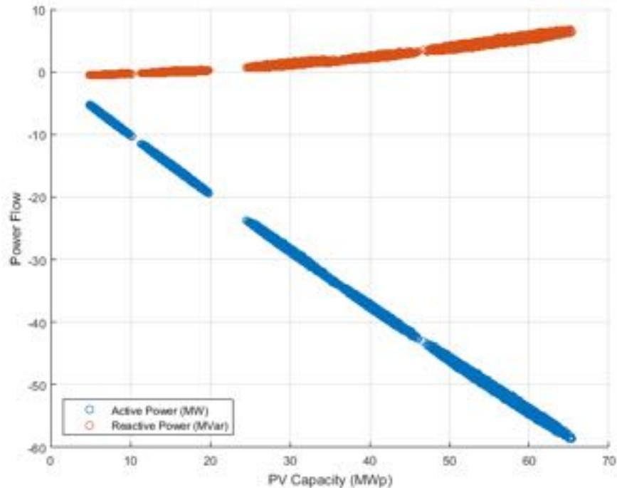
**Figure 259.** Power flow at PCC (connection of the reference substation with HV network) against PV capacity - Unity Power Factor (negative sign denotes reverse power flow).
