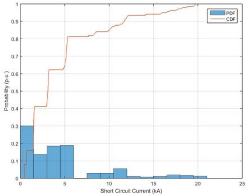
**Figure 81.** Probability distribution and cumulative probability distribution – Short Circuit Current – Power Factor  $\cos\phi(P)$ .
