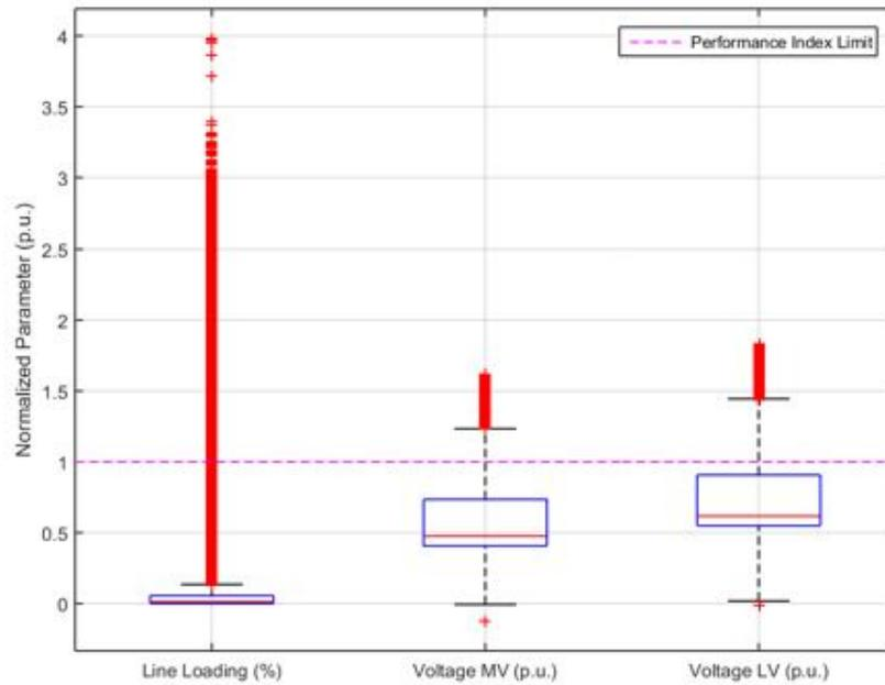
**Figure 130.** Performance Index parameters normalized to their limit – Power Factor  $\cos\phi(P)$ .
