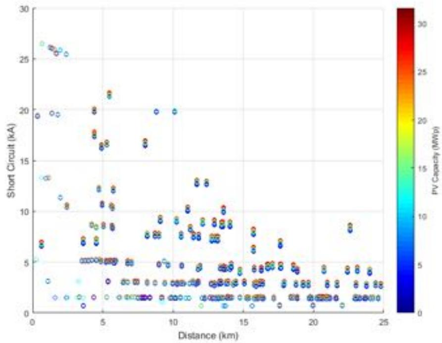
**Figure 162.** Short circuit current against Distance - Power Factor equal to 0.95.
