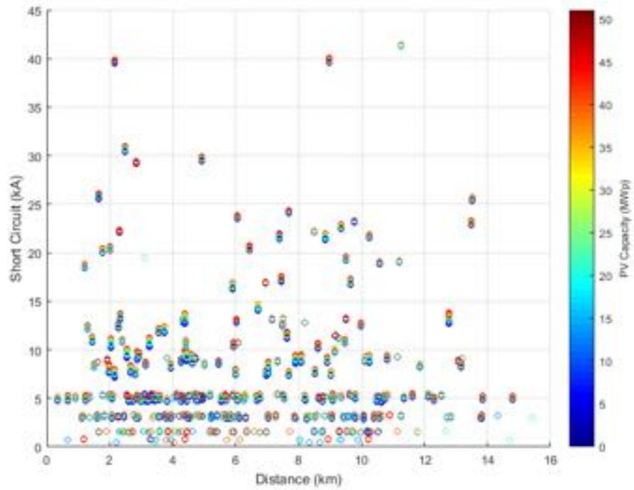
**Figure 313.** Short circuit current against distance - Unity Power Factor.
