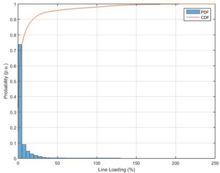
**Figure 80.** Probability distribution and cumulative probability distribution – Line Loading – Power Factor  $\cos\phi(P)$ .
