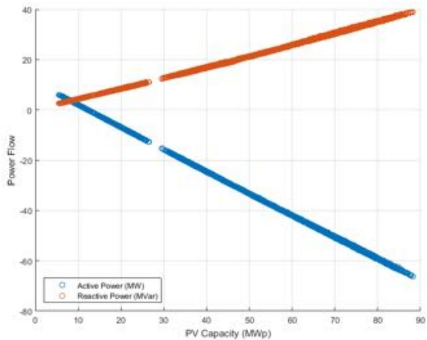
**Figure 63.** Power flow at PCC (connection of the reference substation with HV network) vs PV Capacity - Power Factor  $\cos\phi(P)$ .
