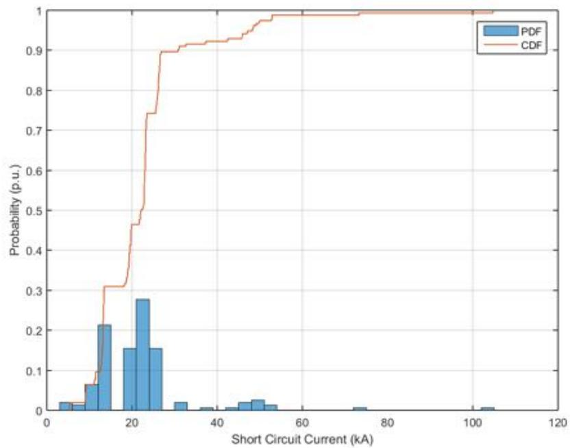
**Figure 200.** Probability distribution and cumulative probability distribution – Short Circuit Current – Power Factor  $\cos\phi(P)$ .
