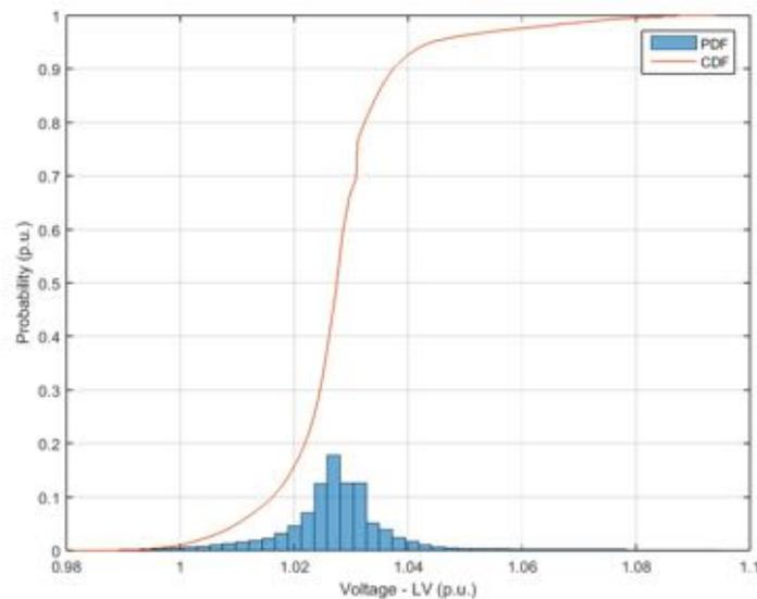
**Figure 20.** Probability distribution and cumulative probability distribution – Voltage at low voltage side – Power Factor equal to 0.95.
