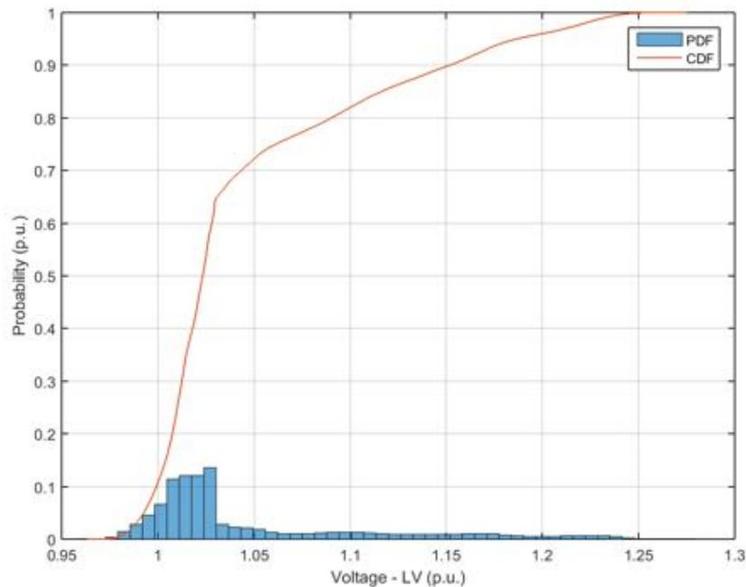
**Figure 126.** Probability distribution and cumulative probability distribution – Voltage at low voltage side – Power Factor equal to 0.95.
