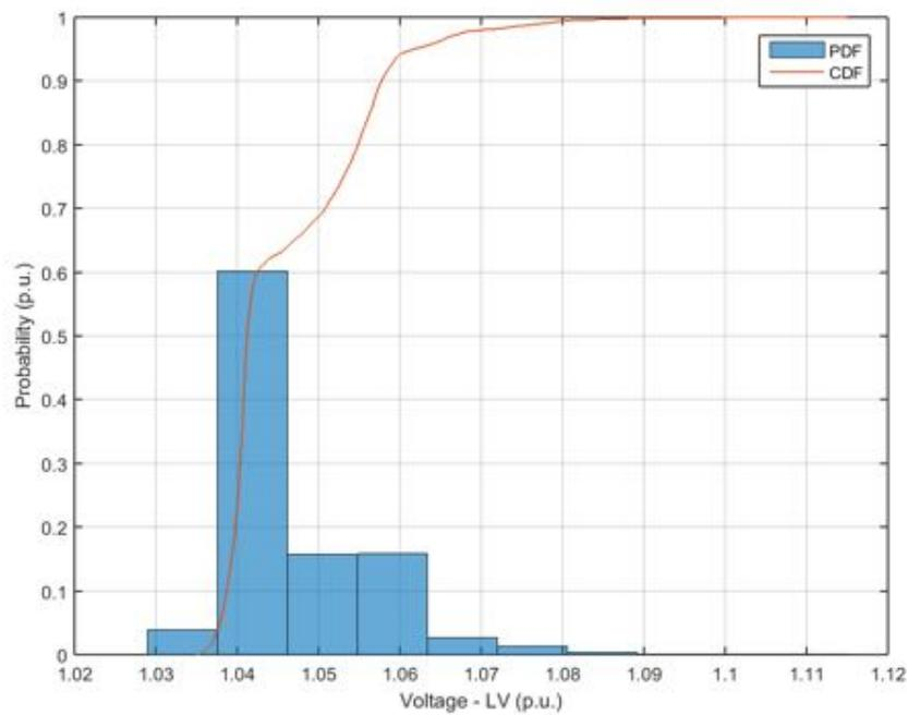
**Figure 243.** Probability distribution and cumulative probability distribution – Voltage at low voltage side – Unity Power Factor.
