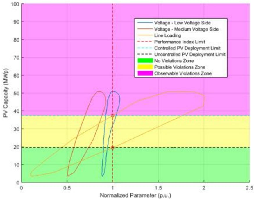
**Figure 318.** Normalized performance index parameters - Power Factor equal to 0.95.
