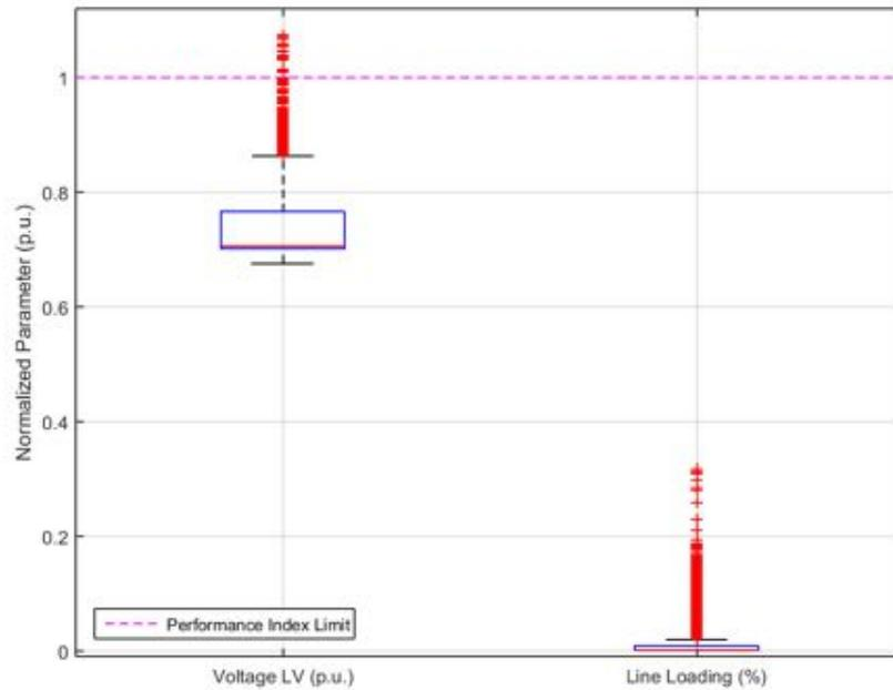
**Figure 242.** Performance Index parameters normalized to their limit – Unity Power Factor.
