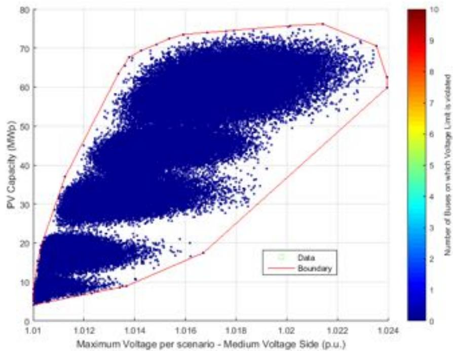
**Figure 218.** PV Capacity against Voltage – Medium voltage side - Power Factor  $\cos\phi(P)$ .
