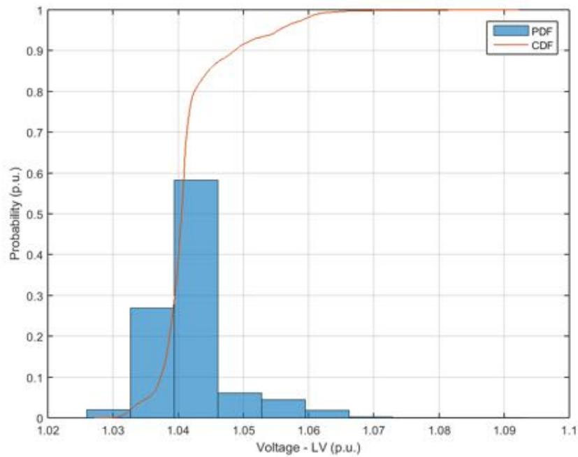
**Figure 251.** Probability distribution and cumulative probability distribution – Voltage at low voltage side – Power Factor  $\cos\phi(P)$ .
