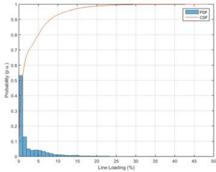
**Figure 40.** Probability distribution and cumulative probability distribution – Line Loading – Power Factor  $\cos\phi(P)$ .
