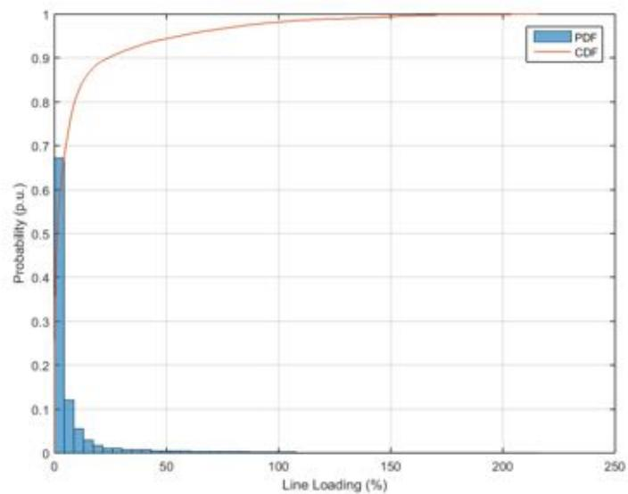
**Figure 27.** Probability distribution and cumulative probability distribution – Line Loading – Power Factor  $\cos\phi(P)$ .
