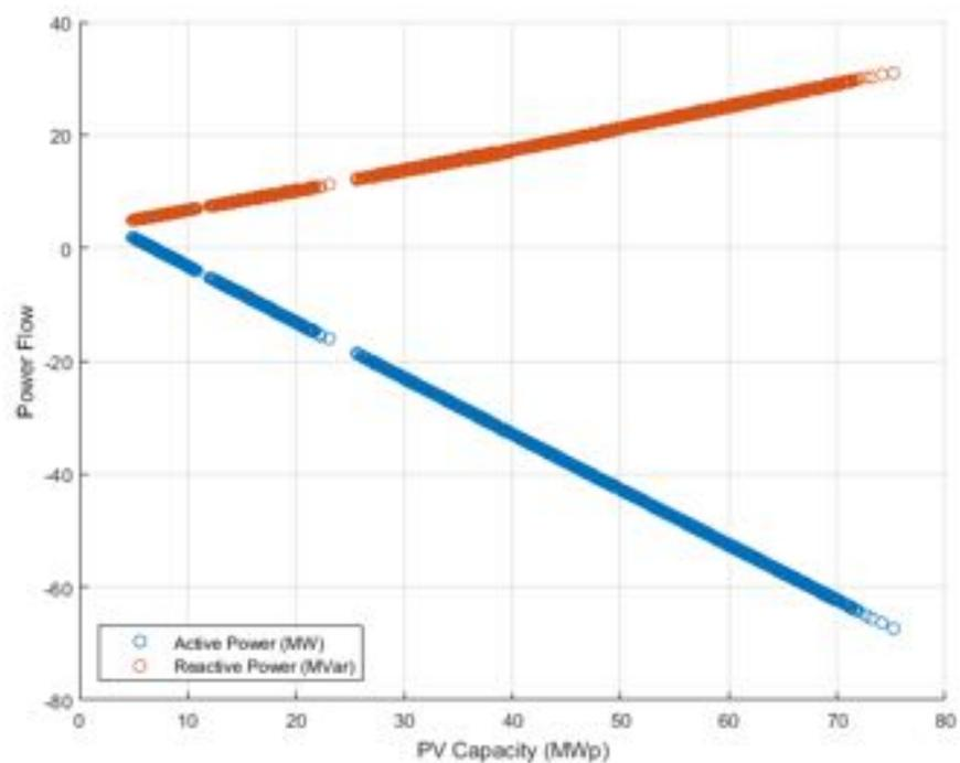
**Figure 214.** Power flow at PCC (connection of the reference substation with HV network) vs PV Capacity - Power Factor equal to 0.95.
