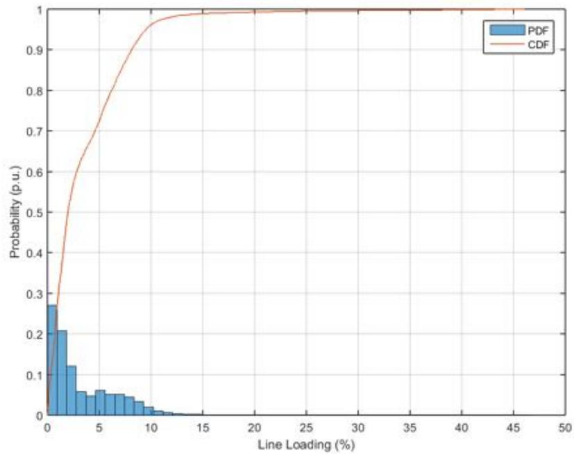
**Figure 199.** Probability distribution and cumulative probability distribution – Line Loading – Power Factor  $\cos\phi(P)$ .
