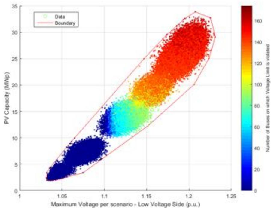
**Figure 156.** PV Capacity against Voltage – Low voltage side - Power Factor equal to 0.95.
