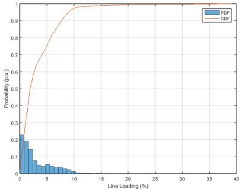
**Figure 191.** Probability distribution and cumulative probability distribution – Line Loading – Unity Power Factor.
