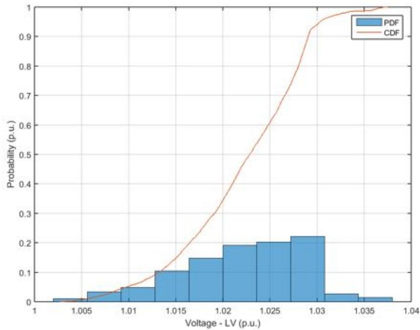
**Figure 304.** Probability distribution and cumulative probability distribution – Voltage at low voltage side – Power Factor  $\cos\phi(P)$ .
