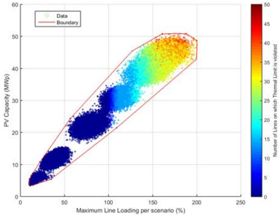
**Figure 317.** PV Capacity against Line Loading - Power Factor equal to 0.95.
