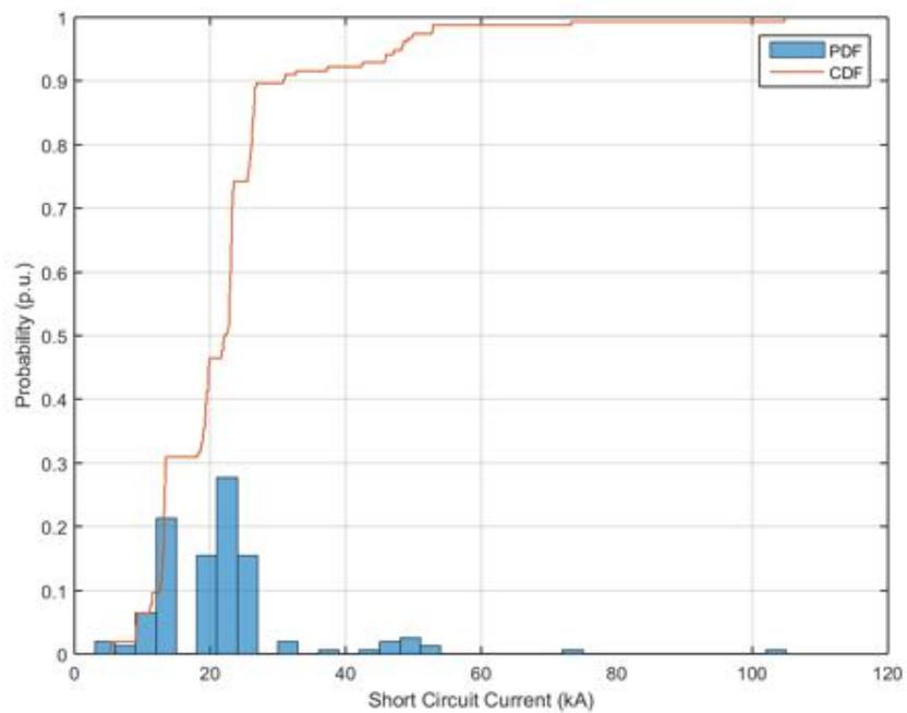
**Figure 196.** Probability distribution and cumulative probability distribution – Short Circuit Current – Power Factor equal to 0.95.
