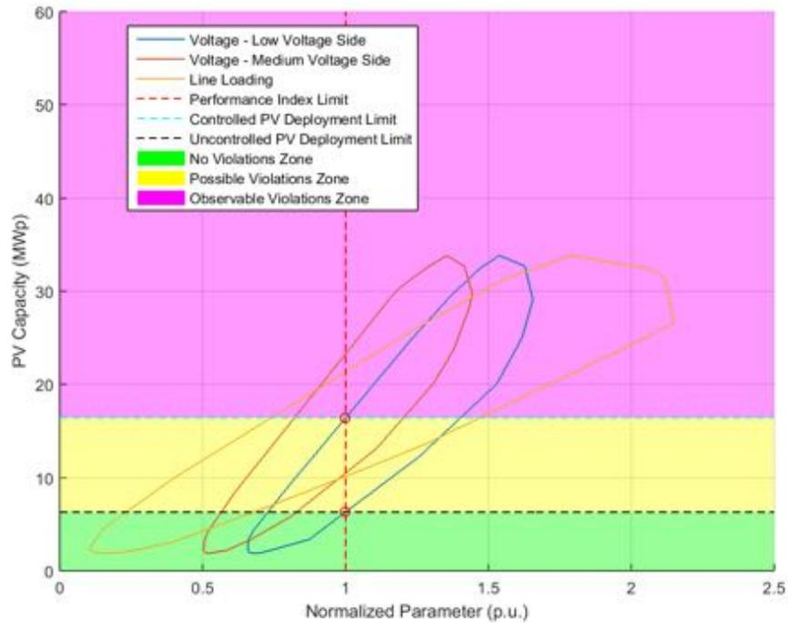
**Figure 159.** Normalized performance index parameters - Power Factor equal to 0.95.
