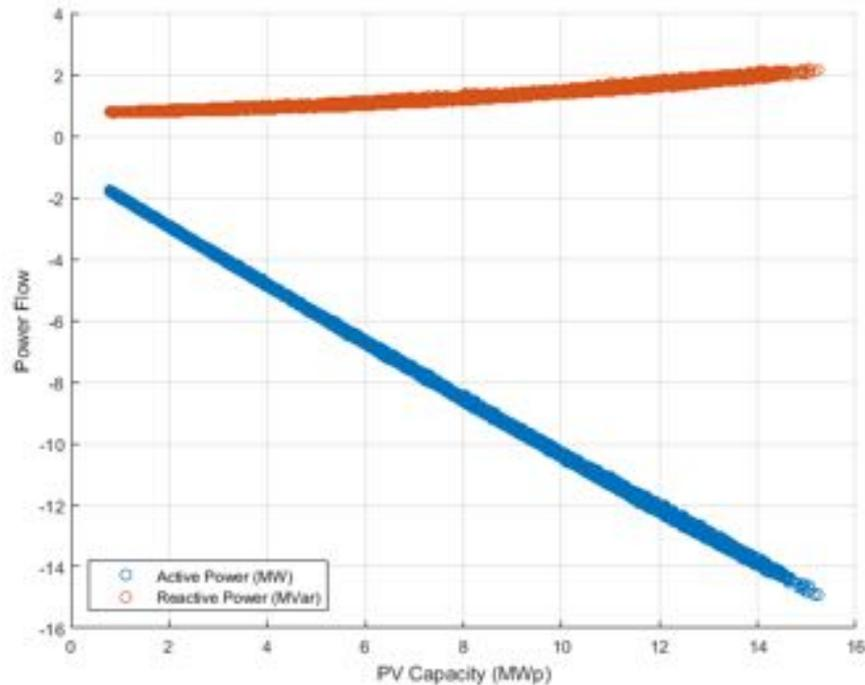
**Figure 100.** Power flow at PCC (connection of the reference substation with HV network) against PV capacity - Unity Power Factor (negative sign denotes reverse power flow).
