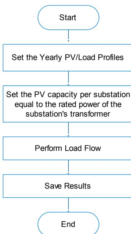
**Figure 4.** Flowchart of maximum installed PV capacity scenario.
