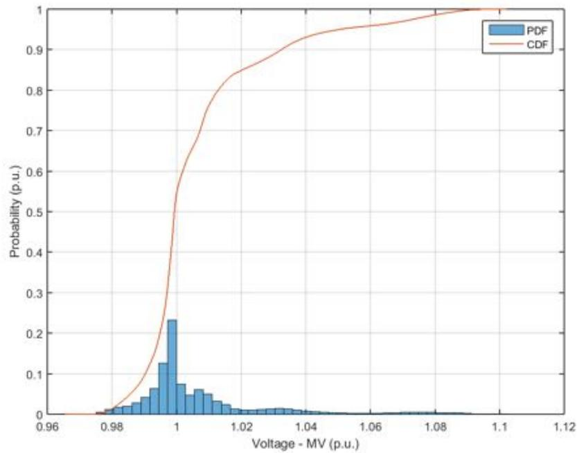
**Figure 79.** Probability distribution and cumulative probability distribution – Voltage at medium voltage side – Power Factor  $\cos\phi(P)$ .
