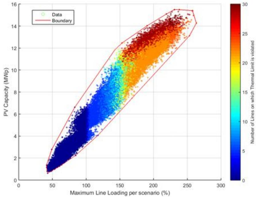
**Figure 113.** PV Capacity against Line Loading - Power Factor  $\cos\phi(P)$ .
