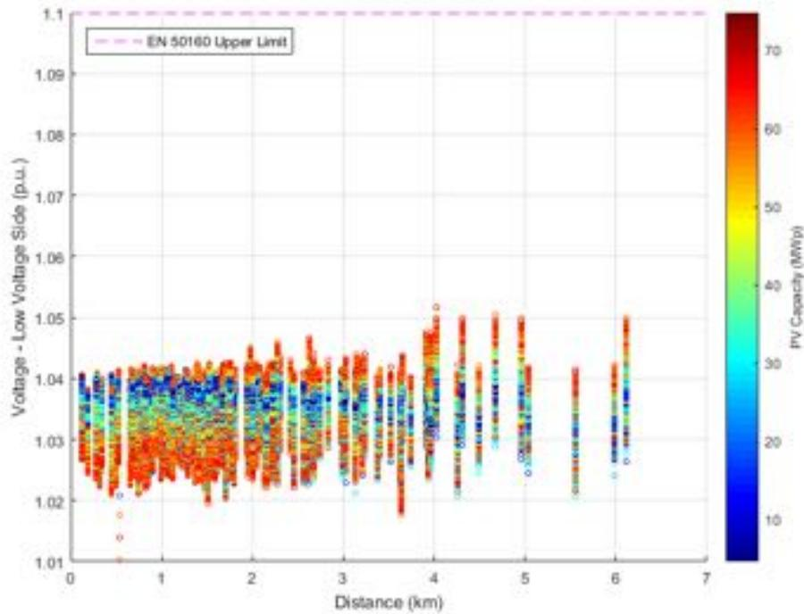
**Figure 221.** Voltage at low voltage side against distance from transmission substation - Power Factor  $\cos\phi(P)$ .
