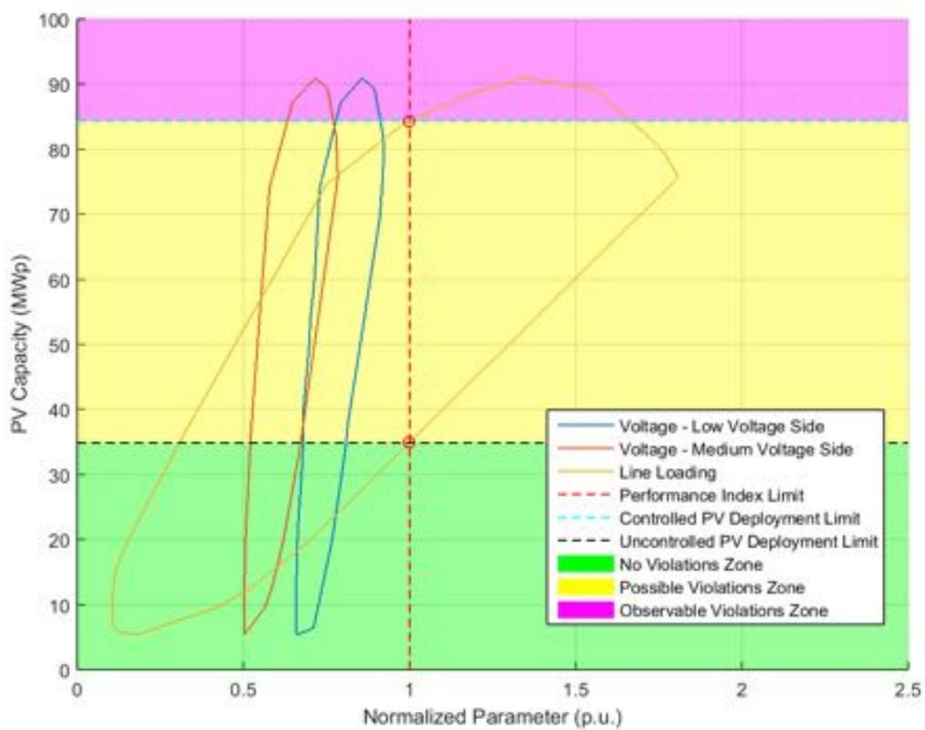
**Figure 53.** Normalized performance index parameters - Power Factor equal to 0.95.
