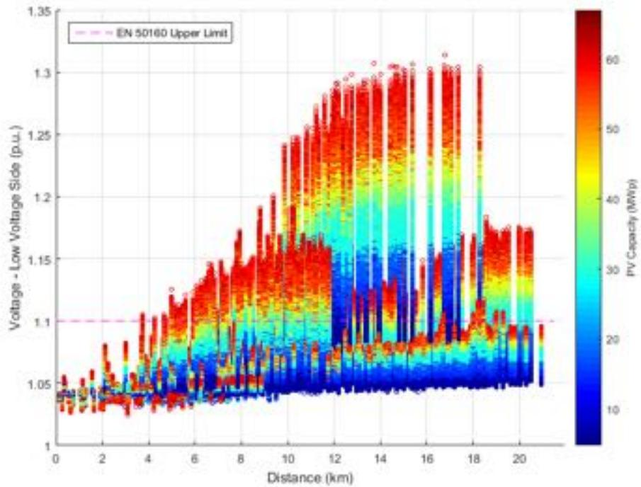
**Figure 274.** Voltage at low voltage side against distance from transmission substation - Power Factor  $\cos\phi(P)$ .
