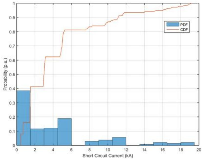
**Figure 82.** Probability distribution and cumulative probability distribution – Short Circuit Current – No PV.
