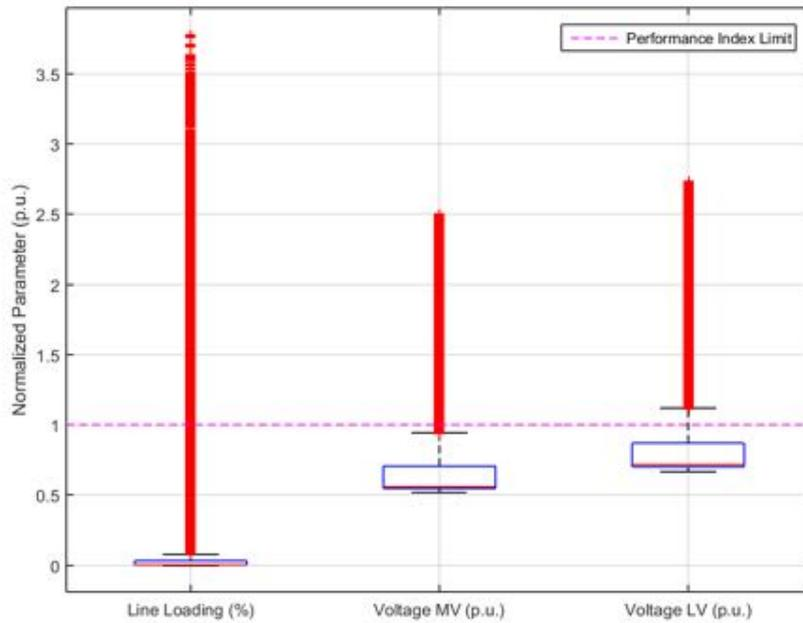
**Figure 231.** Performance Index parameters normalized to their limit – Power Factor equal to 0.95.
