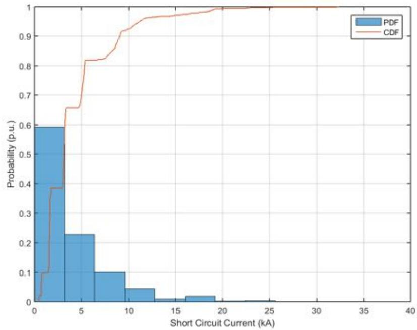
**Figure 240.** Probability distribution and cumulative probability distribution – Short Circuit Current – Power Factor  $\cos\phi(P)$ .
