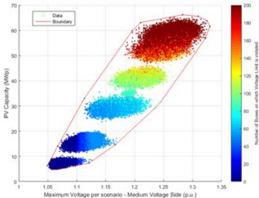
**Figure 263.** PV Capacity against Voltage – Medium voltage side - Power Factor equal to 0.95.
