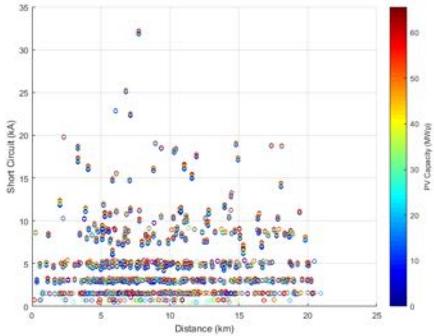
**Figure 268.** Short circuit current against Distance - Power Factor equal to 0.95.
