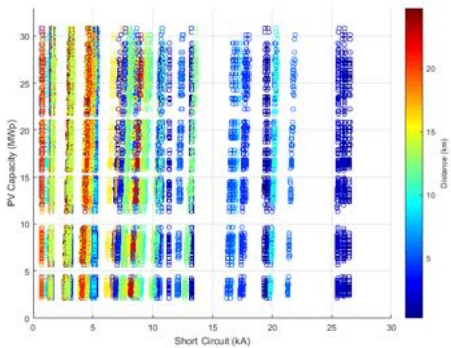
**Figure 155.** PV Capacity against Short circuit current - Unity Power Factor
