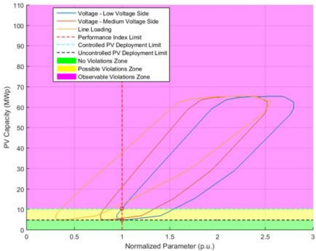
**Figure 257.** Normalized performance index parameters - Unity Power Factor.
