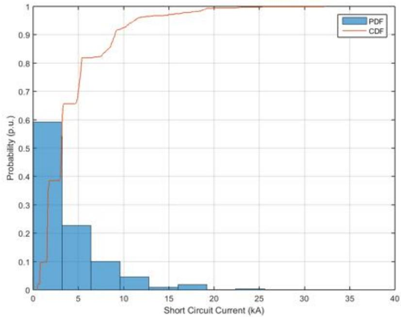
**Figure 235.** Probability distribution and cumulative probability distribution – Short Circuit Current – Power Factor equal to 0.95.
