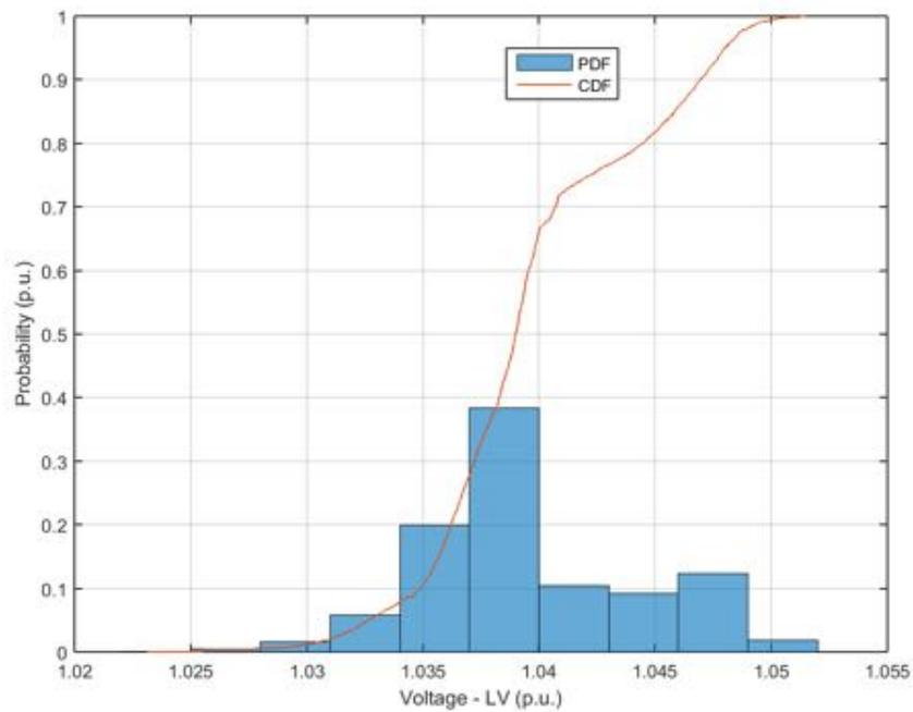
**Figure 190.** Probability distribution and cumulative probability distribution – Voltage at low voltage side – Unity Power Factor.
