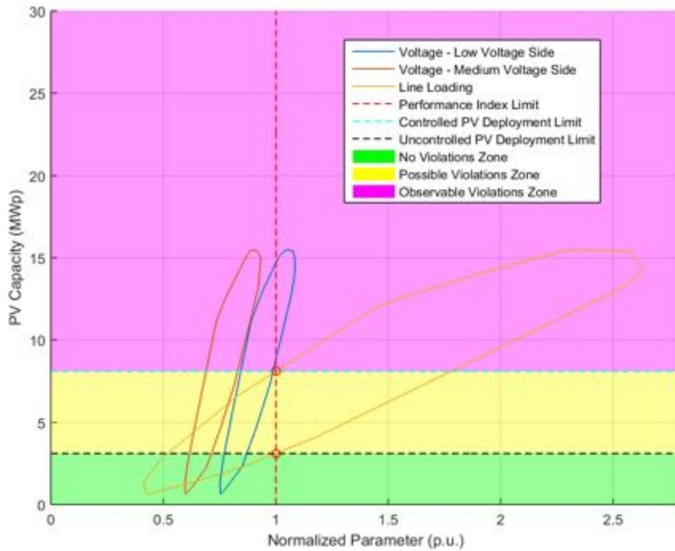
**Figure 114.** Normalized performance index parameters - Power Factor  $\cos\phi(P)$ .
