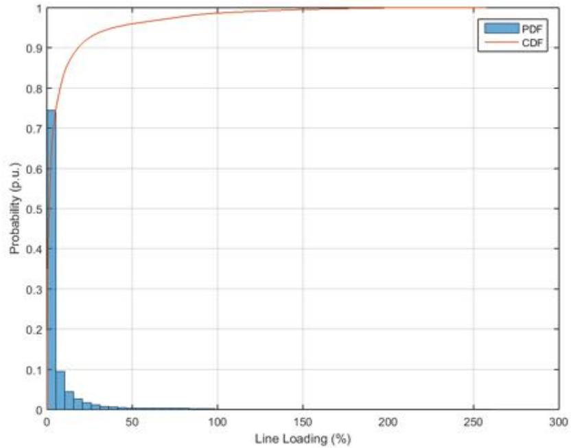
**Figure 123.** Probability distribution and cumulative probability distribution – Line Loading – Unity power factor.
