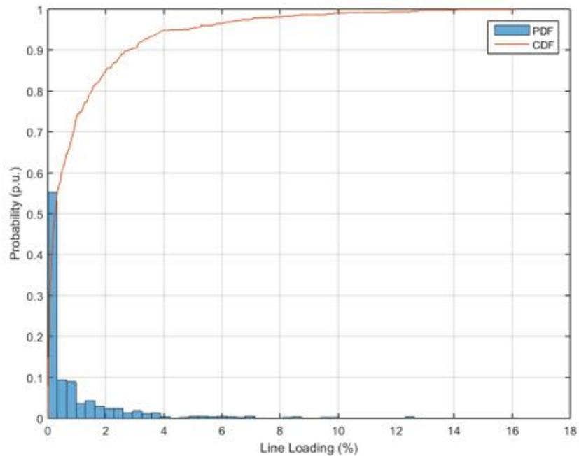
**Figure 138.** Probability distribution and cumulative probability distribution – Line Loading – Unity Power Factor.
