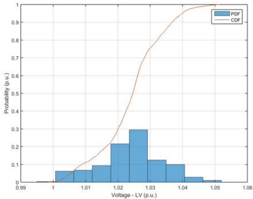
**Figure 84.** Probability distribution and cumulative probability distribution – Voltage at low voltage side – Unity Power Factor.
