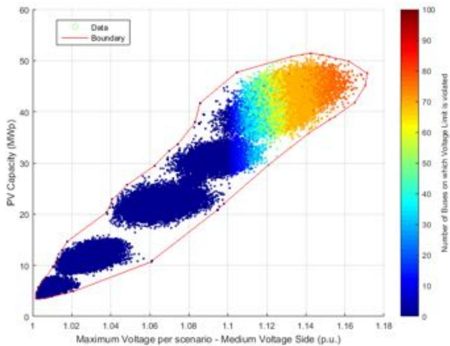
**Figure 308.** PV Capacity against Voltage – Medium voltage side - Unity Power Factor.
