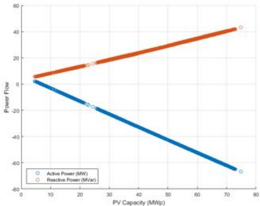
**Figure 222.** Power flow at PCC (connection of the reference substation with HV network) vs PV Capacity - Power Factor  $\cos\phi(P)$ .
