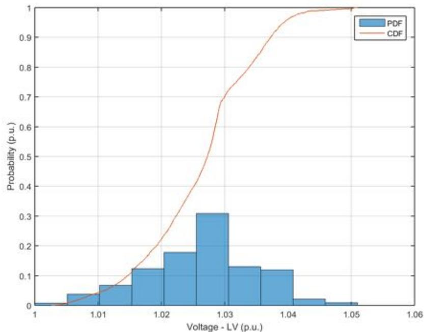
**Figure 296.** Probability distribution and cumulative probability distribution – Voltage at low voltage side – Unity Power Factor.
