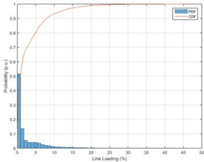
**Figure 36.** Probability distribution and cumulative probability distribution – Line Loading – Power Factor equal to 0.95.
