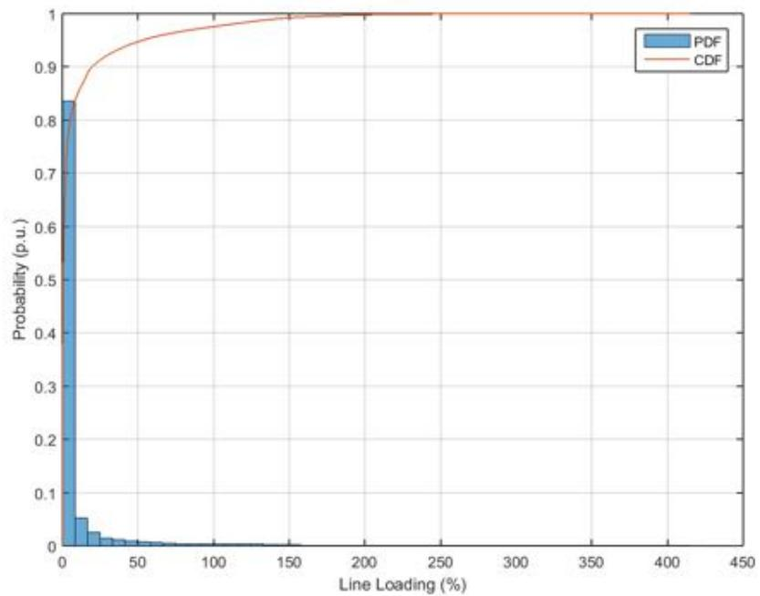
**Figure 239.** Probability distribution and cumulative probability distribution – Line Loading – Power Factor  $\cos\phi(P)$ .
