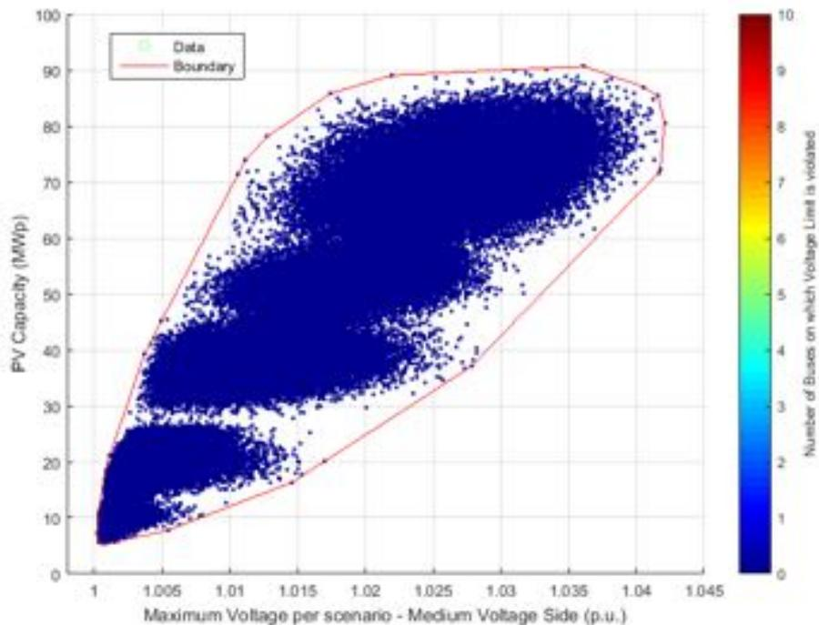
**Figure 59.** PV Capacity against Voltage – Medium voltage side - Power Factor  $\cos\phi(P)$ .
