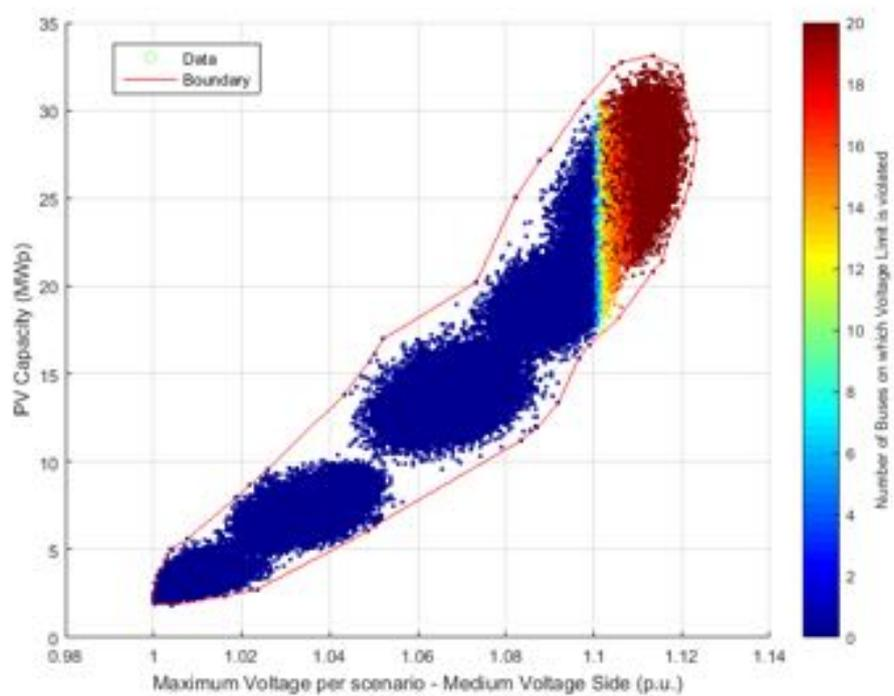
**Figure 165.** PV Capacity against Voltage – Medium voltage side - Power Factor  $\cos\phi(P)$ .
