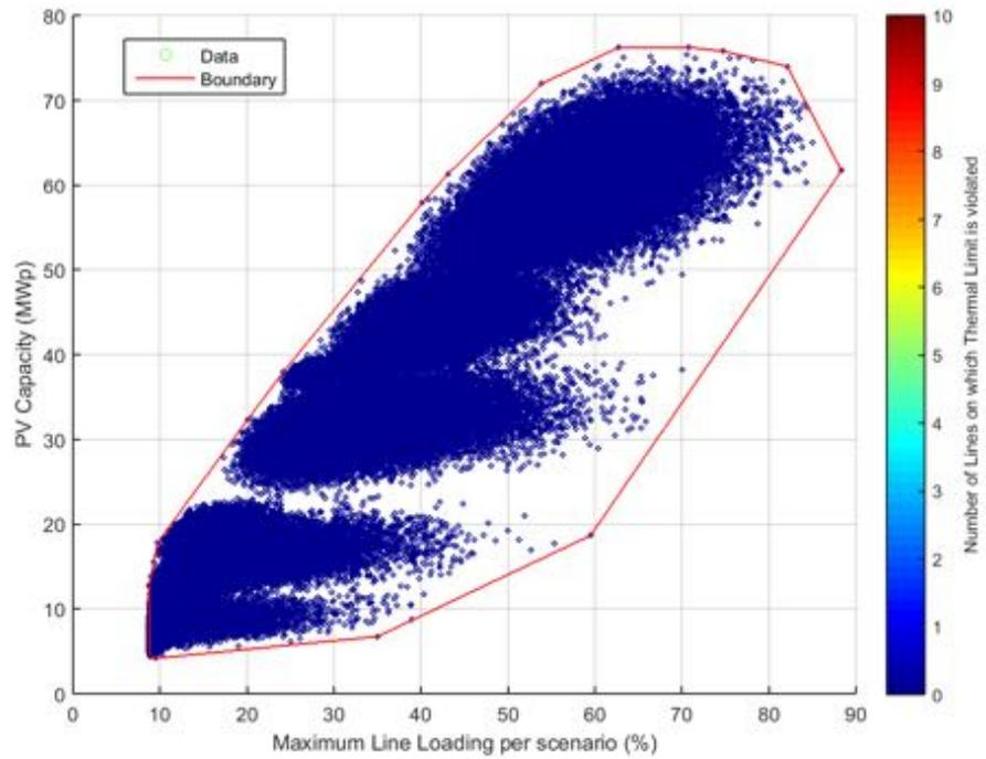
**Figure 203.** PV Capacity against Line Loading - Unity Power Factor.
