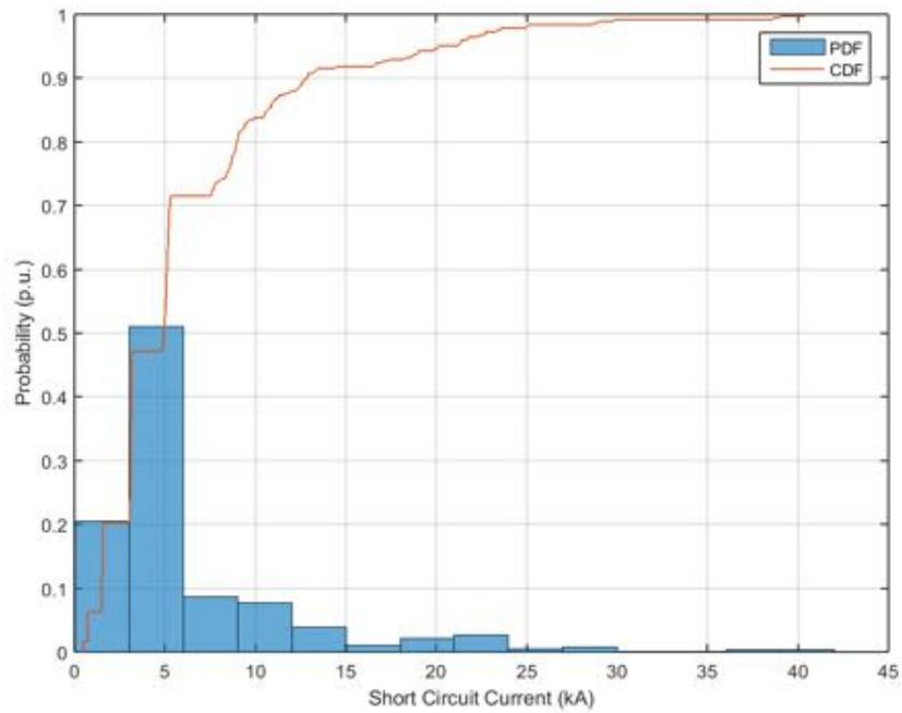
**Figure 293.** Probability distribution and cumulative probability distribution – Short Circuit Current – Power Factor  $\cos\phi(P)$ .
