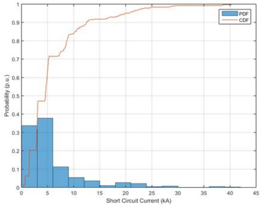
**Figure 294.** Probability distribution and cumulative probability distribution – Short Circuit Current – No PV.
