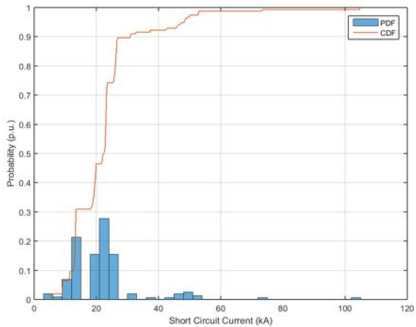
**Figure 177.** Probability distribution and cumulative probability distribution – Short Circuit Current – Unity power factor.
