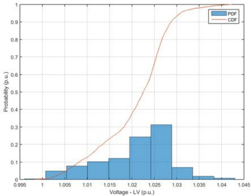
**Figure 88.** Probability distribution and cumulative probability distribution – Voltage at low voltage side – Power Factor equal to 0.95.
