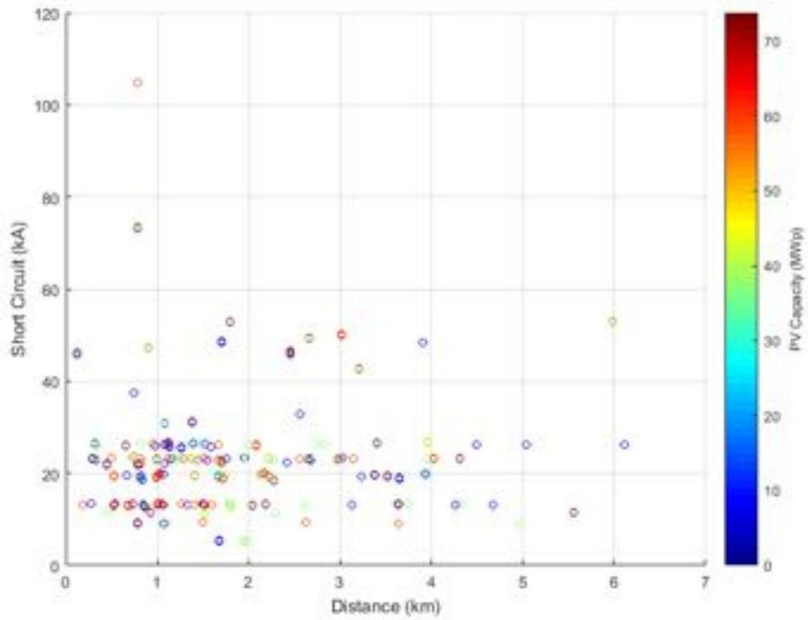
**Figure 207.** Short circuit current against distance - Unity Power Factor.
