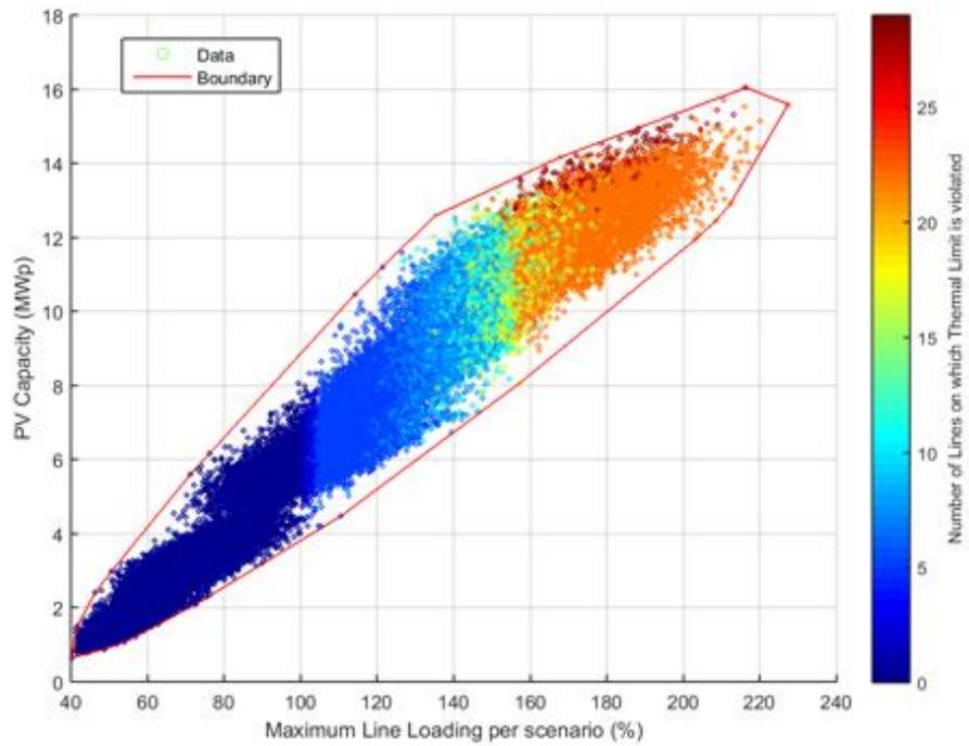
**Figure 97.** PV Capacity against Line Loading - Unity Power Factor.
