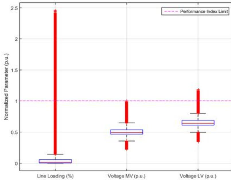
**Figure 284.** Performance Index parameters normalized to their limit – Power Factor equal to 0.95.
