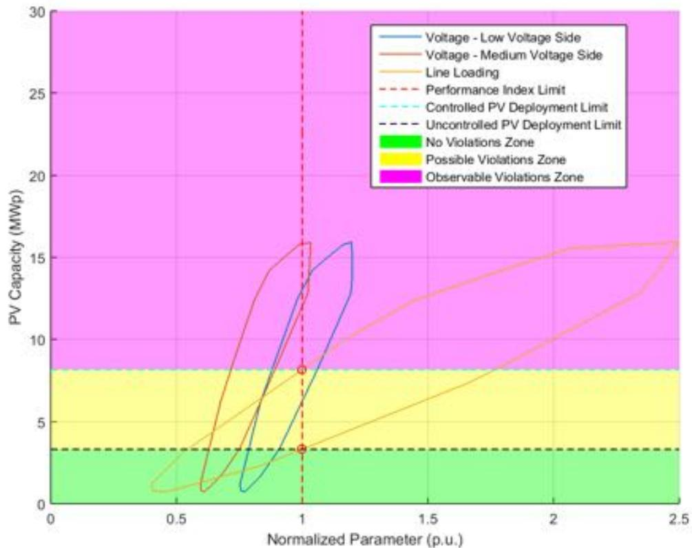
**Figure 106.** Normalized performance index parameters - Power Factor equal to 0.95.
