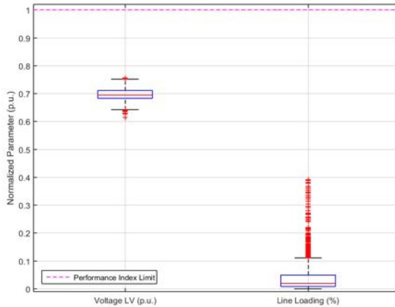
**Figure 189.** Performance Index parameters normalized to their limit – Unity Power Factor.
