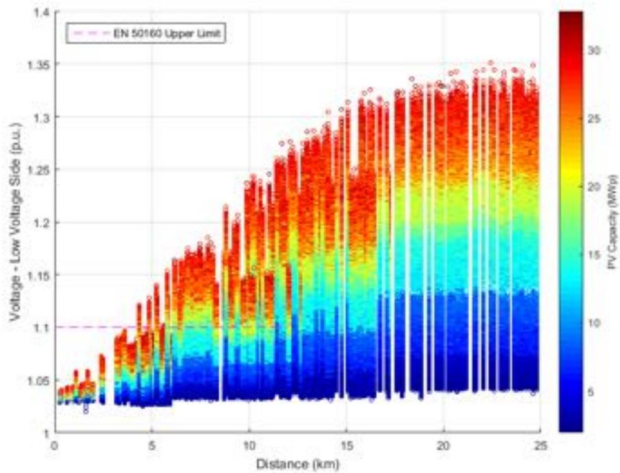
**Figure 152.** Voltage at low voltage side against distance from transmission substation - Unity Power Factor.
