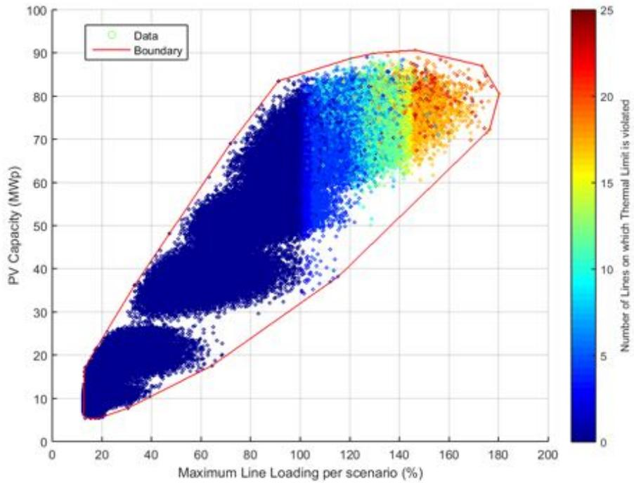
**Figure 60.** PV Capacity against Line Loading - Power Factor  $\cos\phi(P)$ .
