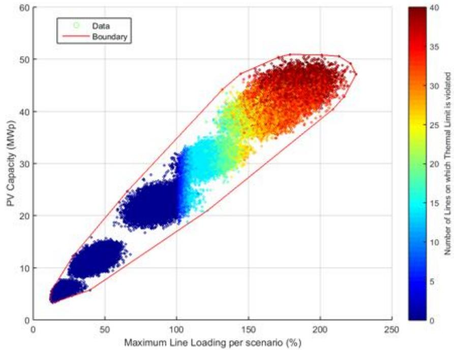
**Figure 325.** PV Capacity against Line Loading - Power Factor  $\cos\phi(P)$ .
