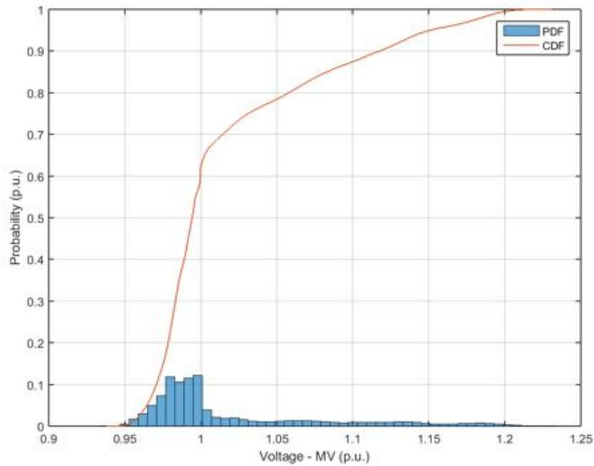
**Figure 127.** Probability distribution and cumulative probability distribution – Voltage at medium voltage side – Power Factor equal to 0.95.
