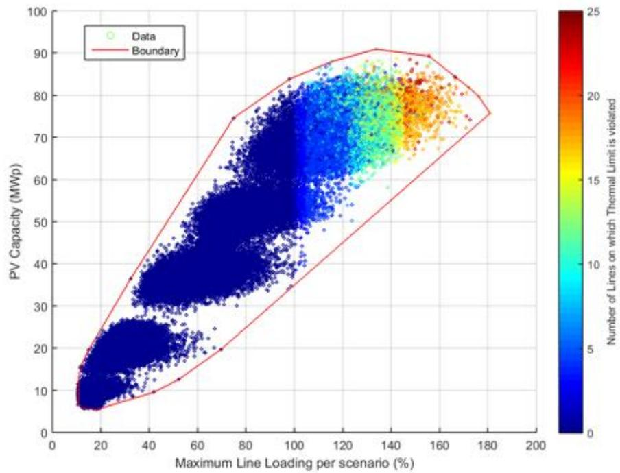
**Figure 52.** PV Capacity against Line Loading - Power Factor equal to 0.95.
