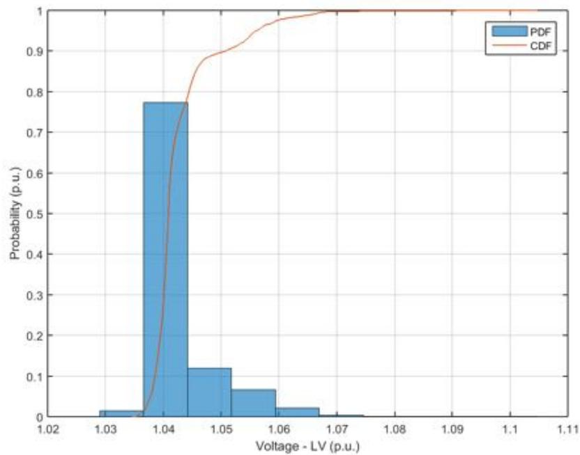
**Figure 247.** Probability distribution and cumulative probability distribution – Voltage at low voltage side – Power Factor equal to 0.95.
