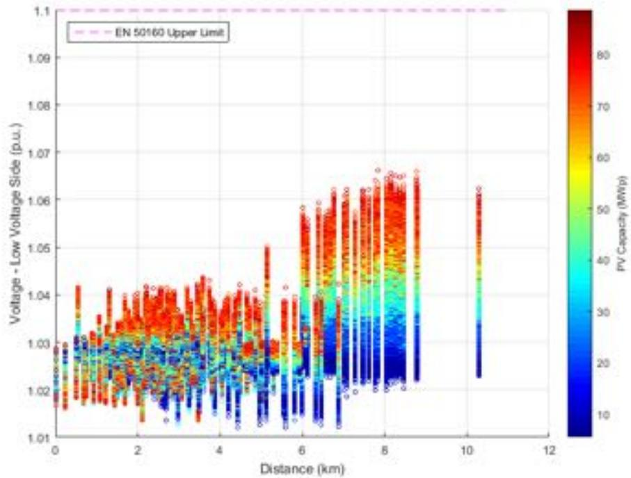
**Figure 62.** Voltage at low voltage side against distance from transmission substation - Power Factor  $\cos\phi(P)$ .
