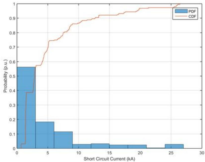
**Figure 147.** Probability distribution and cumulative probability distribution – Short Circuit Current – Power Factor  $\cos\phi(P)$ .
