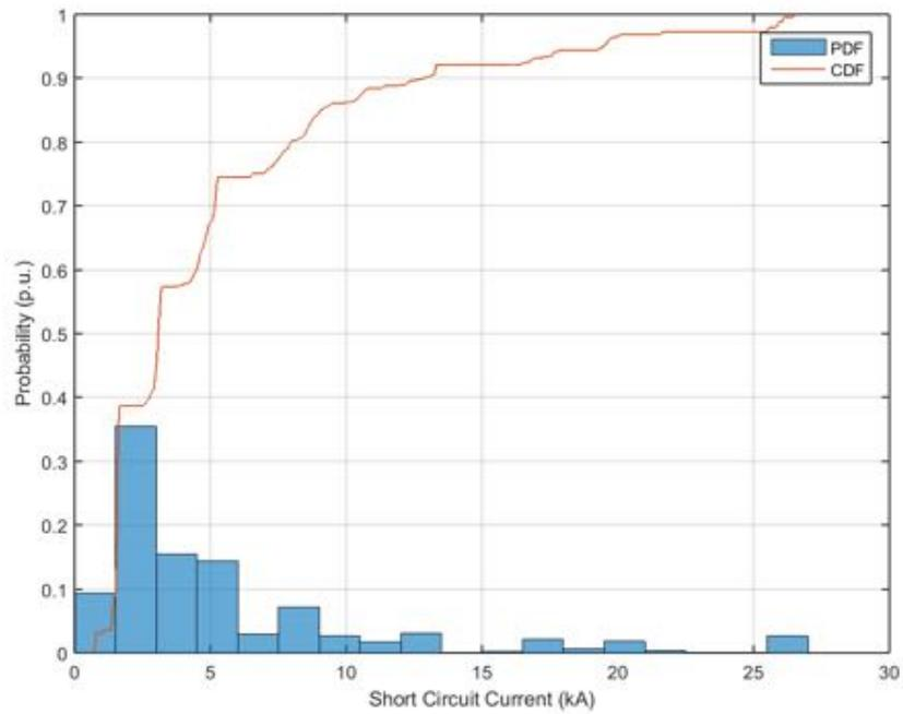
**Figure 134.** Probability distribution and cumulative probability distribution – Short Circuit Current – Power Factor  $\cos\phi(P)$ .
