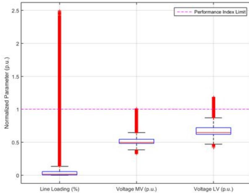
**Figure 77.** Performance Index parameters normalized to their limit – Power Factor  $\cos\phi(P)$ .
