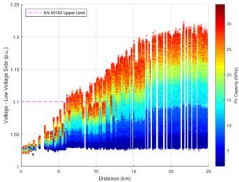
**Figure 160.** Voltage at low voltage side against Distance from transmission substation - Power Factor equal to 0.95.
