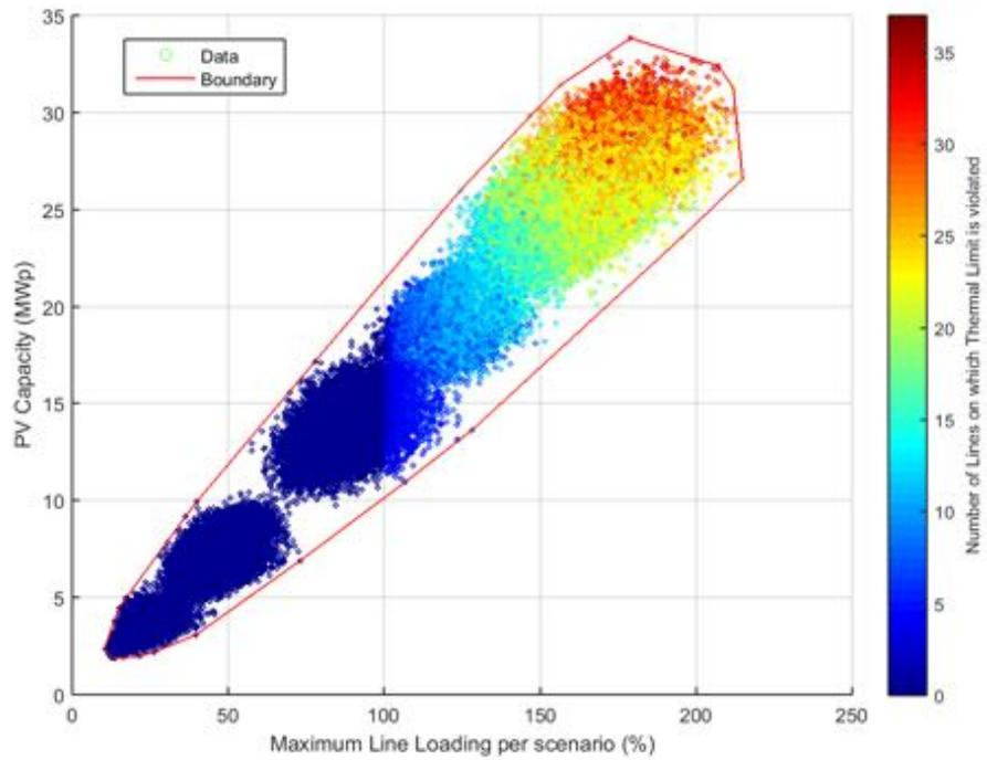
**Figure 158.** PV Capacity against Line Loading - Power Factor equal to 0.95.
