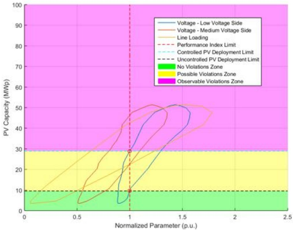
**Figure 310.** Normalized performance index parameters - Unity Power Factor.
