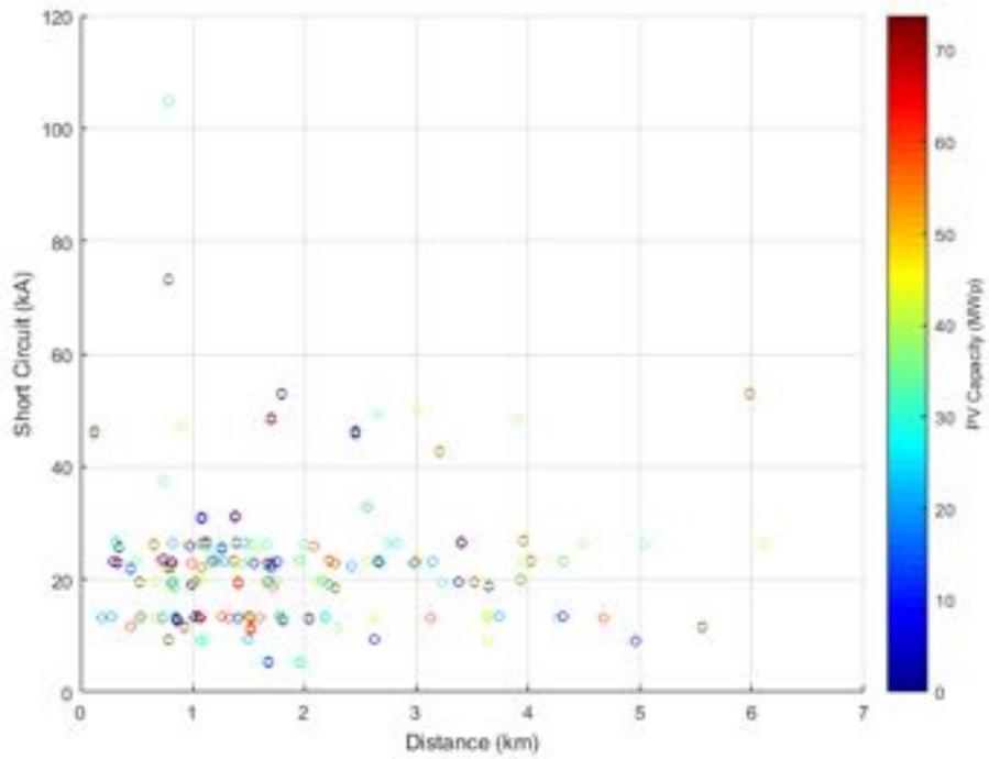
**Figure 215.** Short circuit current against Distance - Power Factor equal to 0.95.
