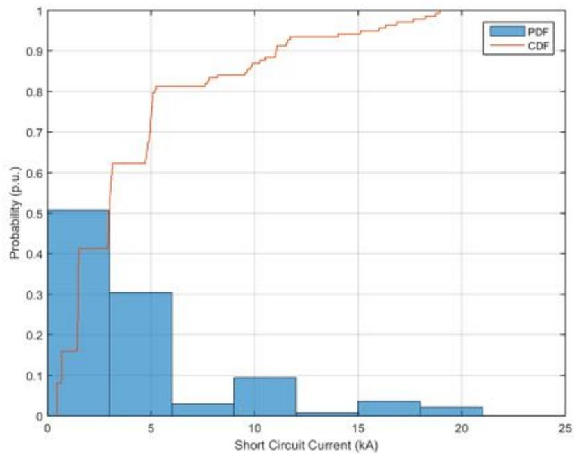
**Figure 94.** Probability distribution and cumulative probability distribution – Short Circuit Current – Power Factor  $\cos\phi(P)$ .
