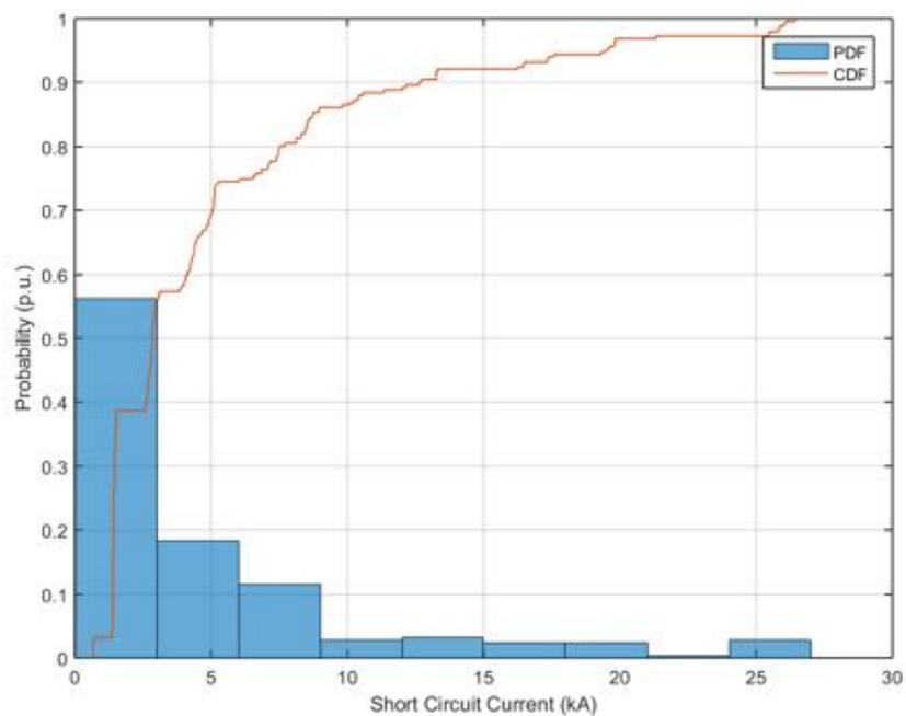
**Figure 139.** Probability distribution and cumulative probability distribution – Short Circuit Current – Unity Power Factor.
