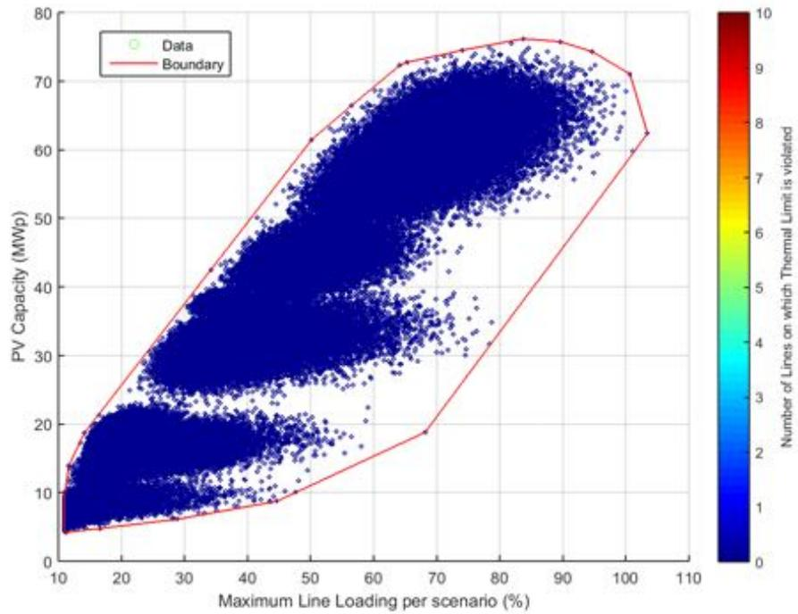
**Figure 219.** PV Capacity against Line Loading - Power Factor  $\cos\phi(P)$ .
