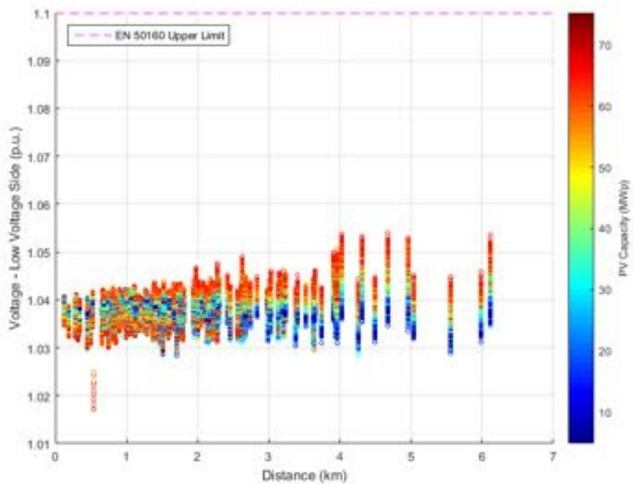
**Figure 213.** Voltage at low voltage side against Distance from transmission substation - Power Factor equal to 0.95.
