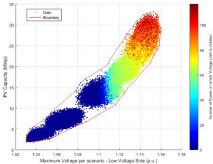
**Figure 164.** PV Capacity against Voltage – Low voltage side - Power Factor  $\cos\phi(P)$ .
