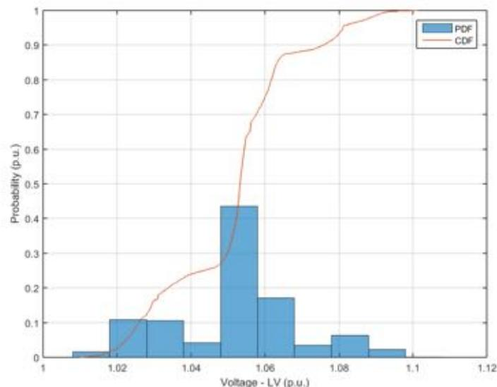
**Figure 31.** Probability distribution and cumulative probability distribution – Voltage at low voltage side – Unity Power Factor.
