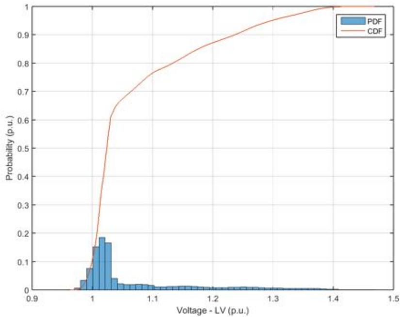
**Figure 121.** Probability distribution and cumulative probability distribution – Voltage at low voltage side – Unity power factor.
