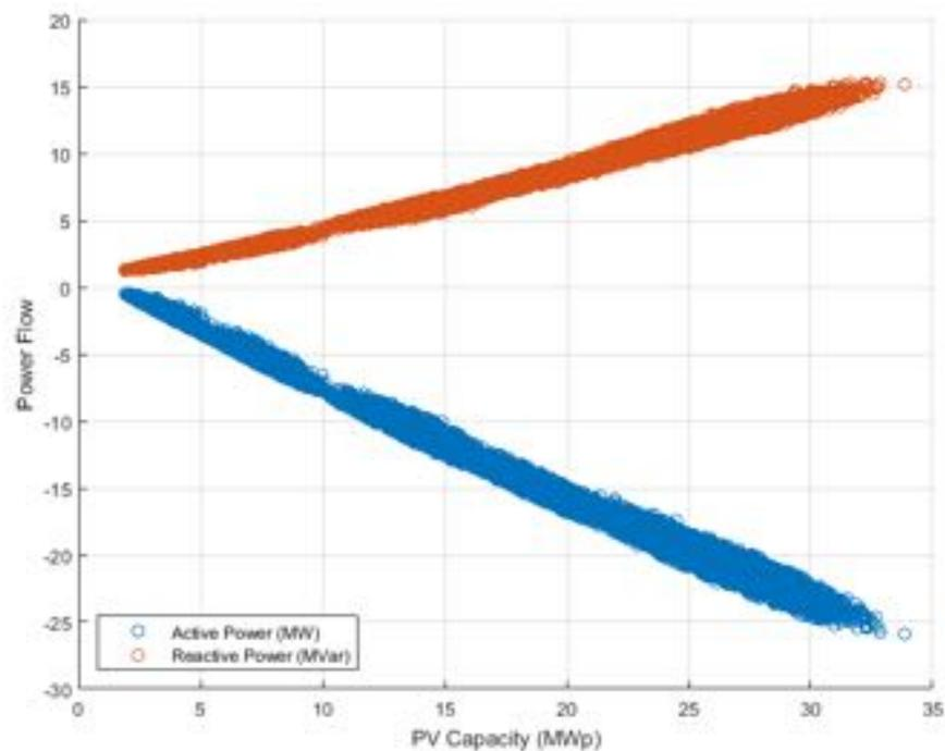
**Figure 161.** Power flow at PCC (connection of the reference substation with HV network) vs PV Capacity - Power Factor equal to 0.95.
