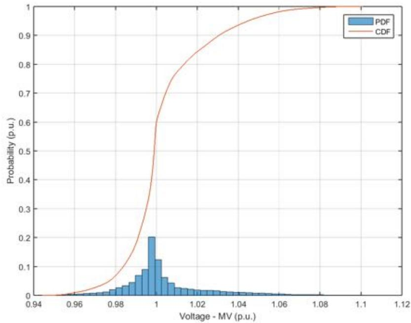
**Figure 286.** Probability distribution and cumulative probability distribution – Voltage at medium voltage side – Power Factor equal to 0.95.
