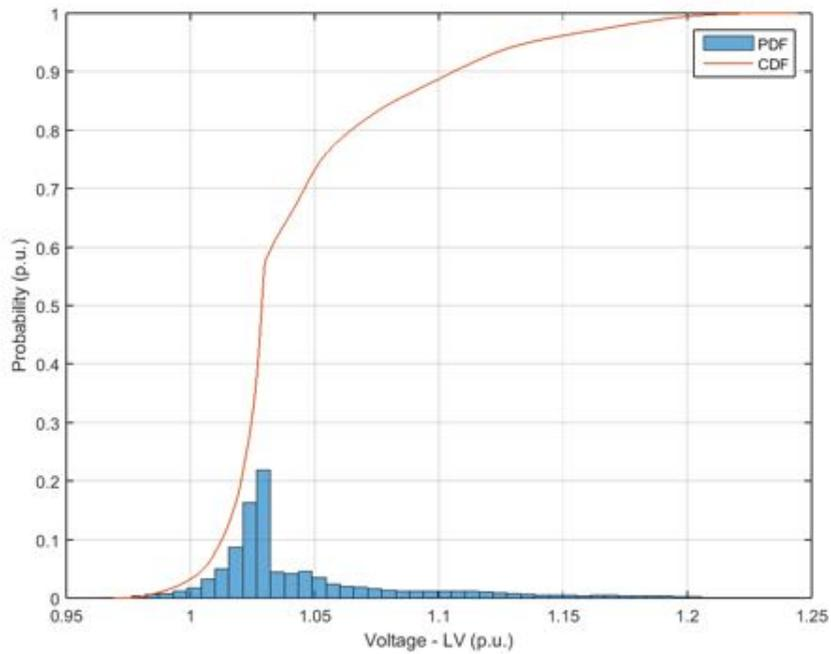
**Figure 280.** Probability distribution and cumulative probability distribution – Voltage at low voltage side – Unity power factor.
