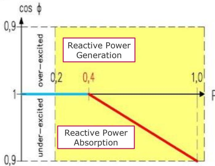
Figure 13. Characteristic curve  $\cos\phi (P)$  of power factor in relation to the generated power.
