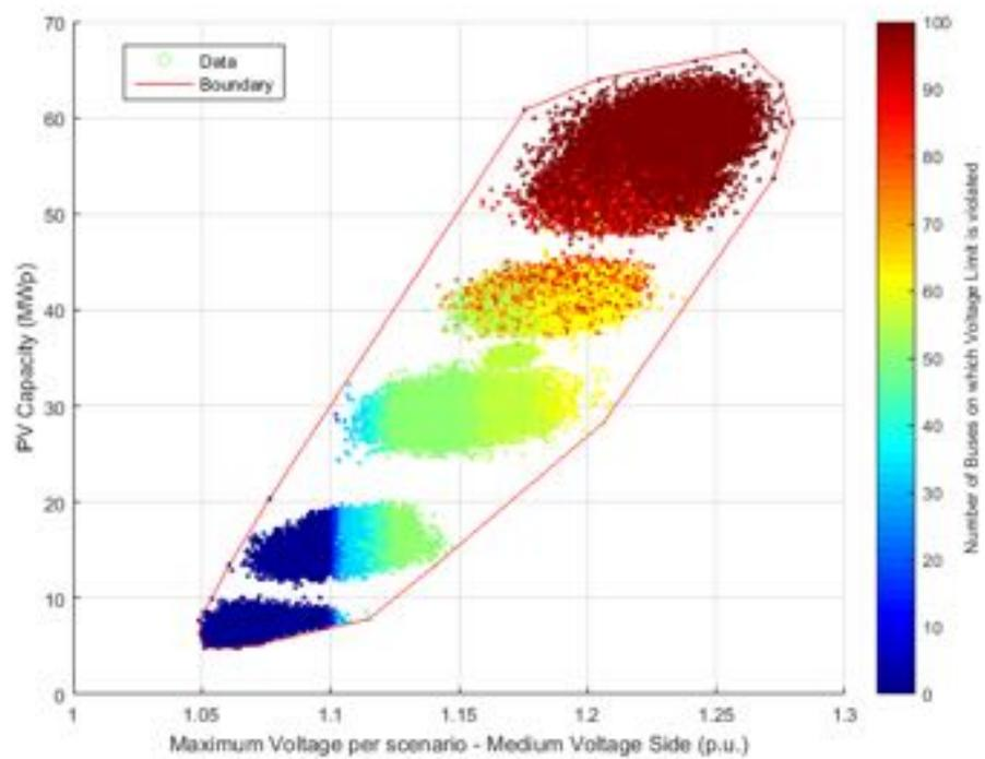
**Figure 271.** PV Capacity against Voltage – Medium voltage side - Power Factor  $\cos\phi(P)$ .
