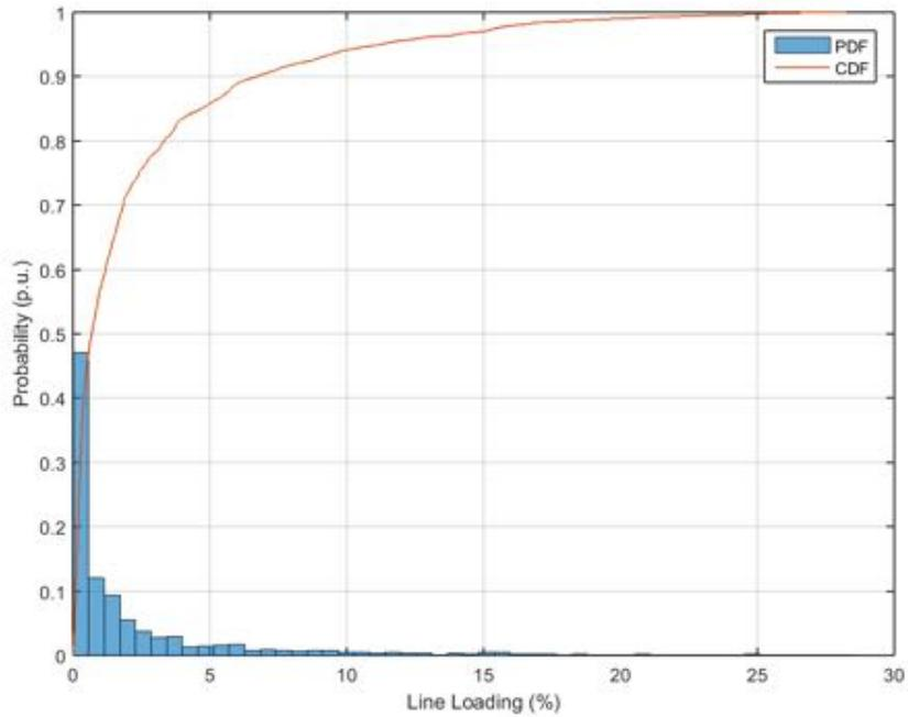
**Figure 301.** Probability distribution and cumulative probability distribution – Line Loading – Power Factor equal to 0.95.
