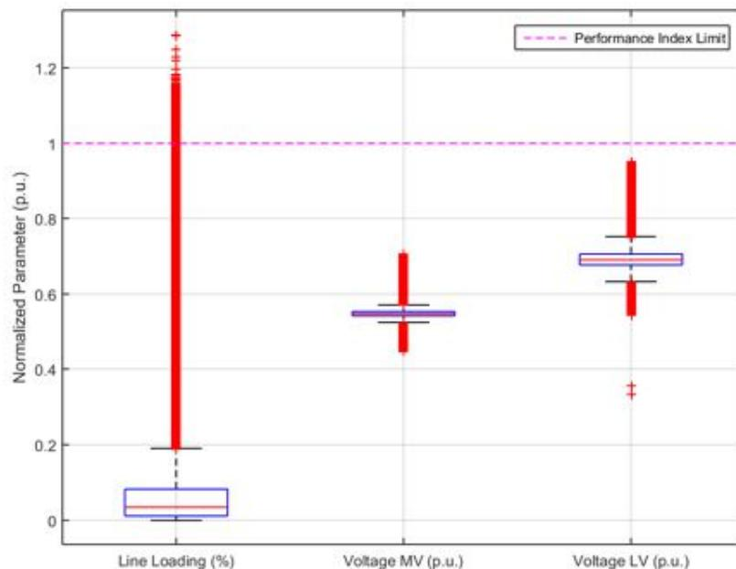
**Figure 173.** Performance Index parameters normalized to their limit – Unity Power Factor.
