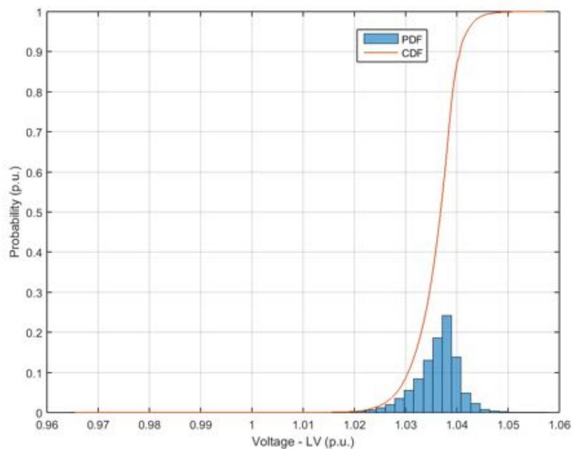
**Figure 184.** Probability distribution and cumulative probability distribution – Voltage at low voltage side – Power Factor  $\cos\phi(P)$ .
