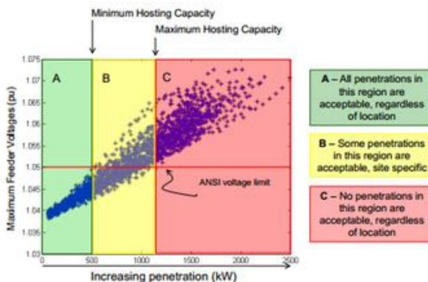
**Figure 10.** Graphical representation of PV hosting capacity zones [13].
