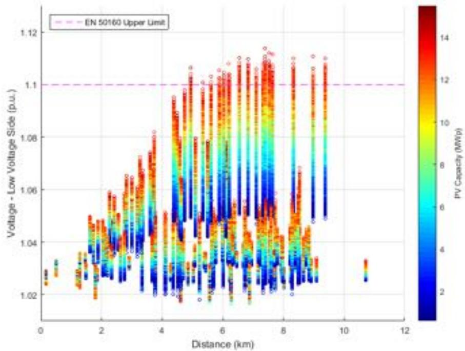
**Figure 115.** Voltage at low voltage side against distance from transmission substation - Power Factor  $\cos\phi(P)$ .
