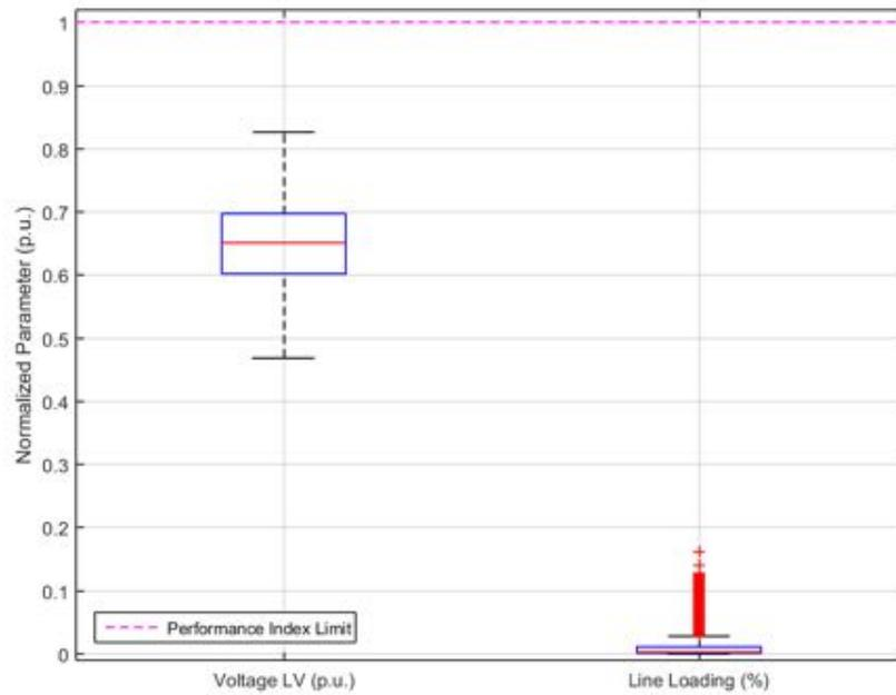
**Figure 136.** Performance Index parameters normalized to their limit – Unity Power Factor.
