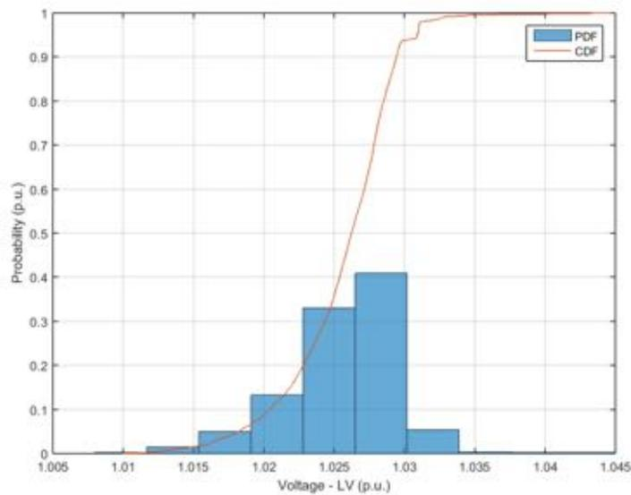
**Figure 35.** Probability distribution and cumulative probability distribution – Voltage at low voltage side – Power Factor equal to 0.95.
