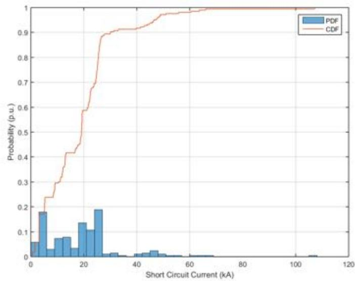
**Figure 41.** Probability distribution and cumulative probability distribution – Short Circuit Current – Power Factor  $\cos\phi(P)$ .
