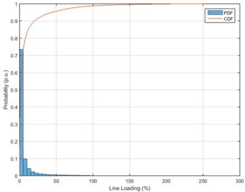
**Figure 292.** Probability distribution and cumulative probability distribution – Line Loading – Power Factor  $\cos\phi(P)$ .
