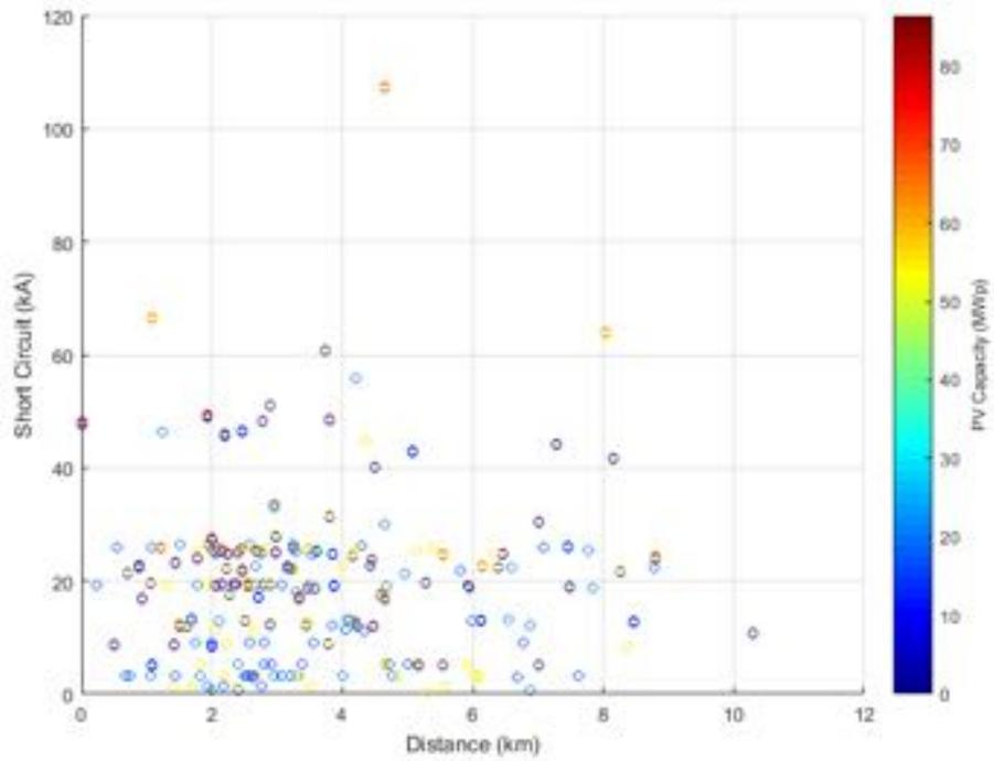
**Figure 64.** Short circuit current against distance - Power Factor  $\cos\phi(P)$ .
