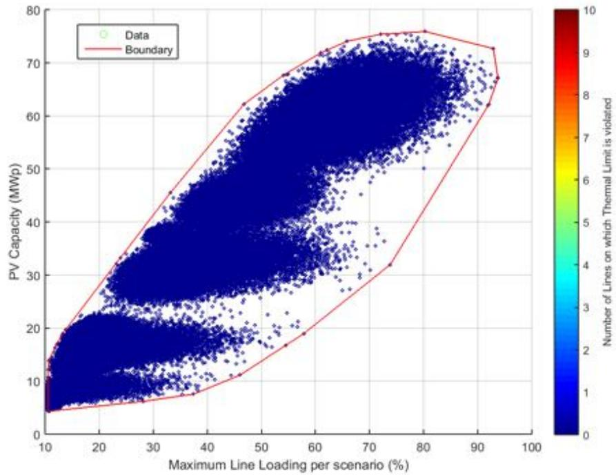
**Figure 211.** PV Capacity against Line Loading - Power Factor equal to 0.95.
