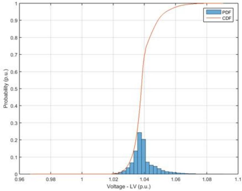
**Figure 174.** Probability distribution and cumulative probability distribution – Voltage at low voltage side – Unity power factor.
