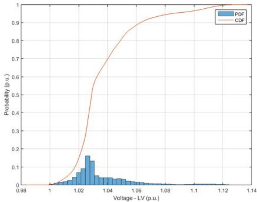
**Figure 78.** Probability distribution and cumulative probability distribution – Voltage at low voltage side – Power Factor  $\cos\phi(P)$ .
