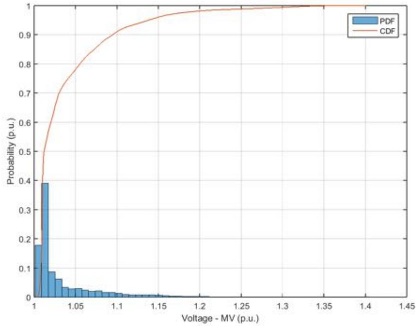
**Figure 233.** Probability distribution and cumulative probability distribution – Voltage at medium voltage side – Power Factor equal to 0.95.
