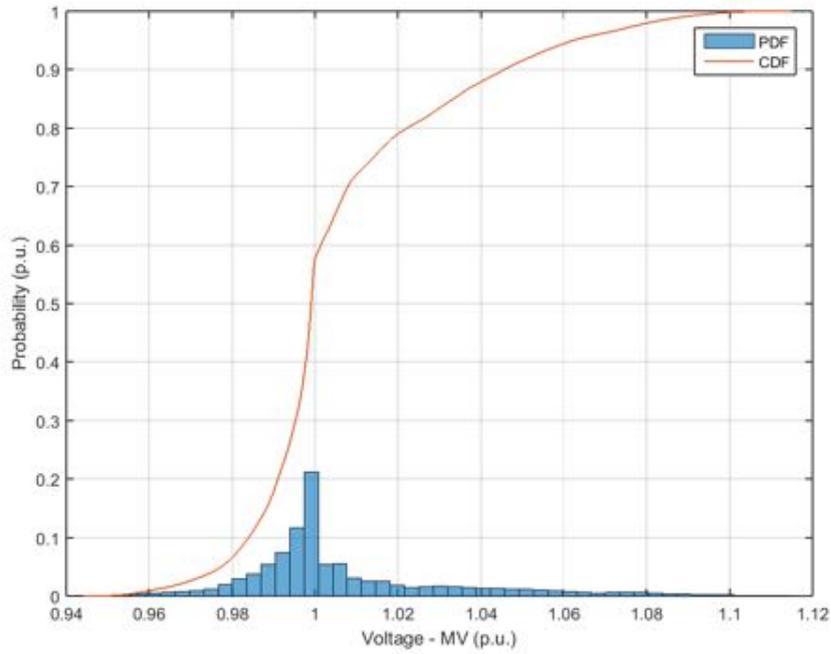
**Figure 291.** Probability distribution and cumulative probability distribution – Voltage at medium voltage side – Power Factor  $\cos\phi(P)$ .
