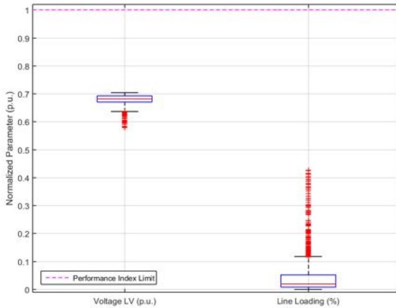
**Figure 193.** Performance Index parameters normalized to their limit – Power Factor equal to 0.95.
