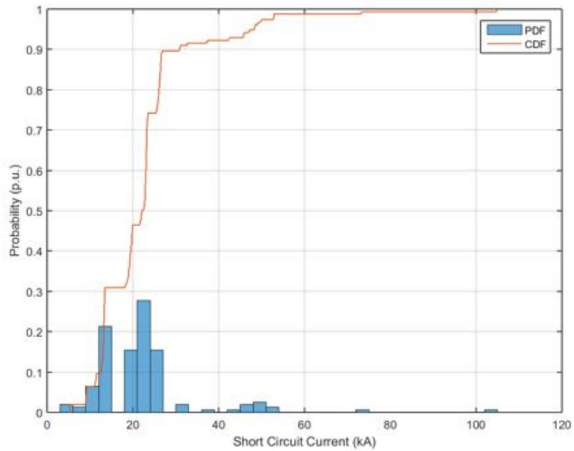
**Figure 188.** Probability distribution and cumulative probability distribution – Short Circuit Current – No PV.
