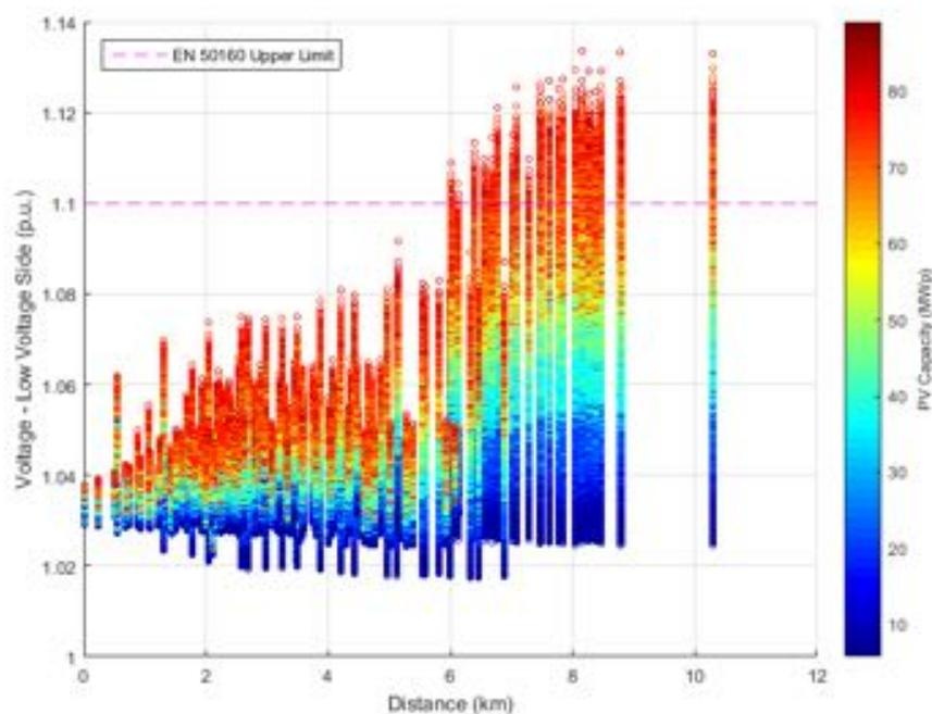
**Figure 46.** Voltage at low voltage side against distance from transmission substation - Unity Power Factor.
