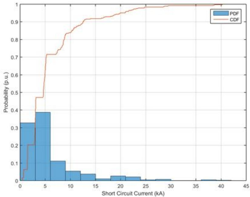
**Figure 302.** Probability distribution and cumulative probability distribution – Short Circuit Current – Power Factor equal to 0.95.
