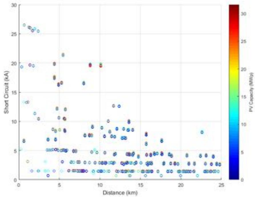
**Figure 170.** Short circuit current against distance - Power Factor  $\cos\phi(P)$ .
