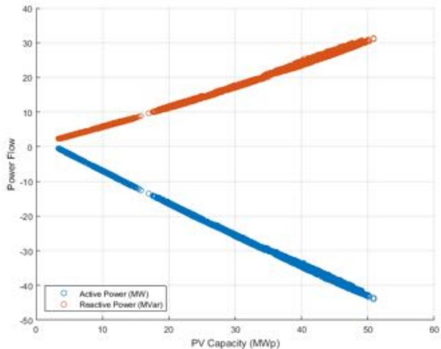
**Figure 328.** Power flow at PCC (connection of the reference substation with HV network) vs PV Capacity - Power Factor  $\cos\phi(P)$ .
