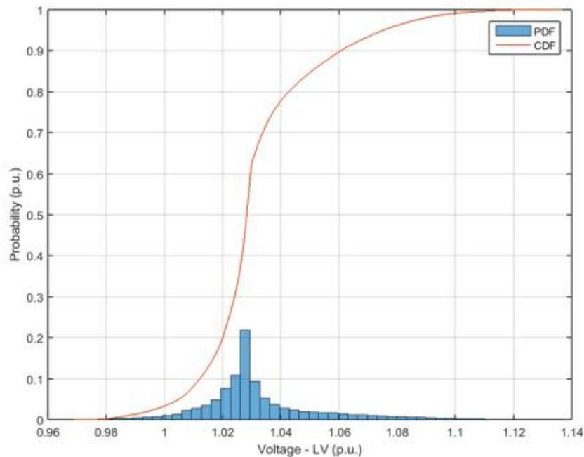
**Figure 285.** Probability distribution and cumulative probability distribution – Voltage at low voltage side – Power Factor equal to 0.95.
