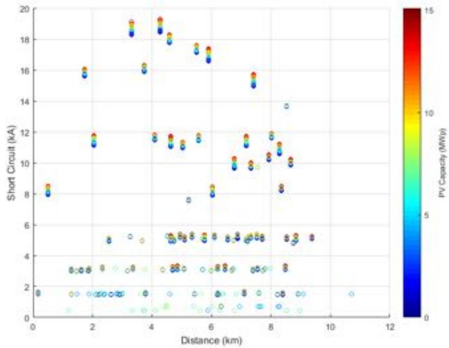
**Figure 101.** Short circuit current against distance - Unity Power Factor.
