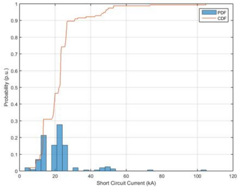
**Figure 187.** Probability distribution and cumulative probability distribution – Short Circuit Current – Power Factor  $\cos\phi(P)$ .
