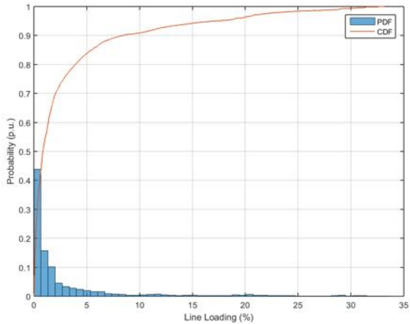
**Figure 89.** Probability distribution and cumulative probability distribution – Line Loading – Power Factor equal to 0.95.
