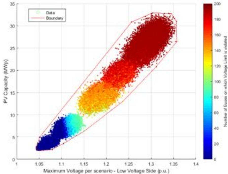
**Figure 148.** PV Capacity against Voltage – Low voltage side - Unity Power Factor.
