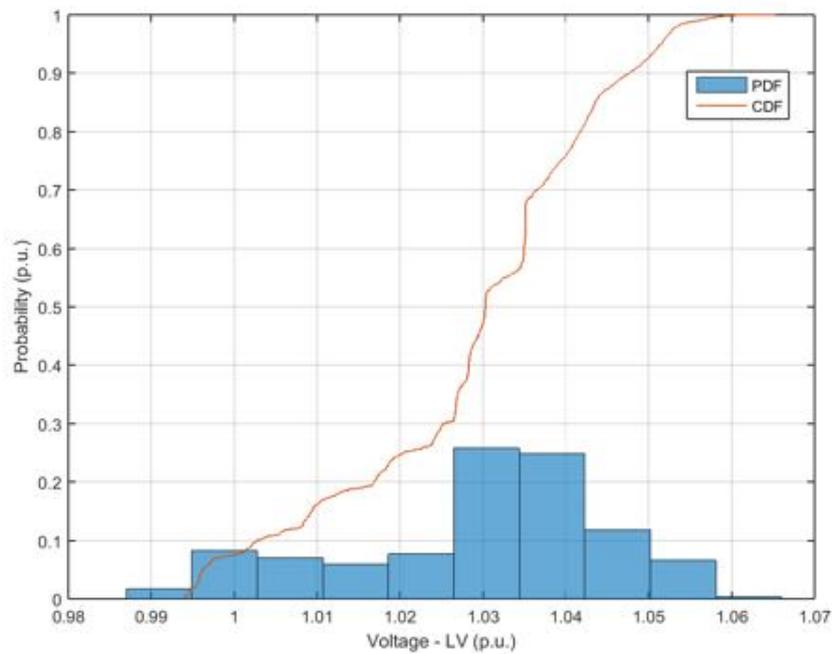
**Figure 137.** Probability distribution and cumulative probability distribution – Voltage at low voltage side – Unity Power Factor.
