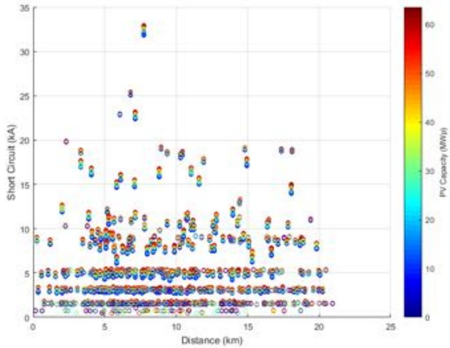
**Figure 260.** Short circuit current against distance - Unity Power Factor.
