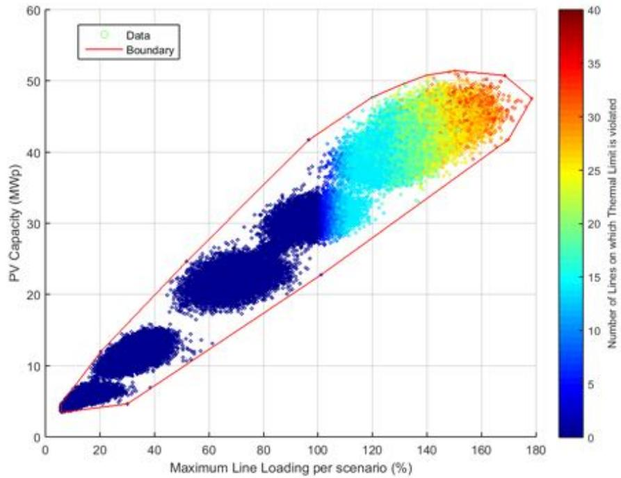
**Figure 309.** PV Capacity against Line Loading - Unity Power Factor.
