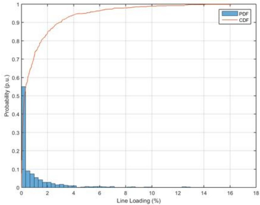
**Figure 142.** Probability distribution and cumulative probability distribution – Line Loading – Power Factor equal to 0.95.
