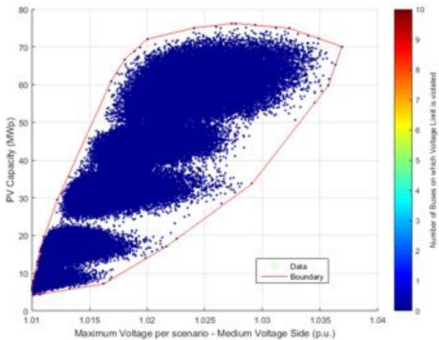
**Figure 202.** PV Capacity against Voltage – Medium voltage side - Unity Power Factor.
