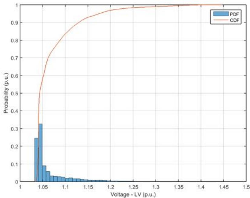
**Figure 232.** Probability distribution and cumulative probability distribution – Voltage at low voltage side – Power Factor equal to 0.95.
