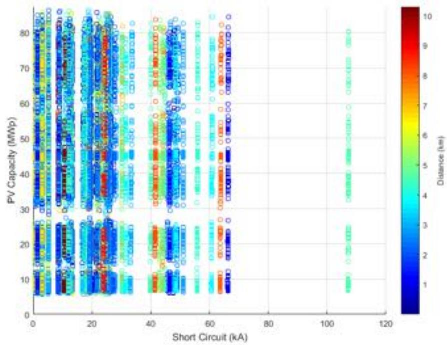
**Figure 57.** PV Capacity against Short Circuit current - Power Factor equal to 0.95.
