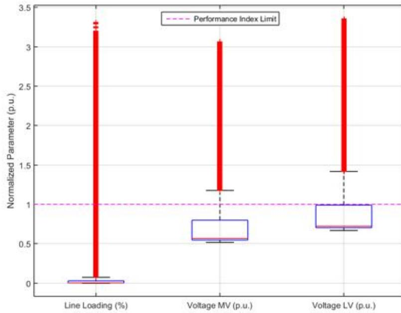
**Figure 226.** Performance Index parameters normalized to their limit – Unity Power Factor.
