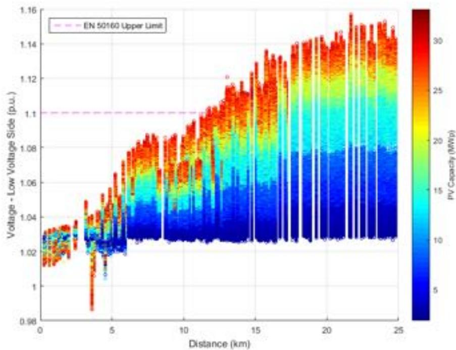
**Figure 168.** Voltage at low voltage side against distance from transmission substation - Power Factor  $\cos\phi(P)$ .
