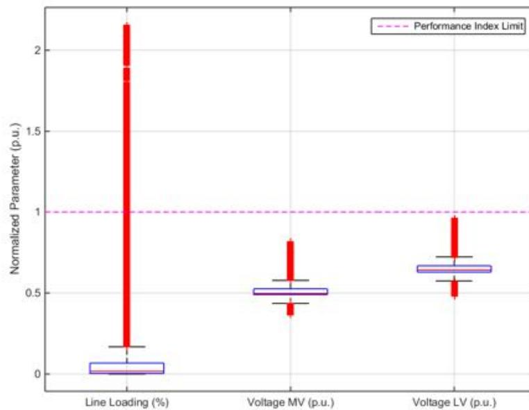
**Figure 24.** Performance Index parameters normalized to their limit – Power Factor  $\cos\phi(P)$ .
