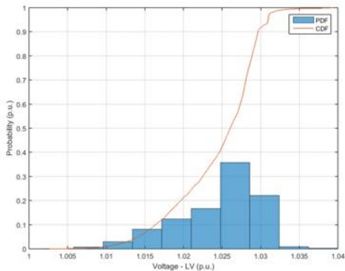
**Figure 39.** Probability distribution and cumulative probability distribution – Voltage at low voltage side – Power Factor  $\cos\phi(P)$ .
