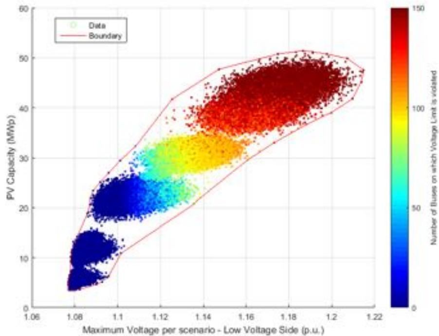
**Figure 307.** PV Capacity against Voltage – Low voltage side - Unity Power Factor.
