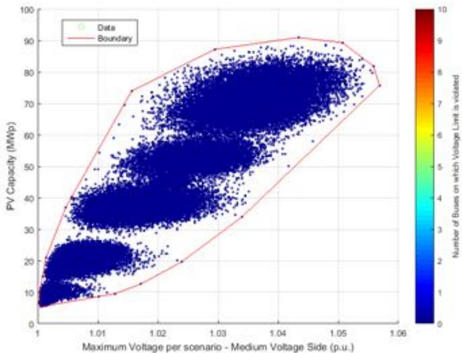
**Figure 51.** PV Capacity against Voltage – Medium voltage side - Power Factor equal to 0.95.
