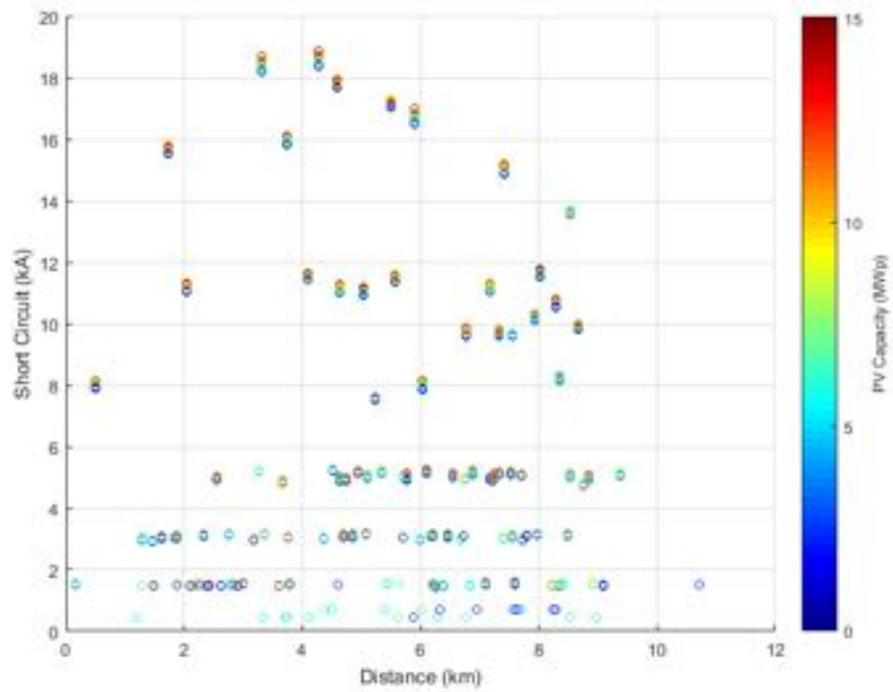
**Figure 117.** Short circuit current against distance - Power Factor  $\cos\phi(P)$ .
