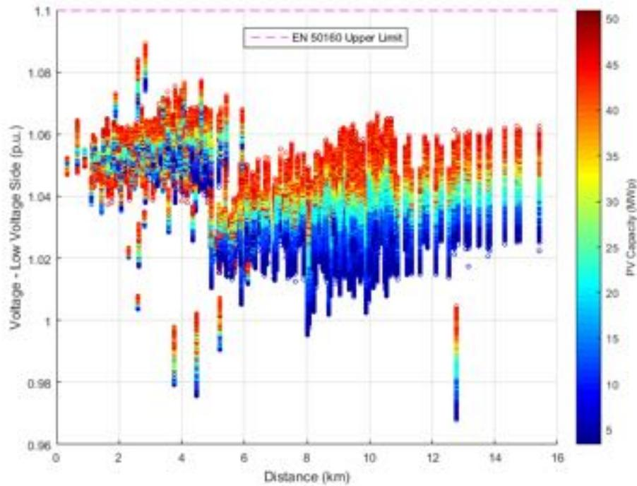
**Figure 327.** Voltage at low voltage side against distance from transmission substation - Power Factor  $\cos\phi(P)$ .
